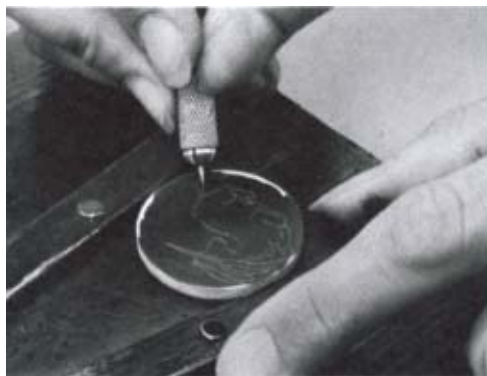
1. Blacken surface with indelible ink, then scratch very lightly to plan design.
