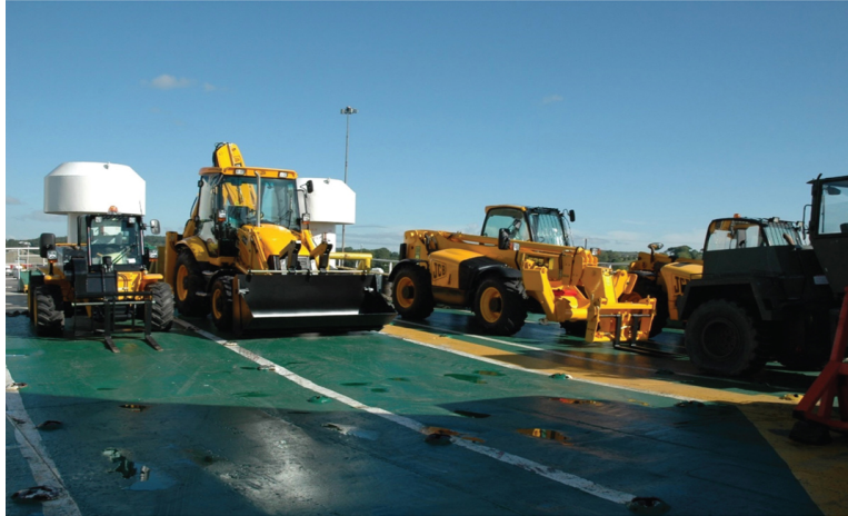
FIGURE 8.22 Possible heavy duty vehicles seen stowed on the upper weather deck of Ro-Ro vessel, prior to being fitted with chain lashings as per the Cargo Securing Manual ( CSM ). Farm tractors, digger vehicles etc, moving on tyres, are treated as runners. Tracked vehicles like military tanks or bulldozes are usually secured to a low-loader by chains and stowed as an integral unit.
