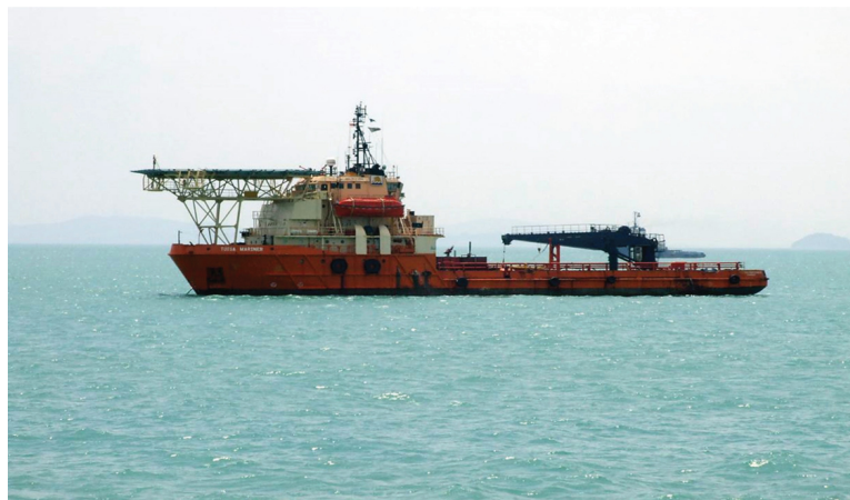
FIGURE 13.3 The ex- Toisa Mariner (IMO No. 7623916) renamed Excellent Diver , lies at anchor. Offshore support/supply vessel with heavy duty crane over the aft deck and prominent heli-pad. It is a multi-purpose offshore vessel capable of safety standby, offshore supply and diving support duties.
