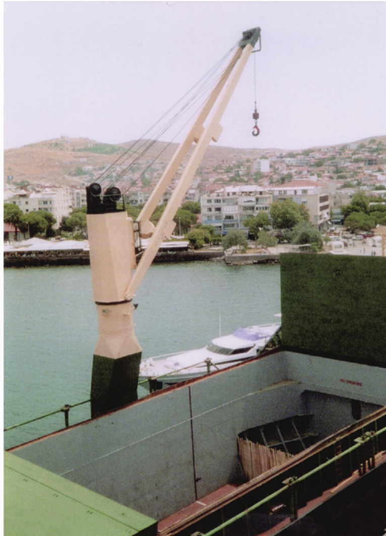
FIGURE 1.14 A 25 ton, SWL Shipboard pedestal crane sited on the port side aboard the general cargo vessel ‘Scandia Spirit’ (IMO No. 8817837) while moored alongside in ‘Dikili’, Turkey.
