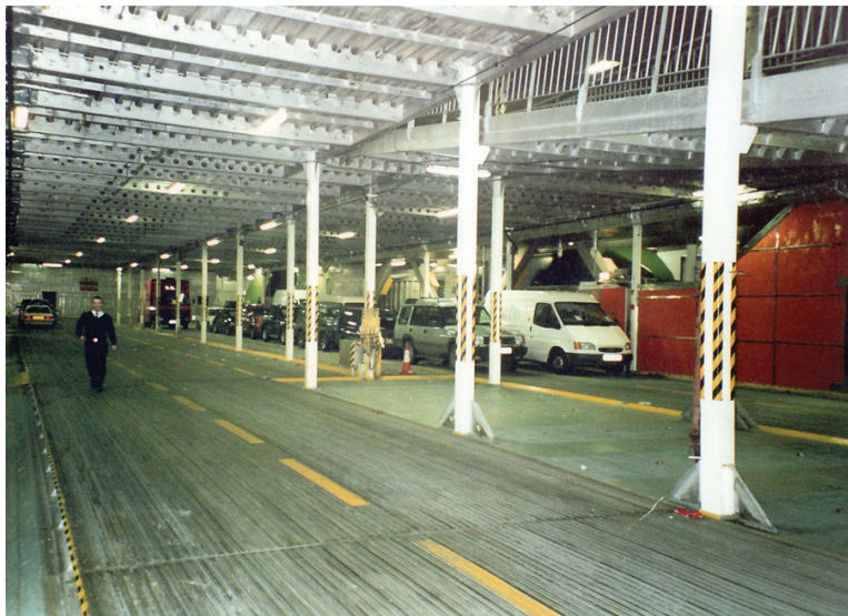
FIGURE 8.23 Roll on, Roll off vehicles being stowed on the internal cargo deck of a large vehicle ferry. Cargo officer monitors tight stowage in the ‘vehicle lanes’ seen walking past the inner ramp to the upper cargo deck.
