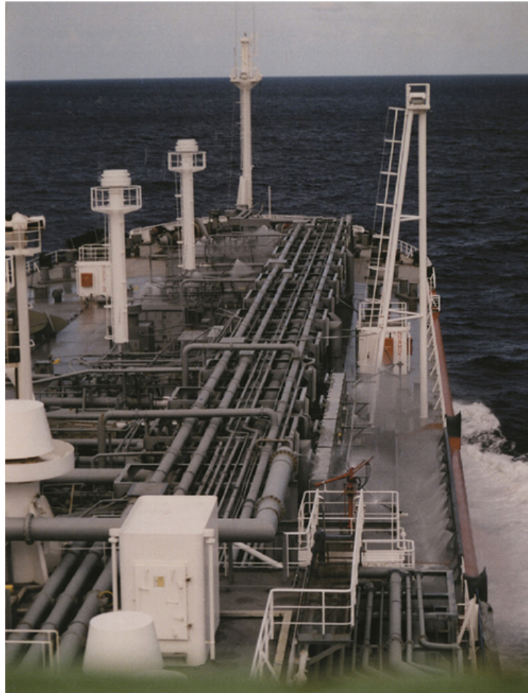
FIGURE 6.10 Typical example of the pipeline and ventilation arrangements (fore deck) of a medium-sized oil tanker seen in the seagoing environment.
