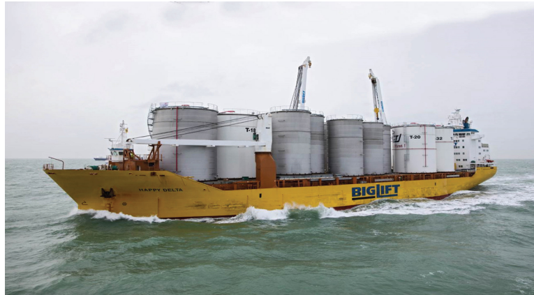
FIGURE 10.5 The Happy Delta (IMO No. 9551935) seen at sea transporting 13 stainless steel tanks on deck. The largest tanks were 14 metres in diameter at a height of 20.8 metres. The largest tank had a weight of 106 mt . The total volume of 40,000 cubic meters was the main issue as the total weight of the cargo was only 900 mt . Such a large exposed cargo attracts a greater windage which in turn could influence increased leeway when on passage.
