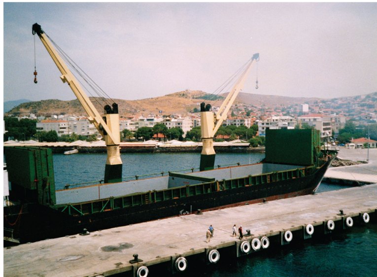
FIGURE 2.13 Open hatchway seen exposing the two cargo holds of the 'Scandi Spirit' (IMO No. 8817837) with the folding 'M' type hydraulic hatch covers in the fixed open position. The hatches are serviced by two port side pedestal cranes.
