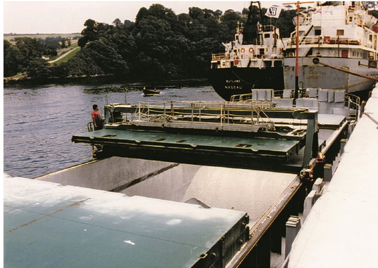
FIGURE 1.22 Stacked steel hatch covers aboard a modern coastal vessel. The ship is fitted with its own travelling mini-gantry crane, for the sole purpose of lifting on and off steel hatch covers.
