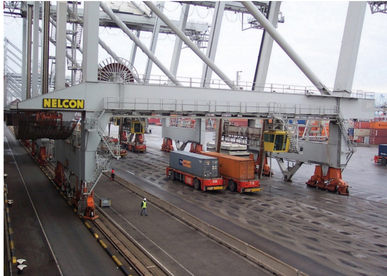
FIGURE 9.33 Tracked container gantry crane for the loading of containers. Semi-automated driverless transports deliver container units to its underside prior to loading onto the container vessel.
