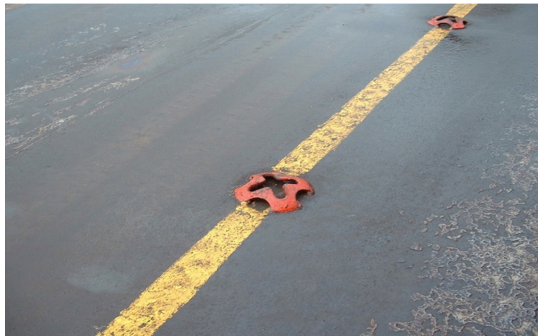
FIGURE 8.26 Deck star dome, raised or flush for the anchoring of chain lashings for Ro-Ro cargo units by hook or club foot attachment to the chain lashing end.
