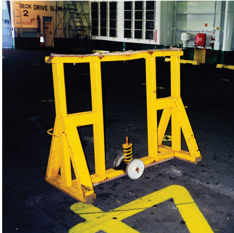
FIGURE 8.27 Wheeled trestle is positioned under the unit before being detached from the motor tug. Trestles are fitted with spring-loaded wheels to permit easy manoeuvring under the cargo unit.
