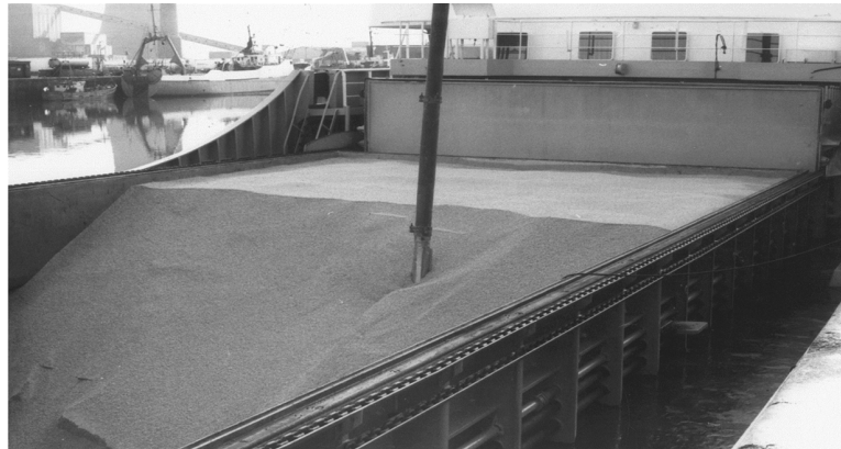
FIGURE 5.16 The suction is extended from the grain elevator into the cargo hold space to extract the cargo into the grain silo.
