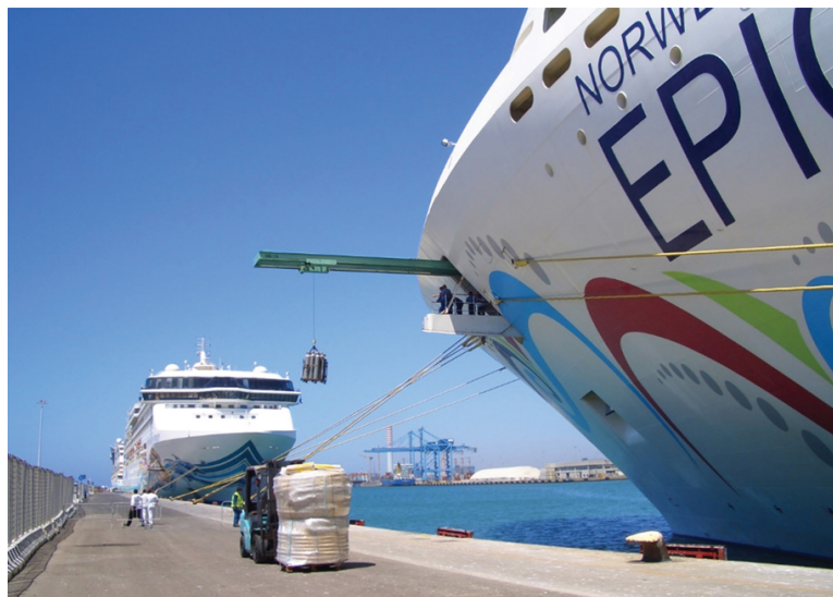
FIGURE 12.12 The passenger ship Norwegian Epic (IMO No. 9410569) seen loading stores and gas bottles into the forward stores by means of an electro-hydraulic gantry hoist.
