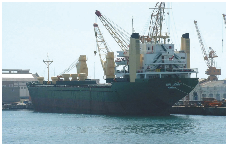
FIGURE 1.15 The Sir John (IMO No. 9634646) general purpose/container cargo vessel lies starboard side to in the Port of Barcelona, fitted with two heavy duty deck cranes both situated on the starboard side of the vessel. Seen with the number one crane in the stowed position and the number two pedestal crane topped and working with shoreside craneage.
