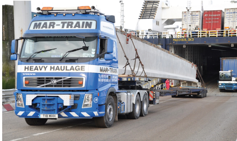
FIGURE 8.20 A long concrete load seen chained to a sixteen-wheel extending trailer after leaving the undercover hold of the ferry Clipper Point (IMO No. 9350666).
