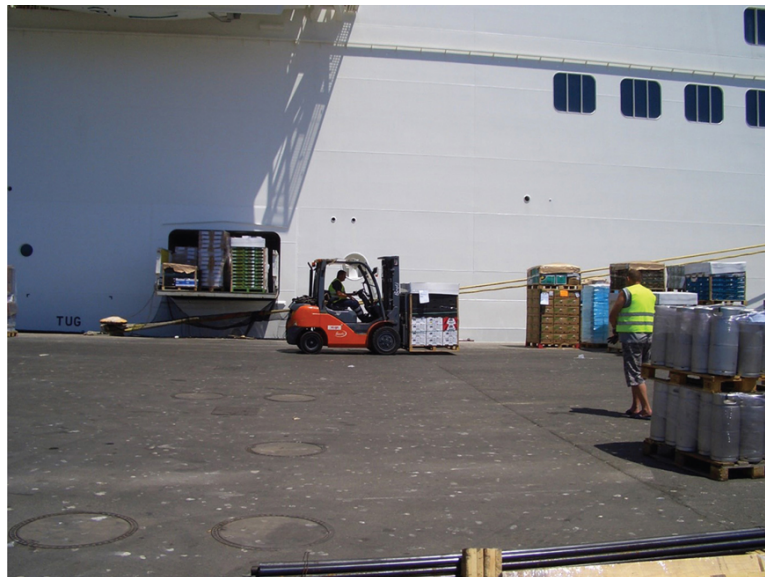
FIGURE 1.41 Small forklift truck used on the quayside for the movement of small cargo parcels, pallets and stores, seen loading into a passenger vessel via its shell door. Lift capacity varies with the size of the forklift unit.
