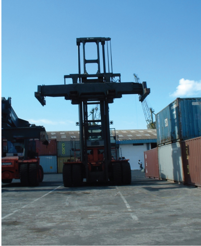
FIGURE 9.35 Container transporter with lift, transport, and stacking capability. A type of container karri lift based on the forklift truck principle which is widely employed in container terminals worldwide.
