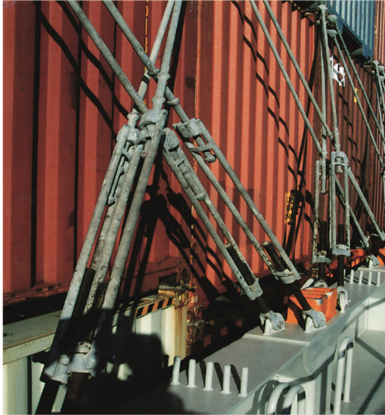
FIGURE 9.27 Stowed containers first and second tier of deck stow secured by lashing rods.
