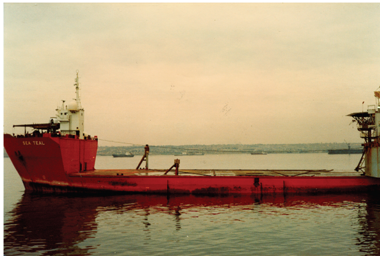
FIGURE 4.19 The 'Seal Teal' (IMO No. 8113566), showing the exposed steel cargo deck. The semi-submersible is seen without cargo and would submerge the deck to allow a float on cargo lift to take place.
