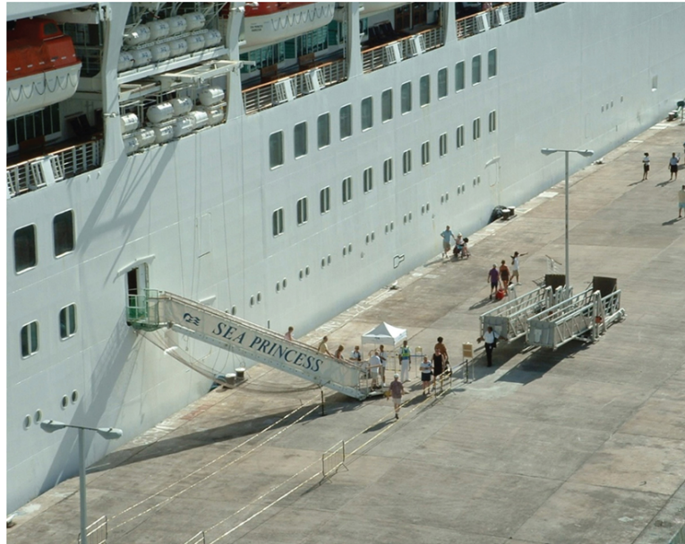
FIGURE 12.6 The passenger gangway arrangement from the Sea Princess (IMO No. 9150913) rigged from a side shell door to the quayside. Both inboard and outboard ends of the gangway are attended by security watchmen. A swipe on-board, swipe off-board system is usually in place so that the ship knows total persons on board at all times.
