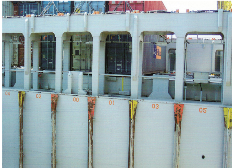
FIGURE 9.1 Empty ‘Cell guides’, numbered from the centre line, odd to starboard and even to port, found at the ends of the bays.
