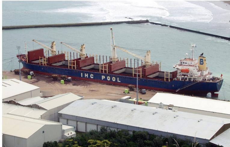
FIGURE 2.1 The Mount France general cargo vessel seen port side to on the timber berth in Napier, New Zealand. The vessel is loading ‘logs’ from quayside transports using its own deck cranes. The vessel has five hatches all fitted with hydraulic steel hatch covers, seen in the open position.
