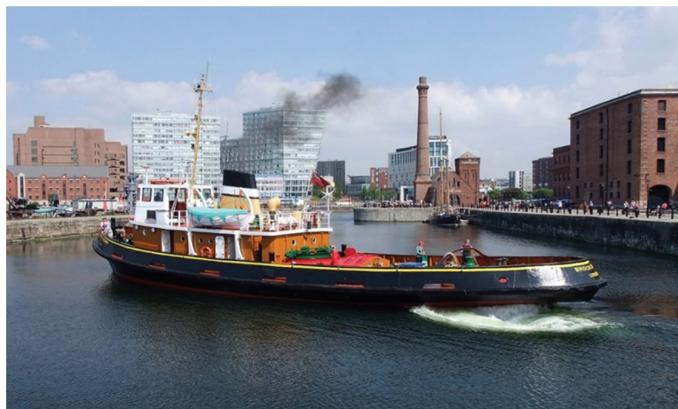
FIGURE 13.13 The Liverpool docking tug Brocklbank (IMO No. 642048) seen operating off Albert Dock Liverpool. The large cargo vessels, container, bulk carriers, tankers and passenger vessels generally all engage tugs for berthing.
