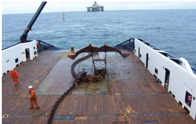
FIGURE 13.2 A 15 tonne 'Stevpris Anchor' being recovered to the aft open deck of an anchor handling vessel in the offshore regions of the North Sea.
