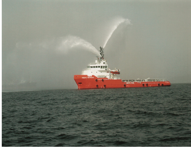
FIGURE 13.1 The new build Pacific Retriever (IMO No. 9236810, built 2002) anchor handling and offshore support vessel seen on trials testing and checking operational systems.
