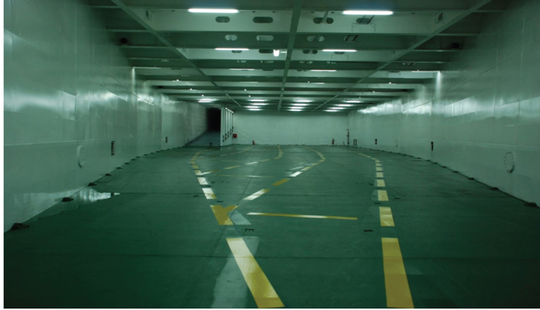
FIGURE 8.18 View inside the lower hold of the ferry Clipper Point . A lower ramp from the main vehicle deck is seen on the starboard side and the vehicle stowage lanes are indicated on the deck of the hold. Some Ro-Ro vessels do not have a fixed ramp into lower hold spaces and employ a built in hydraulic lift operation to load units below.
