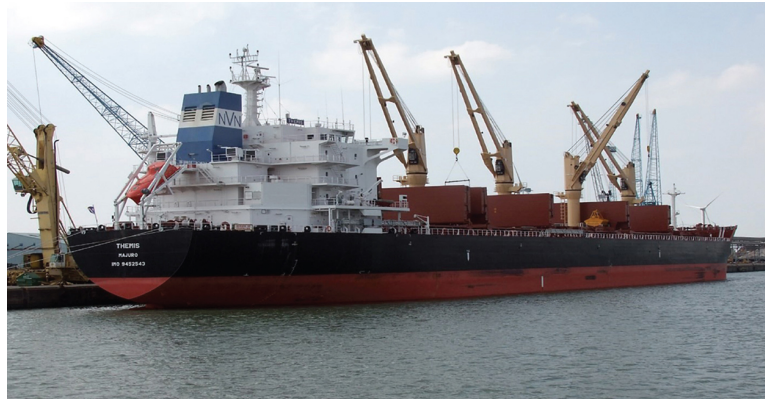
FIGURE 1.16 The general cargo bulk carrier 'Themis' seen with all deck cranes topped and working cargo from open steel hatches (IMO No. 9452543).
