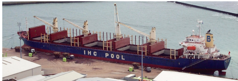
FIGURE 7.5 A vessel loads short timber logs from quayside trailers to cargo holds. The uprights are identified for the purpose of securing lashings for any timber deck cargo.
