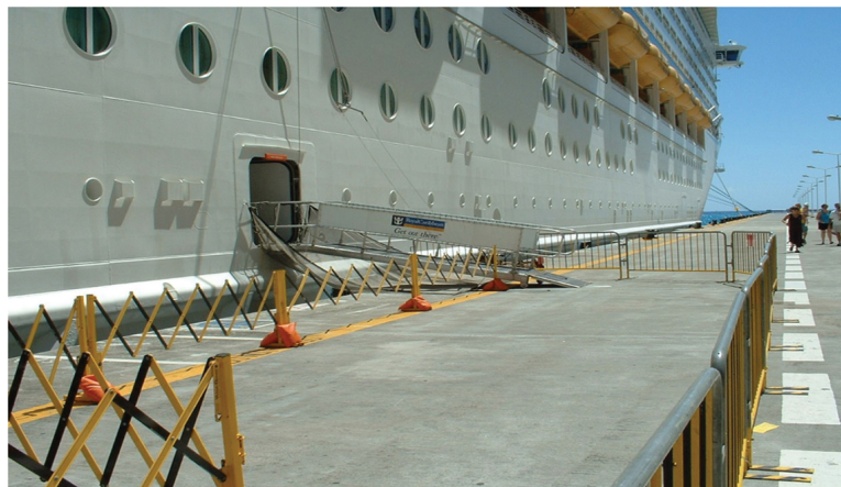
FIGURE 12.7 Gangway arrangements vary from ship to ship and port to port, usually because of changing tidal levels. The gangway shown is for the Royal Caribbean ship Explorer of the Seas (IMO No. 9161728) deployed with a security/safety fenced barrier area on the quayside.
