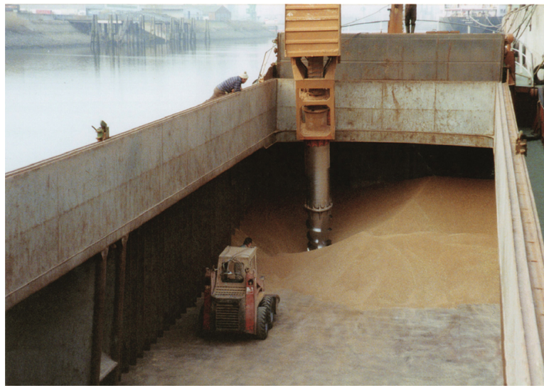
FIGURE 5.15 A tractor engaged in the tween deck of a vessel discharging cereals to ensure that suction of the grain elevator has access to all residuals of the cargo product.
