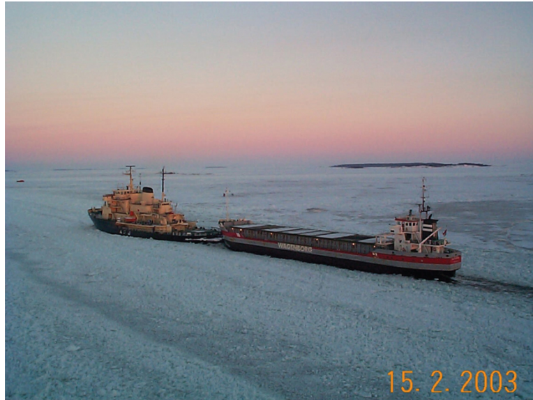
FIGURE 13.12 Designated ice-breaker engaged in towing a coastal vessel in Baltic ice conditions. Most of the countries around the Baltic Sea offer ice-breaker services to keep water access free to shipping.
