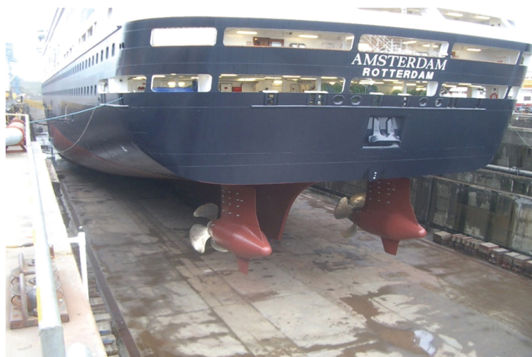
FIGURE 12.14 The passenger vessel Amsterdam (IMO No. 9853890) seen in dry dock fitted with twin 'pod' propulsion units either side of a centre line skeg. A centre line stern anchor is also featured. Such ships are usually built with a high level of manoeuvring aids like stabilisers, bow thrust units and CPP propellers. The Master/pilot will tend to have 'joystick' fingertip bridge control of all ship movements, particularly useful to ensure ease of docking and berthing activities.
