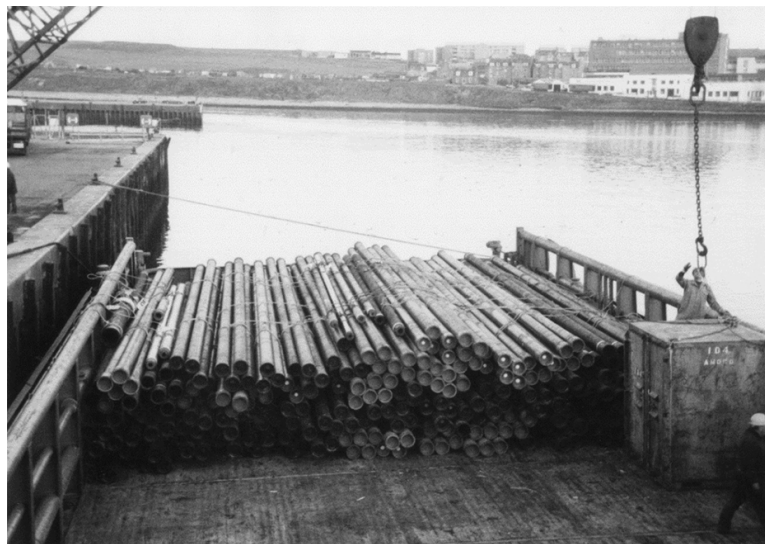
FIGURE 10.9 Capped drilling pipes seen loaded on the wide beam cargo deck of an offshore supply vessel. The pipes are capped at each end to prevent water retention in the event of the vessel encountering rough weather. Any fluid in quantity being retained among deck cargoes could seriously affect the positive stability of the vessel.
