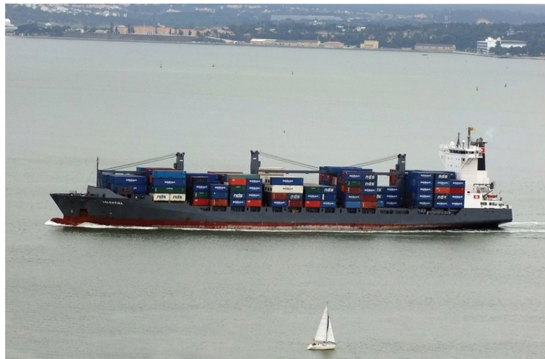
FIGURE 9.8 The container vessel Valentina (IMO No. 9344722) seen loaded in a seagoing condition. The ship is equipped with its own container cranes.
