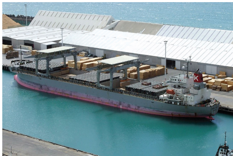
FIGURE 1.23 The 'Pan Pac Spirit' (IMO No. 9186780) seen starboard side to the timber berth in Napier, New Zealand. The ship engages in loading finished package timber by means of her own ships gantry cranes.
