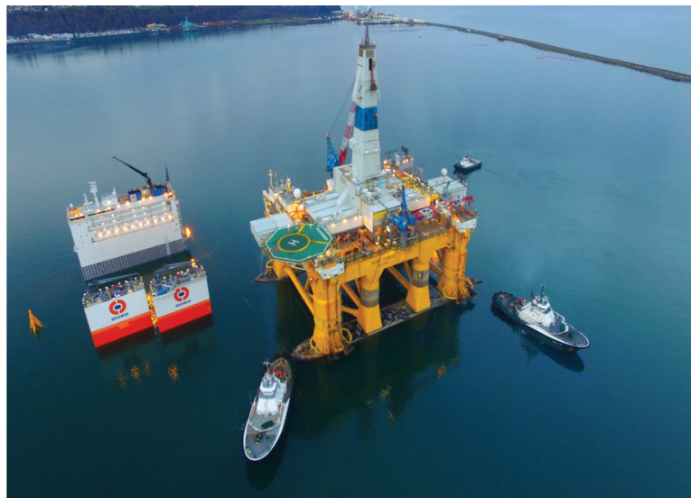
FIGURE 4.29 The offshore installation Polar Pioneer is seen being manoeuvred with tug assistance over the submerged platform deck of the semi-submersible Dockwise Vanguard .
