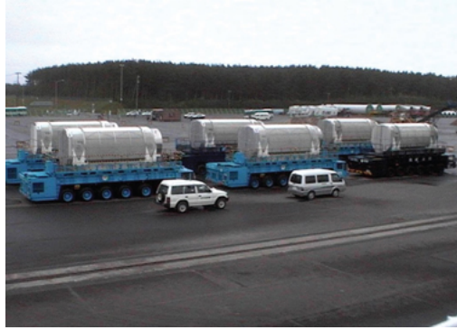
FIGURE 11.1 Nuclear waste flasks discharged with full heavy lift precautions onto special transports in Japan monitored by security mobiles and specialised personnel. Open aspects and security fencing surround the working area of the port facility.
