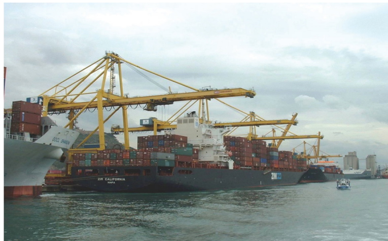
FIGURE 9.2 Gantry cranes engage in container cargo operations over the Zim California (IMO No. 7043556) berthed in Barcelona, Spain.
