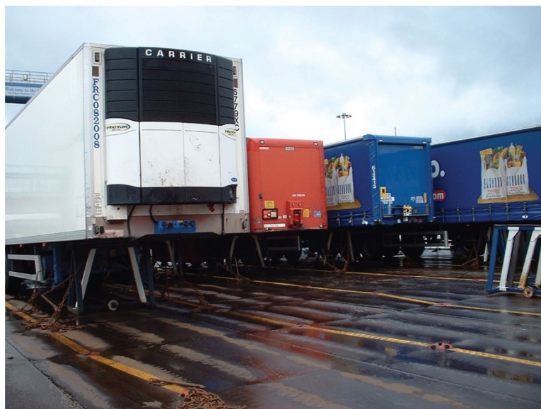
FIGURE 8.14 Example upper vehicle deck of the Ben-My-Cree RoPax ferry operating in the Irish Sea region. Drop trailer units are seen stowed on trestles in vehicle lanes. Load binder chain lashings are seen securing the units to star dome lashing points.
