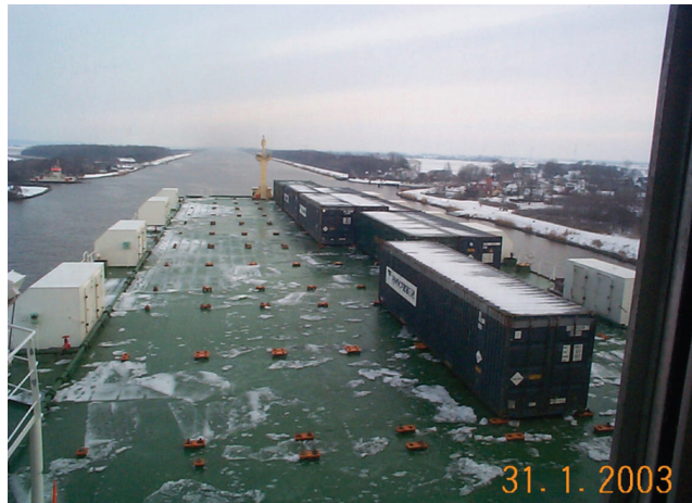
FIGURE 10.6 The steel fore deck of the Baltic Eide (IMO No. 8801917) fitted to receive containers overall, but seen above with a part load of containers, as its deck cargo, during a transit of the Kiel Canal.
