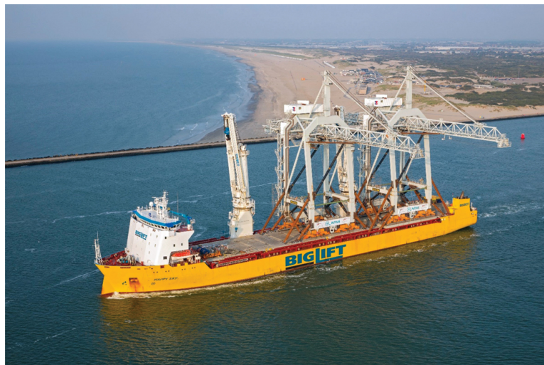
FIGURE 4.31 The ‘Happy Sky’ (IMO No. 9457220) of the Big Lift shipping company engaged in transporting two container gantry cranes secured to its upper deck. With such a high load, the centre of gravity of the cargo above the ship’s centre of gravity, effective lower ballast was used to maintain the ships stability. Obvious concerns for the passage plan for such a cargo would also be for the air draught through narrow waterways and if passing under low bridges.
