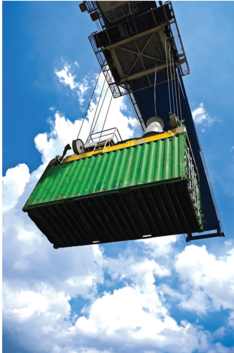
FIGURE 9.4 Extended jib of a ship loading gantry crane seen engaged in container movement, ship to shore.
