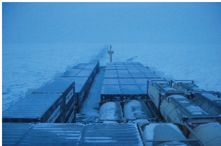
FIGURE 9.23 The foredeck of the Baltic Eider loaded with a container deck cargo. The stow includes single and double tier standard containers inclusive of liquid tank containers seen aft and to starboard. The vessel is seen passing through a pancake ice sea surface in the Baltic Sea.
