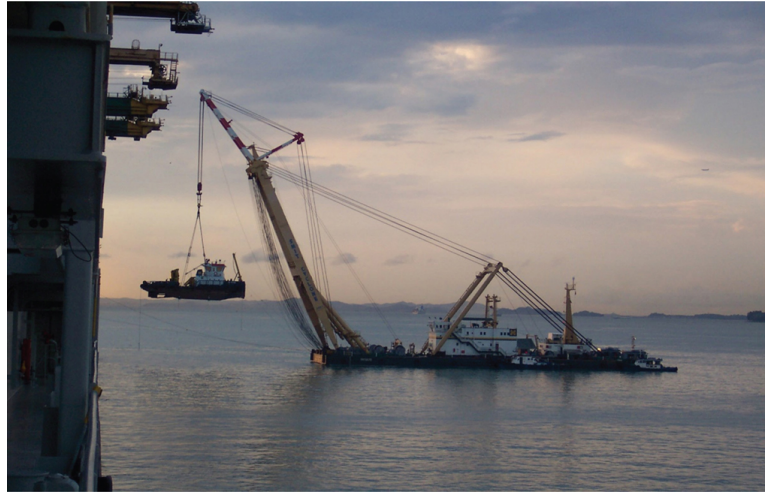
FIGURE 4.17 The Smit ‘Cyclone’ (IMO No. 7603688) floating sheer leg barge, engages in a general cargo heavy lift operation on a container vessels offshore side.
