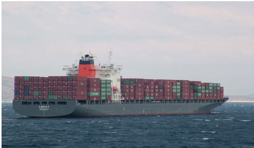
FIGURE 11.8 The container ship Lircay (IMO No. 9294824) seen with deck container stack fore and aft of the navigation bridge position. The tiers of the containers are five (5) high above the weather deck. The larger container vessels of today frequently have up to ten or eleven tiers high. The Lircay has been renamed Pohorje .
