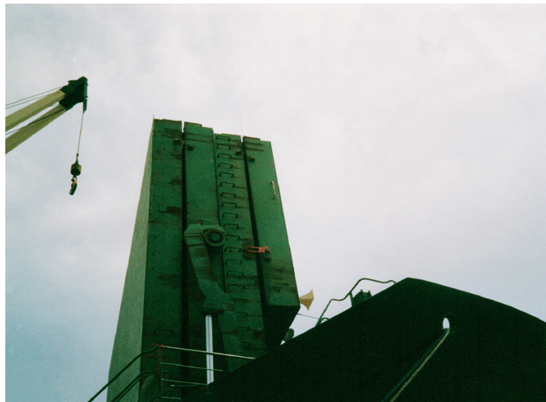
FIGURE 2.8 Folding hydraulic operated double steel hatch covers, seen in the vertical open position. Securing cleating seen in position prevents accidental roll back when in open position.
