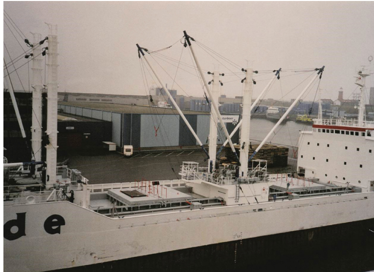
FIGURE 1.4 General cargo vessel rigged with conventional 5 tonne SWL derricks and steel hatch covers. The derricks can be rigged to operate as single swinging derricks or rigged in ‘Union purchase’ with schooner guys secured between the derrick heads.
