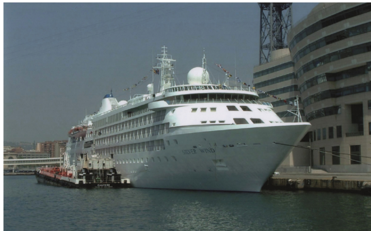
FIGURE 12.11 The passenger vessel Silver Wind (IMO No. 8903935) seen port side to alongside the passenger terminal in Barcelona, Spain while taking bunkers from an oil barge on the starboard side.
