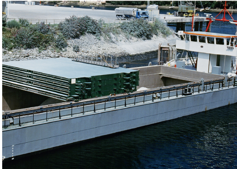
FIGURE 2.9 Steel hatch pontoon type covers seen stacked on the part open hatch. The covers are lifted and stacked by the ship's own mini-gantry travelling crane.
