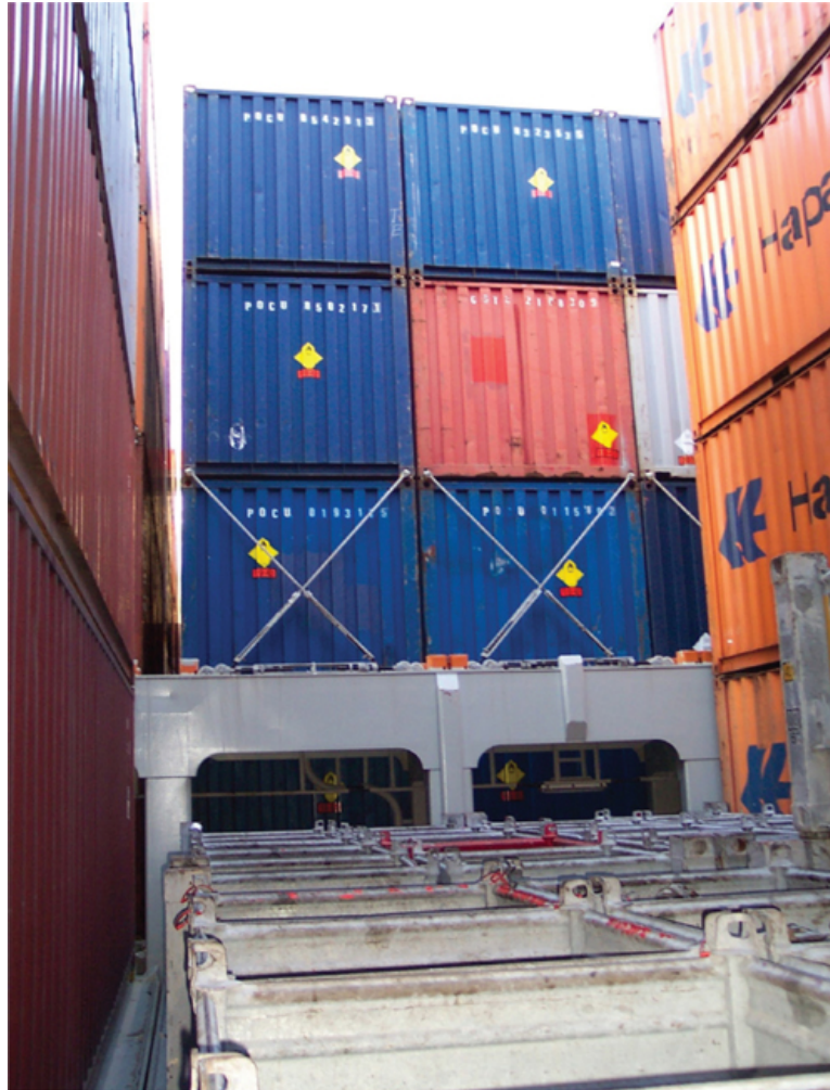
FIGURE 9.26 The deck stow is seen in way of the edge of the pontoon hatch cover. The lashings are to the base, third tier container level by long bar. The second tier container level being secured by short bar lashings with the base containers locked to the pontoon.
