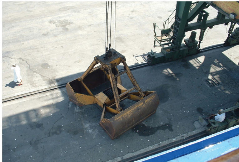
FIGURE 5.10 Mechanical clamshell bucket grab seen in the open position on the quayside. The crane is configured so that the controlling crane driver can open and shut the grab by means of a control wire to open and close the bucket arrangement.
