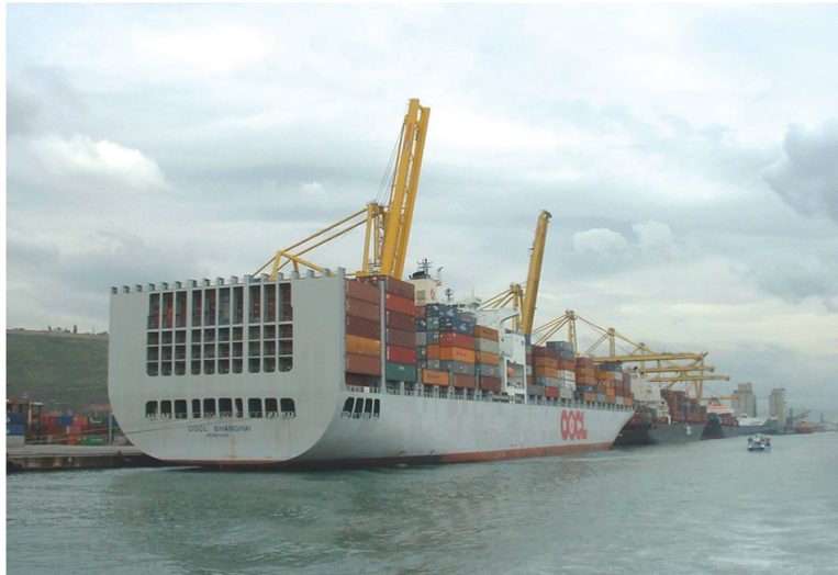
FIGURE 9.18 The OOCL Shanghai (IMO No. 9198111) lies port side to the container terminal in Barcelona, Spain, after completing cargo loading with a full container load. The deck stack is at a six tier height. The terminal gantry cranes are seen in the upright and clear position. (The ship is not fitted with its own cranes.)
