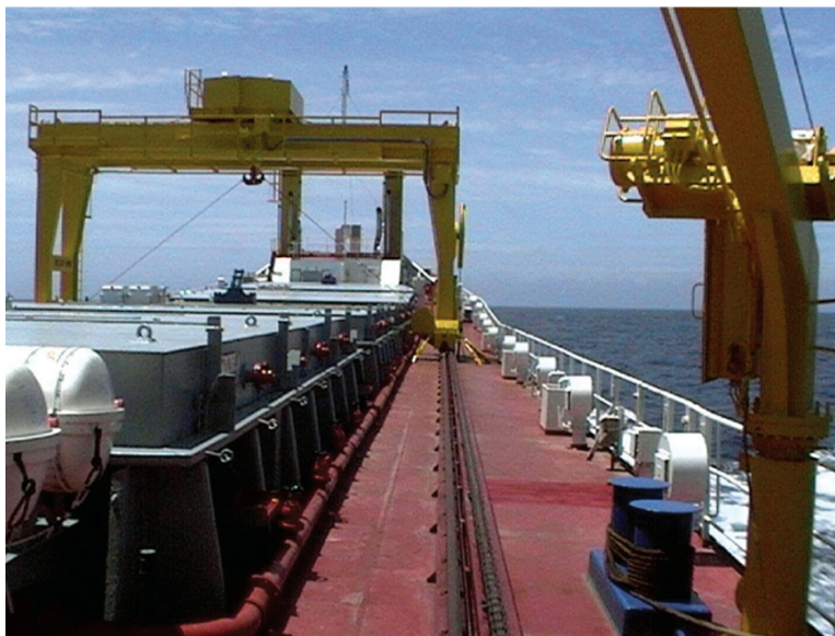
FIGURE 1.21 Shipboard tracked travelling gantry crane fitted to the fore deck of vessel dedicated to the carriage and transport of nuclear waste material.
