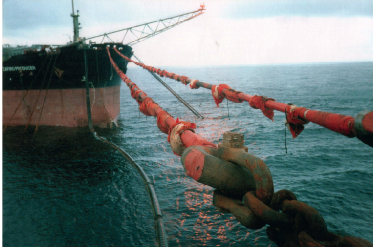
FIGURE 6.2 Tanker moorings and floating pipeline seen prior to liquid cargo transfer taking place from the Floating Storage Unit (FSU) to the tanker.
