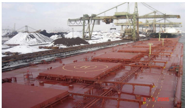
FIGURE 5.8 The bulk carrier Berge Nord (IMO No. 9127150) alongside the iron ore berth Seven Islands, Canada. The upper deck shows the side moving hatch top arrangement in the closed positions.
