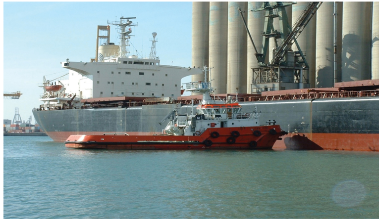
FIGURE 5.19 The bulk carrier Konkar Lydia (IMO No. 8022444) seen here twin side opening hatch tops open lying port side to the grain silo berth in Barcelona, Spain. The tug in attendance provides size comparison of the hatch top covers.
