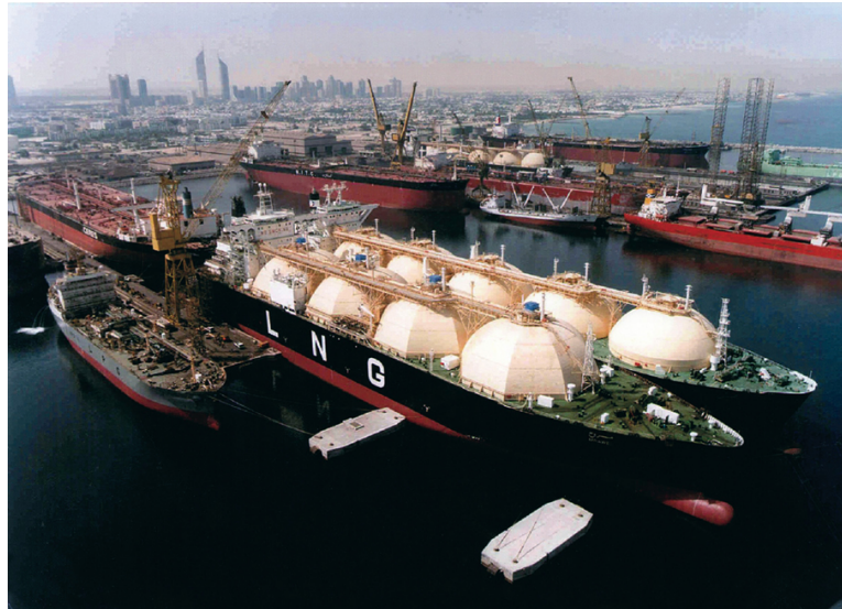
FIGURE 6.32 Two liquid natural gas carriers lay alongside each other, outside the Dubai dry dock complex. These dedicated ships are prominent for the conspicuous cargo domes covering the gas tanks.
