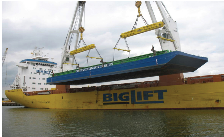
FIGURE 4.23 Big Lift vessel ‘Happy Delta’ (IMO No. 9551935) engages in a tandem lift, employing its two heavy duty Huisman cranes to discharge a long steel barge (cargo) into a calm water landing. Heavy duty lift beams work with four bridle spreaders to accept the load along its full length.
