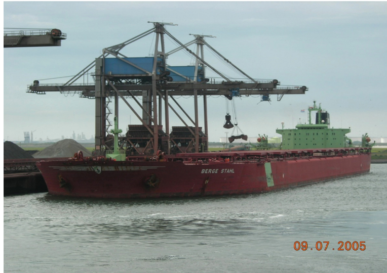
FIGURE 5.7 The bulk carrier Berge Stahl (IMO No. 8420804) is seen starboard side to the loading berth. The shoreside gantry cranes use 20-tonne mechanical grabs to complete the loading of iron ore.
