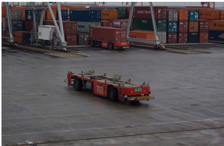
FIGURE 9.32 Automated driverless ground handling transports deliver container units from the terminal stack to the underside of ship/shore gantry cranes.
