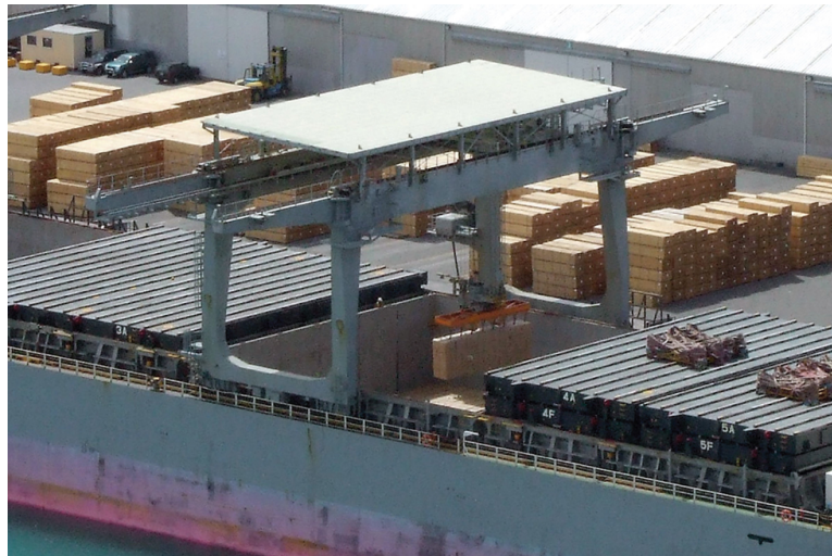
FIGURE 7.6 Tracked gantry crane loading packaged sawn timber, below decks in Napier, New Zealand. The outraches of the gantry crane are seen extended to allow the hoist carriage to load stacked quayside loads to the cargo holds.
