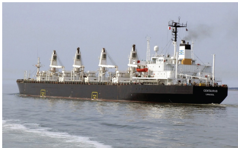
FIGURE 1.17 The cargo vessel 'Centaurus' seen in a seagoing capacity departing the River Mersey, all cranes lowered and secured and hatches battened down (IMO No. 8118592).
