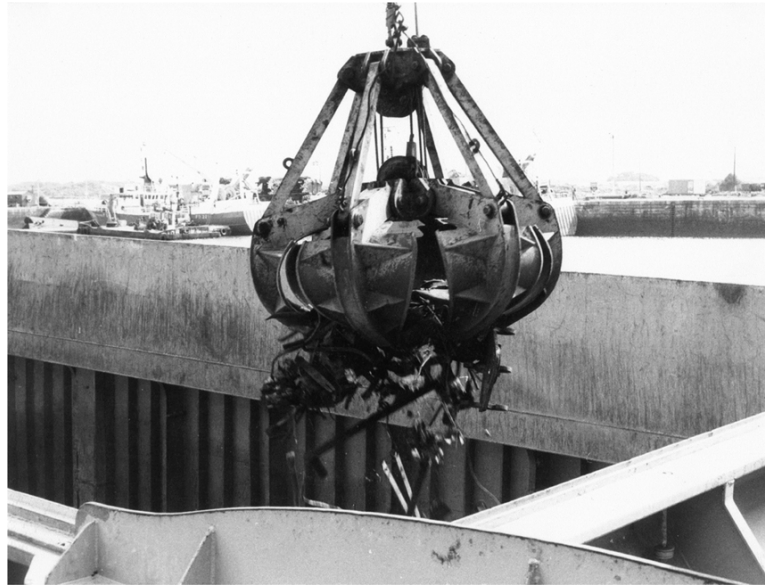
FIGURE 5.9 A mechanical grab with the tines closed, seen discharging scrap metal.
