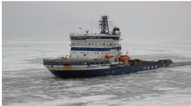
FIGURE 13.5 The Nordica offshore support vessel seen in operations in ice conditions of the Baltic Sea in 2003. Built as a multi-purpose ice-breaker and platform supply vessel. Also capable of being employed in offshore construction duties.
