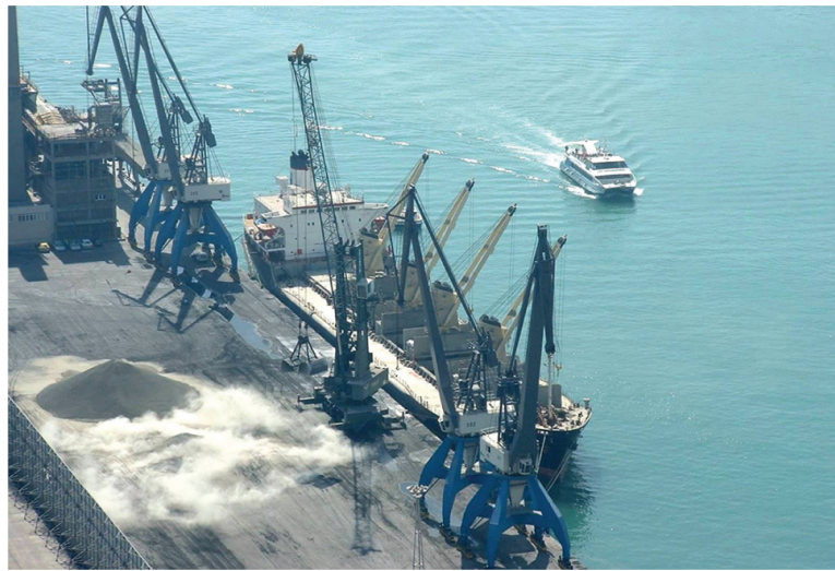
FIGURE 5.2 An overhead view of a general cargo vessel engaged in the discharge of concentrates by means of a free-standing crane using a mechanical grab. The ship's own deck cranes are turned outboard to allow easy access for the shoreside crane operation.
