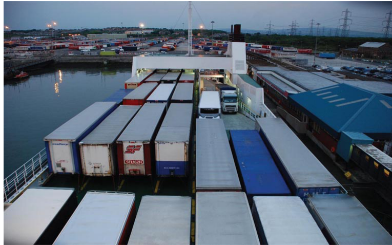
FIGURE 8.17 The same vehicle deck of the ferry Clipper Point (IMO No. 9350666) fully loaded with drop trailers and runner units on the ramp on the port side.
