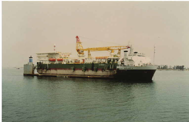
FIGURE 4.20 The heavy lift vessel ‘Super Servant 3’ (IMO No. 8025331) loaded by float on float off methods with the crane barge Al-Baraka 7 , seen lying at anchor in the Arabian Gulf region.
