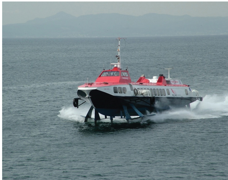
FIGURE 12.17 High-speed hydrofoil passenger-only Flying Dolphin 17 (IMO No. 8331467) operational in the non-displacement mode in the Mediterranean Sea in the vicinity of the Greek Islands.
