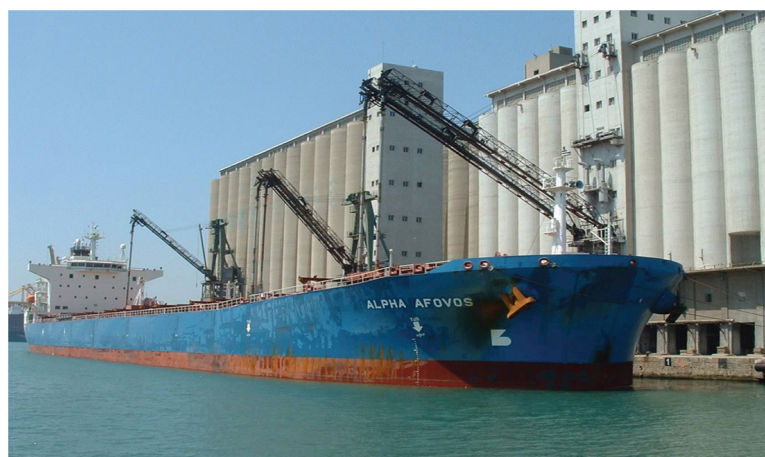
FIGURE 5.14 Bulk carrier Alpha Afovos (IMO No. 9221853) lies port side to the grain silos in Barcelona. The grain elevators are seen
