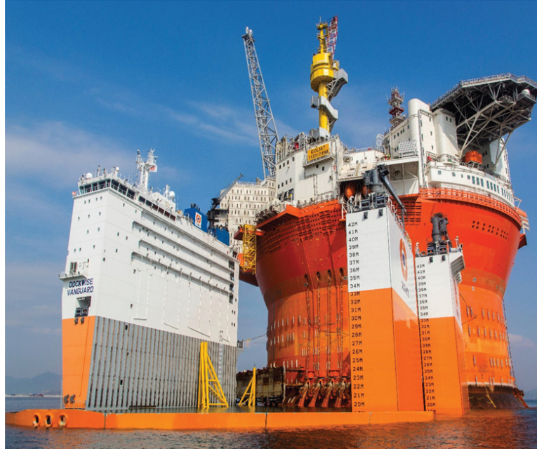
FIGURE 4.25 The Dockwise Vanguard (IMO No. 9618783) seen in a semi-submersible position lifting the Goliat (FPSO), a turret loading system, for delivery to an offshore site. Such project loads are frequently of several thousand tonnes per transport. The vessel has since been renamed as ‘Boka Vanguard’. It has a lift capacity of 110,000 tonnes.
