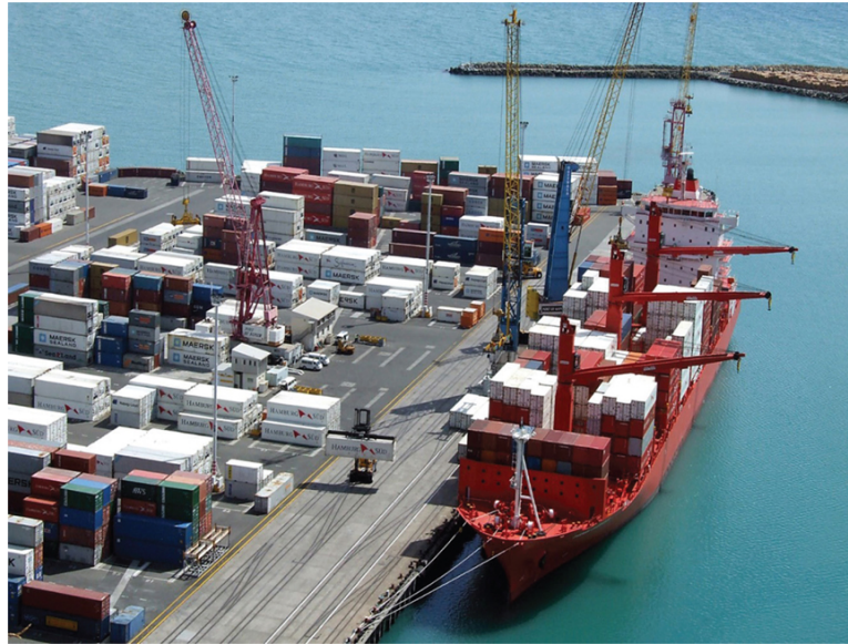
FIGURE 1.19 The ‘Tasman Crusader’ (IMO No. 9344667) renamed ( Cap Patton ) seen fitted with its own deck container cranes working containers by shore side cranes while starboard side to, in Napier, New Zealand. The ships own deck cranes are turned outboard to allow working space for cargo movement.
