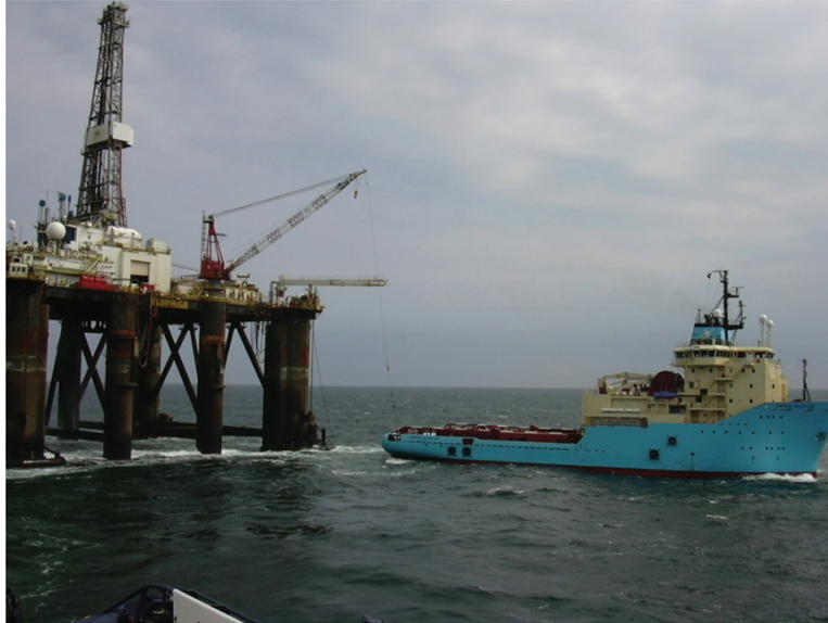
FIGURE 13.9 An AHV Maersk Achiever (IMO No. 9245902) in close proximity to the installation prior to using the chaser method to recover an anchor.
