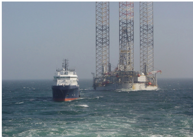
FIGURE 10.11 A jack-up oil drilling rig 'Galaxy III' is moved under tow by the anchor handling vessel (AHV) Highland Courage .
