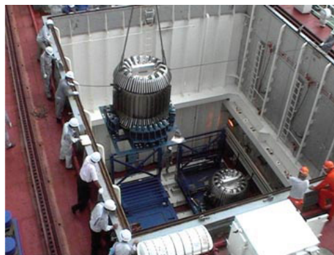
FIGURE 11.3 Nuclear waste flasks being lifted from carriage cradles from a stowed position inside a lower hold. The units are bolted onto the athwartships beams of the ship and treated as heavy lift, supervised loads. Once landed to the transports on the quay, the bedplates of the units are bolted onto the ground transports to become an integral unit, preventing any unwanted movement of the flask.
