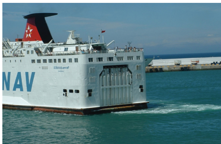
FIGURE 8.8 Example stern door of a RoPax ferry Al Masour (IMO No. 7360629) seen in the stowed, closed position as she turns off the berth in the harbour of Tangier.
