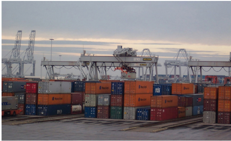
FIGURE 9.31 Automated stacking cranes provide unit movements to the terminal's container stack. The containers are being loaded to driverless ground handling transports.
