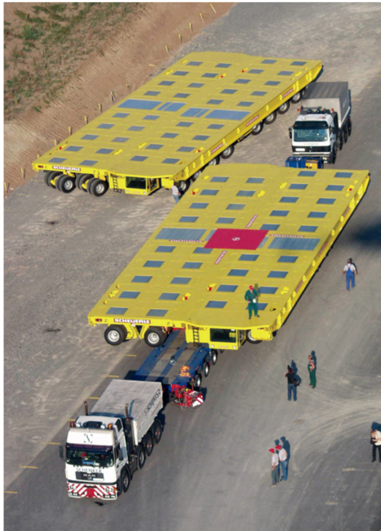
FIGURE 4.27 Scheuerle multi-wheel land driven heavy lifting transport platforms. These combination platforms can be adapted in size to suit smaller and larger loads at shippers needs. They are extensively used to transport heavy lift parcels and project cargoes.
