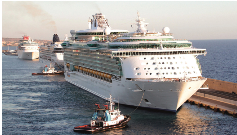
FIGURE 12.13 Large Class 1A passenger vessel Liberty of the Seas (IMO No. 9330030) operated by Royal Caribbean Shipping Company, seen berthing with tug assistance at fore and after ends.
