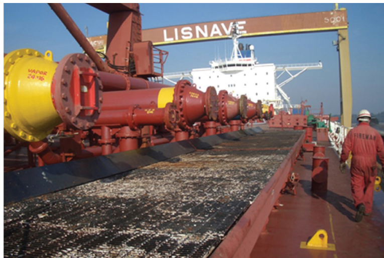
FIGURE 6.12 Upper deck of an oil tanker showing the manifold connections, seen inside the Lisnave dry dock complex.
