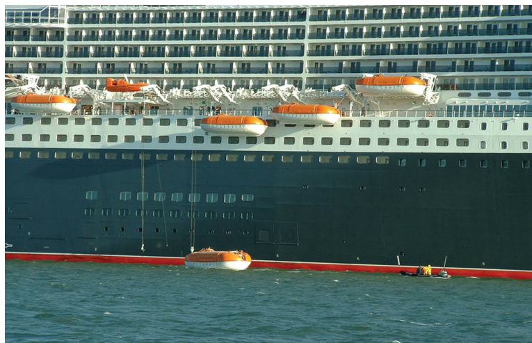
FIGURE 12.4 The passenger vessel Queen Mary 2 engages in a lifeboat launching drill while secured port side to, in Southampton. Partially enclosed boats are seen turned out and operating on the surface.
