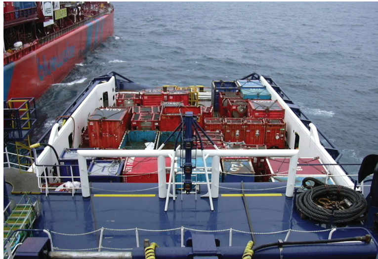
FIGURE 10.7 Deck load seen on offshore supply vessel Highland Courage (IMO No. 9249491). Alongside an FPSO in the North Sea. Loads are normally left pre-slung to ease discharge to FPSO or to the installation.
