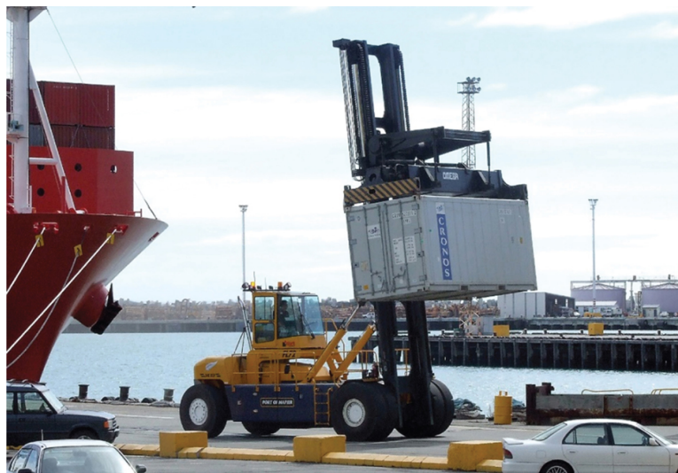
FIGURE 9.37 Mobile units working and stacking containers inside a container park. Heavy duty forklift truck engaged in ground handling the transport of container cargoes. Straddle trucks (elephant trucks) are also deployed at major terminals.
