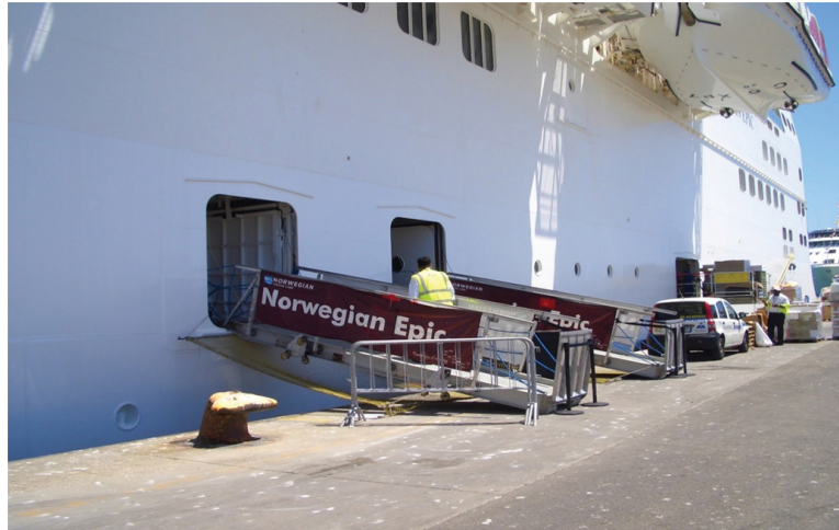
FIGURE 12.8 Twin short gangways are deployed from low shell doors set into the side of the Cruise vessel Norwegian Epic (IMO No. 9410569), rigged with safety gangway nets and quayside barriers with security watchman in place.
