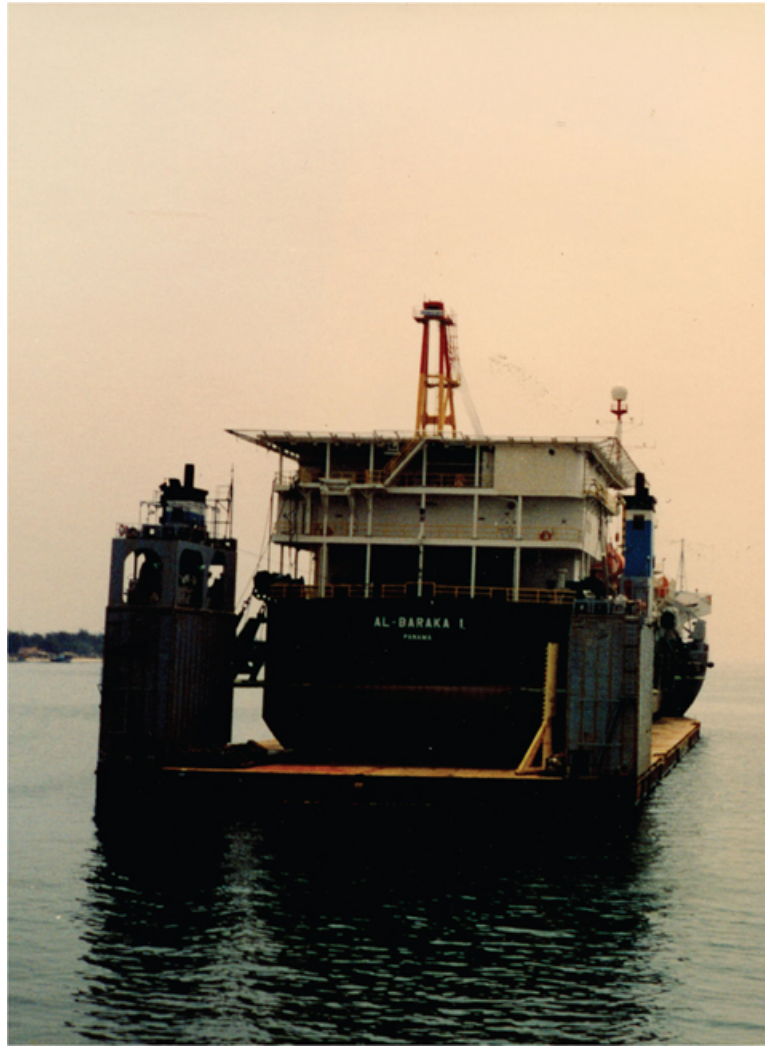
FIGURE 4.21 The semi-submersible ‘Super Servant 3’ as seen from astern carrying the crane barge Al-Baraka 7 , on its main weather deck.
