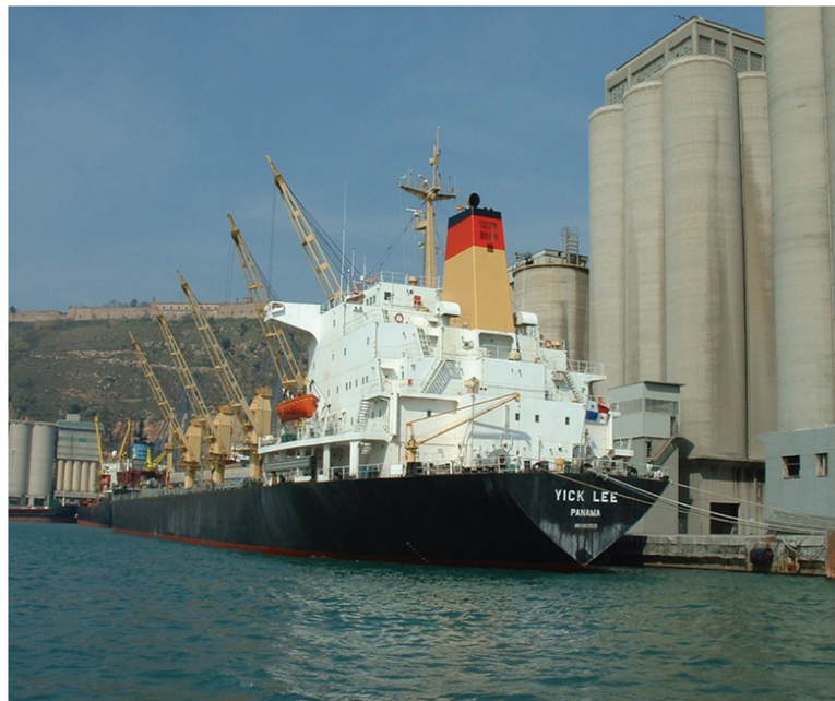
FIGURE 1.18 The bulk carrier 'Yick Lee' (IMO No. 8025525) seen starboard side to the grain berth, Barcelona, Spain. The ship has turned her deck cranes outboard to port to allow access for the suctions of the grain elevators to discharge a bulk cargo of grain.
