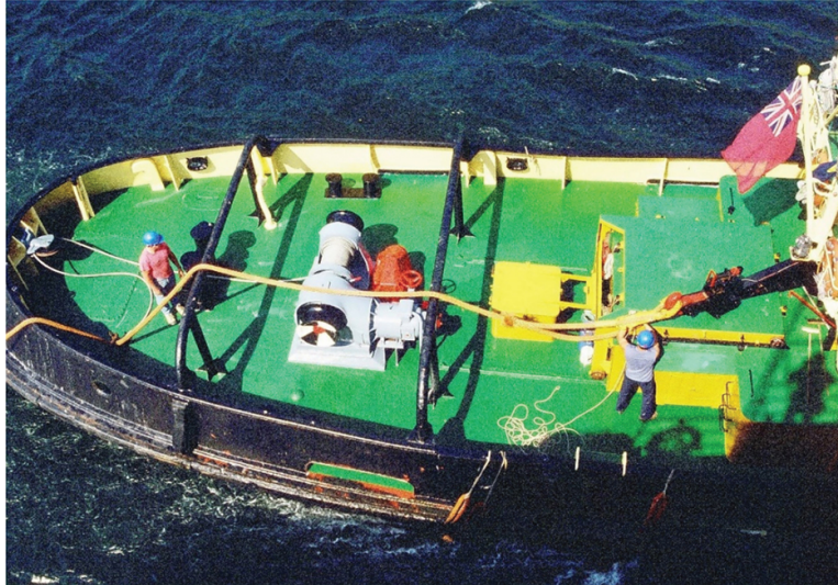
FIGURE 13.14 The deck shows the additional option to the use of the towing hook by way of the towing winch and use of a towing spring hawser. The winch can also be engaged to control the gob rope when deployed with a towing hawser.
