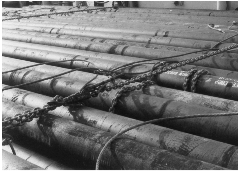
FIGURE 10.8 Steel pipes seen stowed on upper decks. Chain lashings are stretched across at intermediate lengths and tensioned by ratchet gear once in position. The pipes have been left pre-slung with wire snotters for speed of discharge.
