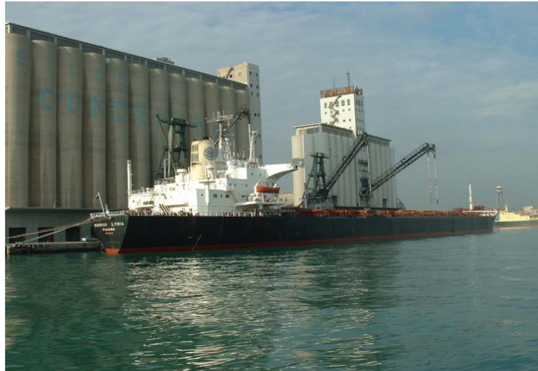
FIGURE 5.20 The bulk carrier Konkar Lydia (Grt 37,340) seen in the loaded condition with the grain elevation suckers poised above the hatches prior to commencing discharge.
