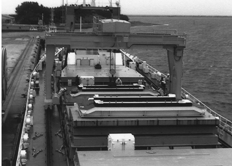
FIGURE 1.20 Example of a mobile tracked gantry crane in operation on the ships foredeck. Suitable for a vessel with all aft accommodation.
