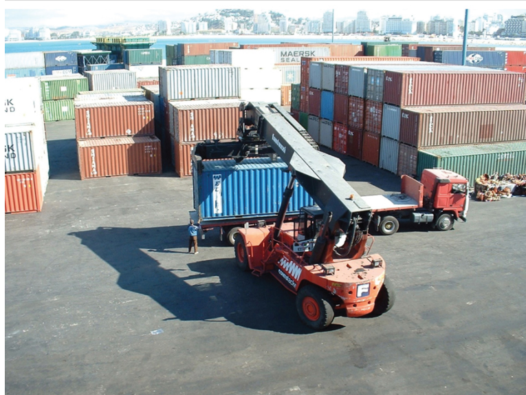
FIGURE 9.36 Tractor unit fitted with extending arm capable of carriage and stacking and loading containers to flat top transport vehicles.
