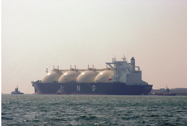
FIGURE 6.35 Large gas carrier seen manoeuvring with tugs in attendance. The four prominent spherical tank ‘domes’ are clearly identified above the uppermost continuous deck. Fully refrigerated spherical LNG tank, the protective steel dome protects the primary barrier above the upper deck. (No secondary barrier.) Double hull construction required in way of all cargo tank spaces.
