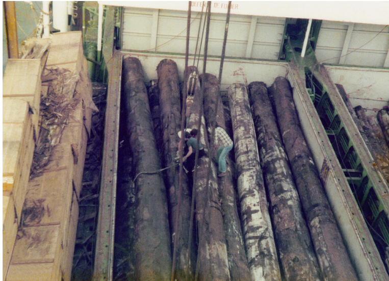
FIGURE 7.4 A cargo of heavy logs stowed under decks in twin hatches being discharged by multi-fold lifting purchase. Wire snotters are used to manoeuvre the logs to allow slings to be passed under, prior to discharging. Slings are often left in situ after loading to ease discharge, but not always. Sawn bundles of lumber are seen stowed at the hatch side as deck cargo.
