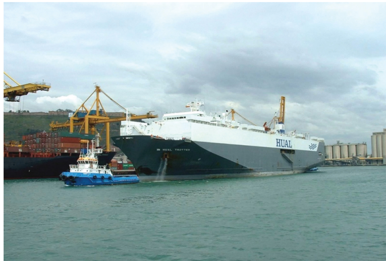
FIGURE 8.34 The high sided Hual Trotter (IMO No. 8116910) car carrier manoeuvres with tug assistance fore and aft in the port of Barcelona, Spain.
