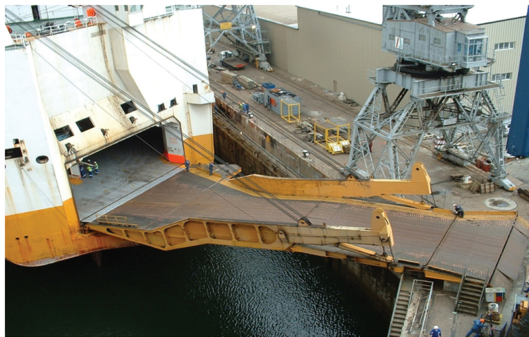
FIGURE 8.36 Angled stern quarter vehical ramp, extensively fitted to multi-deck car carriers.
