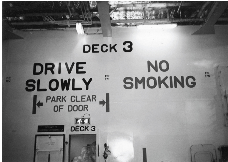
FIGURE 8.19 Typical bulkhead markings prominently displayed around vehicle decks to ensure safe and efficient loading of vehicle lanes.
