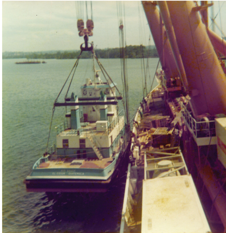
FIGURE 4.7 A heavy lift operation of an inshore and harbour work boat being lifted by a Stüelcken mast arrangement using the ramshorn hook with a double pendulum lifting purchase arrangement.
