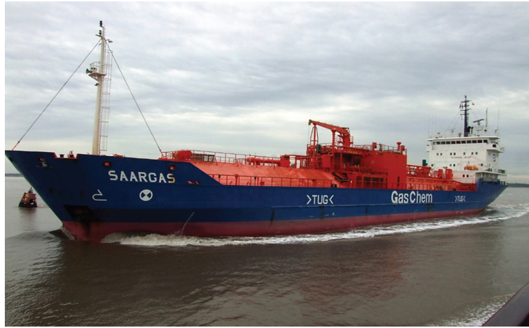
FIGURE 6.27 The Saargas (IMO No. 9135781) LPG /chemical carrier seen underway and leaving the River Mersey, Liverpool, England. The raised upper covers to the tank domes are prominent above the upper deck.
