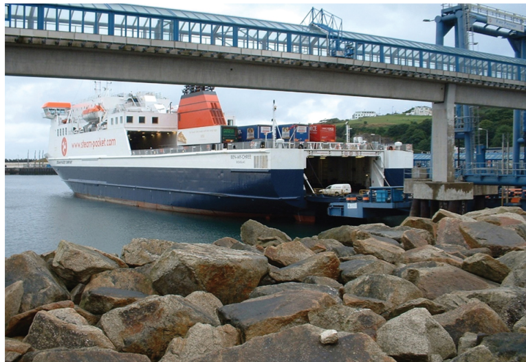
FIGURE 8.13 The RoPax Ferry Ben-My-Cree (IMO No. 9170705) seen stern to the vehicle link in Heysham harbour. The stern door/ramp is open and the vessel is loading vehicle cargo. Upper deck is already part loaded with drop trailer units.
