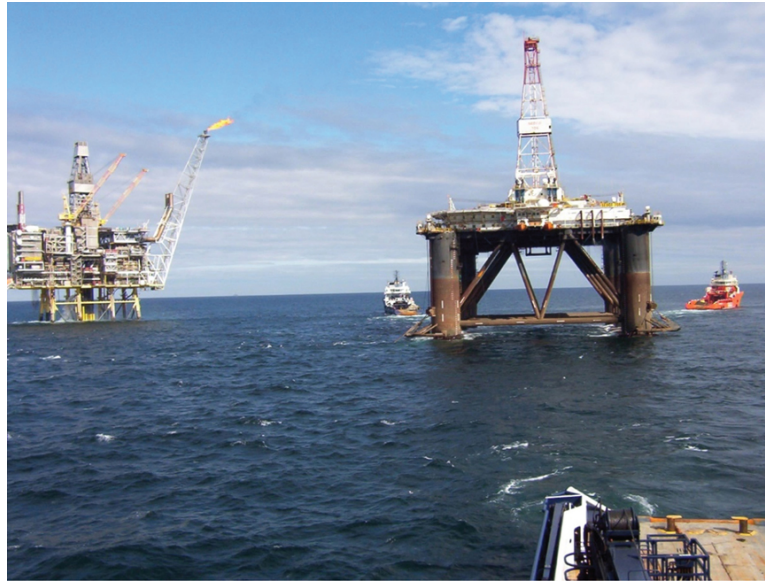
FIGURE 13.8 A semi-submersible moves her position with towed assistance from three stand-by/offshore support vessels. Seen passing a fixed North Sea oil installation.
