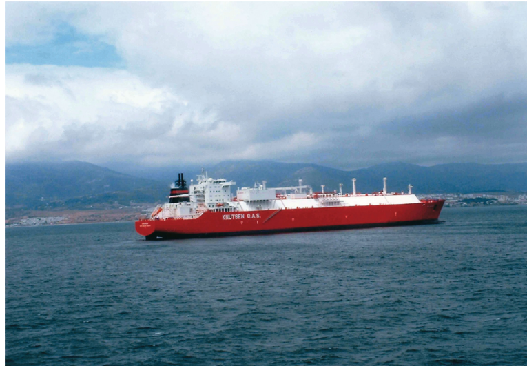
FIGURE 6.33 The LPG tanker Cadiz Khutsen (IMO No. 9246578) lies at anchor off Gibraltar. The vessel operates with membrane tanks and has a capacity of 138,000 m 3 .
