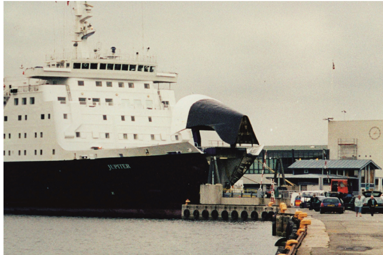
FIGURE 8.9 Bow visor arrangement on the RoPax vessel Jupiter (IMO No. 7360186) (since renamed) seen in the open position against the skyline. The bow-visor fitted with a stern ramp access permits a drive through capability.
