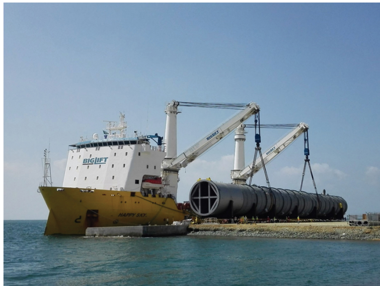
FIGURE 4.22 The Happy Sky (IMO No. 9457220) engages in a lift on lift off tandem lift of a long steel pipe section.
