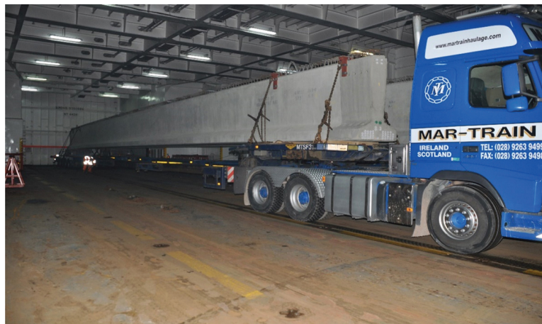
FIGURE 8.21 Long load seen on the main vehicle deck after the vehicle lashings have been removed and the unit is ready to discharge from the ferry Clipper Point .
