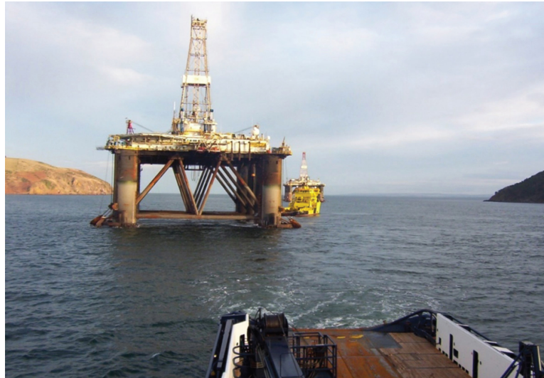
FIGURE 10.10 A semi-submersible drilling rig under tow by offshore multi-purpose supply vessels out of Invergordon, Cromarty Firth, Scotland. Installation moving and positioning is a regular employment of offshore vessels.
