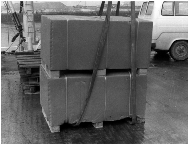
FIGURE 1.25 Canvas and nylon straps are more frequently employed with soft package materials like cardboard cartons. The straps are user friendly, strong and pliable, and cause limited damage.
