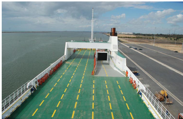
FIGURE 8.16 The upper vehicle main deck of the ferry Clipper Point . Vehicle lanes are clearly identified and trestles are positioned at the sides for use with drop trailer units.
