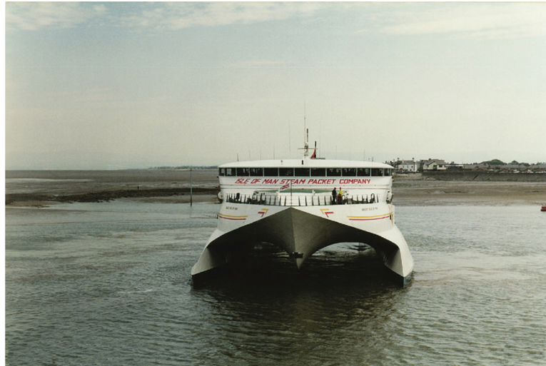
FIGURE 8.4 The modern face of Ro-Ro/Passenger (RoPax) type vessels. High-speed catamaran or trimaran hulls with vehicle access from a stern ramp. Generally engaged on the short sea trade. The Seacat Isle of Man (IMO No. 9176072) passenger/vehicle ferry engaged on the Irish Sea trade between Liverpool and the Isle of Man carrying vehicles and passengers.
