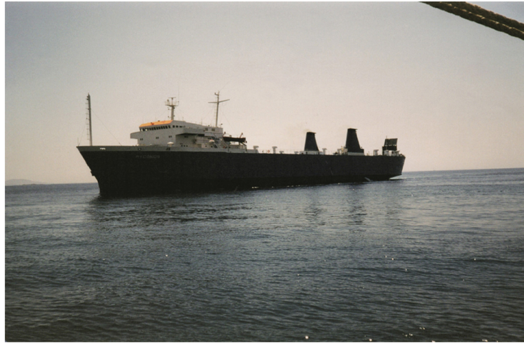
FIGURE 8.5 the MYKONOS modern Greek operated Roll on, Roll off ferry. Design features include all accommodation forward. A stern door/combined vehicle ramp right aft in the upright closed position when the vessel is at sea.
