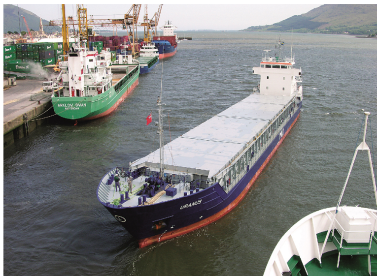
FIGURE 2.10 The container ship 'Uranus' seen docking at Warren Point, Northern Ireland. The vessel is viewed with all pontoon hatch covers in place, prior to loading containers below deck and up to three high on top of the steel covers.
