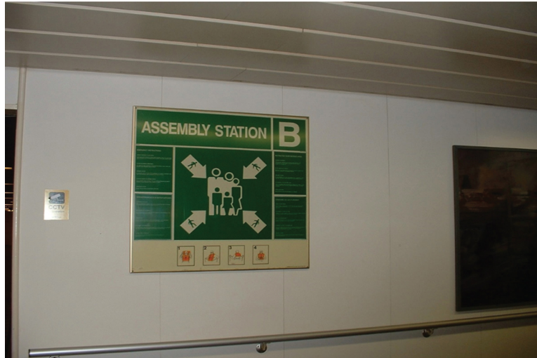
FIGURE 12.5 Emergency muster positions are usually identified specifically inside the rear of cabin doors with the emergency muster point localities. Signage in alleyways and around the vessel will highlight typical assembly stations.
