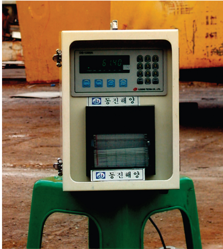
FIGURE 1.11 Example of digital load cell as employed in modern shipyards.
