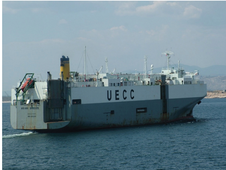
FIGURE 8.38 The quarter vehicle ramp of the vessel Asian Breeze (IMO No. 8202381) seen in the stowed and secured position while the vessel is at sea. A side ramp also stowed upright in a position just forward of the amidships position on the starboard side. The vessel is also fitted with a prominent freefall lifeboat in a launching position directly astern, a regular feature now of high-sided car carriers.
