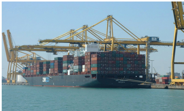
FIGURE 9.3 The container stack on the deck of the Zim Jamaica (IMO No. 9113680) being discharged by terminal gantry cranes in the port of Barcelona, Spain.
