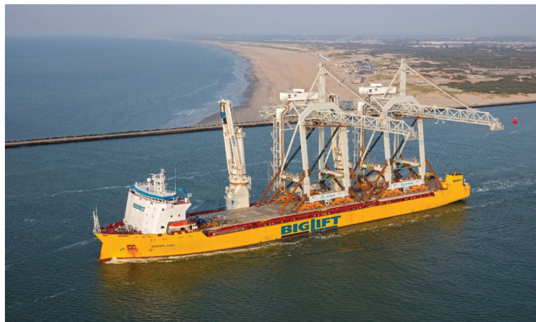
FIGURE 10.4 Overhead view of the port side of the Happy Sky (IMO No. 9457220) seen en route transporting two container gantry cranes as deck cargo. Such a load would have dictated a detailed stability assessment and would operate with an accurately assessed air draught.
