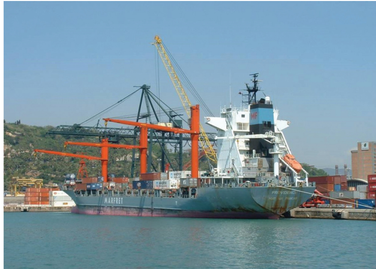
FIGURE 9.30 A single gantry crane and a mobile dockside crane work the container cargo of the feeder container vessel Providence (IMO No. 9080417). The ship's own container cranes are seen turned outboard to facilitate the shoreside loading systems in the port of Barcelona.
