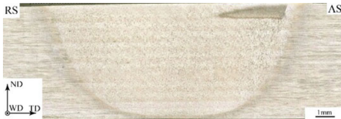
Fig. 3.11 Macrostructure of a Ti-6Al-4V SSFSW 2 joint [12]. Note ND normal direction; TD transverse direction
