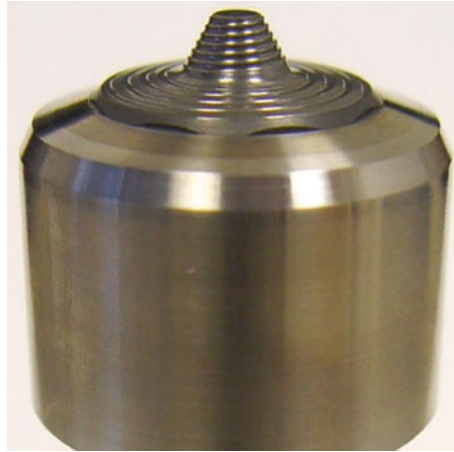
Fig. 4.6 FSR tool (70% PCBN/30% W–Re) [39]
