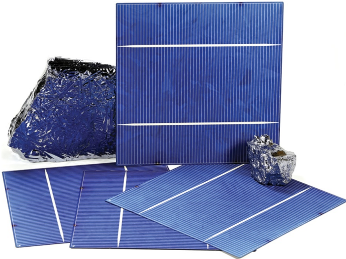
Figure 6.1 Chunks of raw polysilicon and the finished solar cells.
