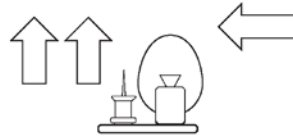
The plate moves further up vertically, allowing the camera to capture other parts of the egg
