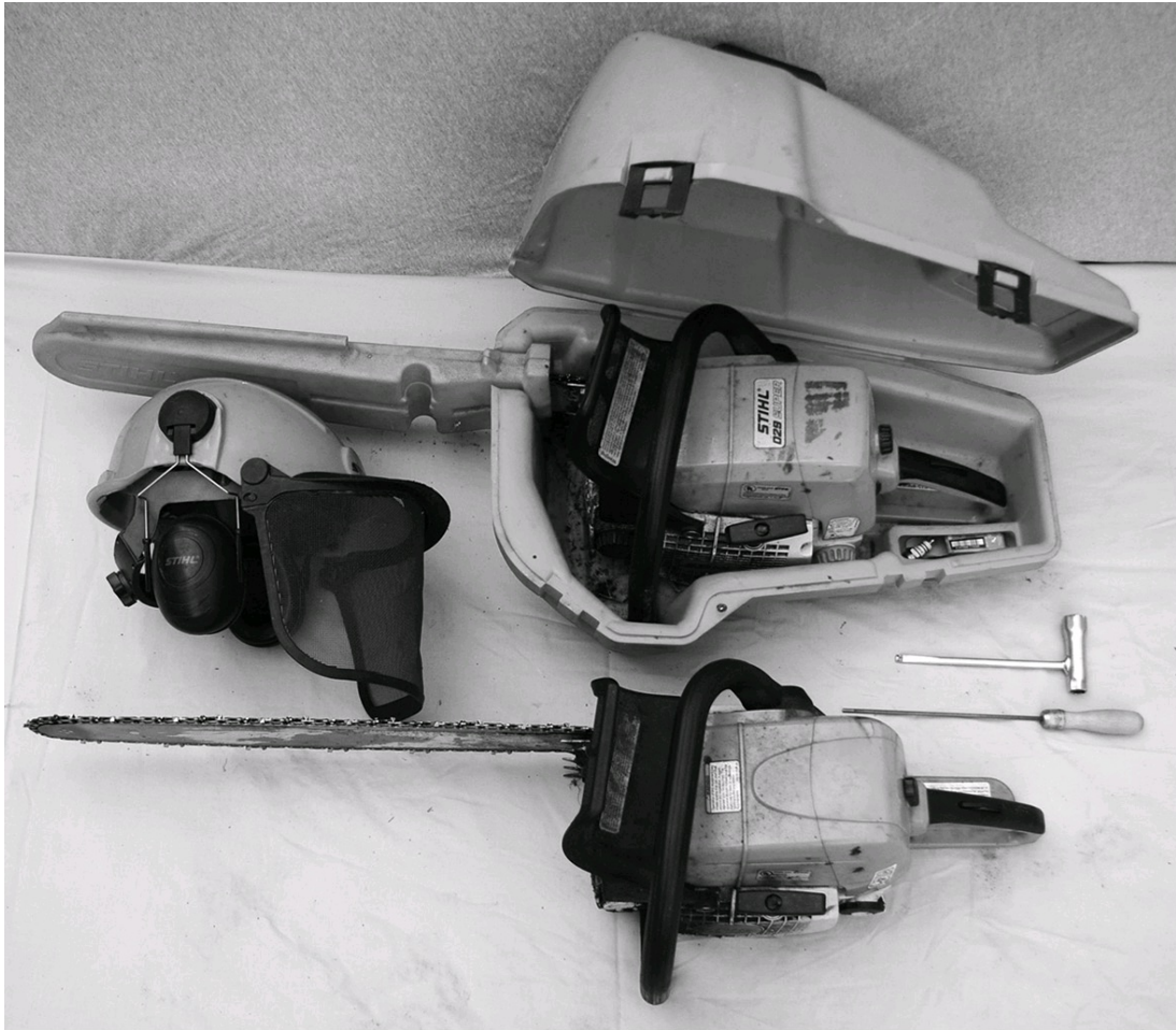
A pair of chain saws, combination tool, chain file, and a combination safety helmet (with integral mask and earmuffs)
