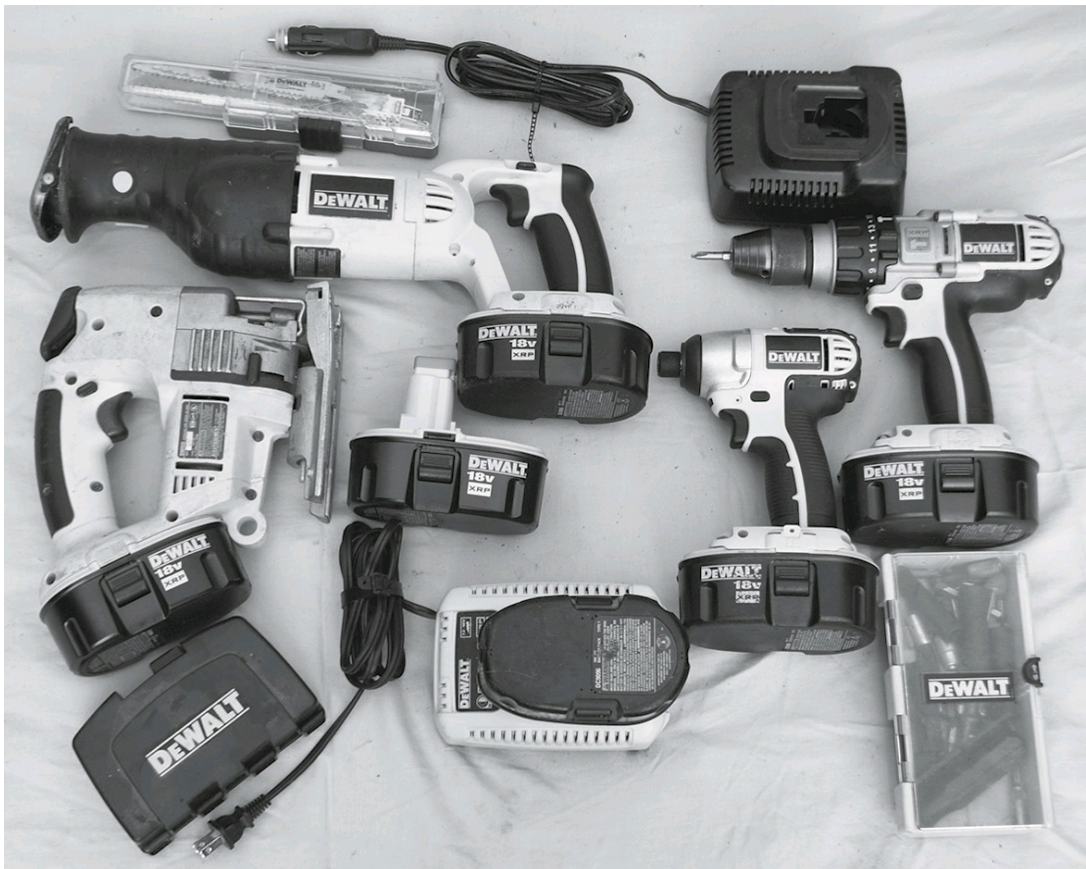
An assortment of DeWalt 18-VDC battery-powered tools and chargers (both AC and 12-VDC)
