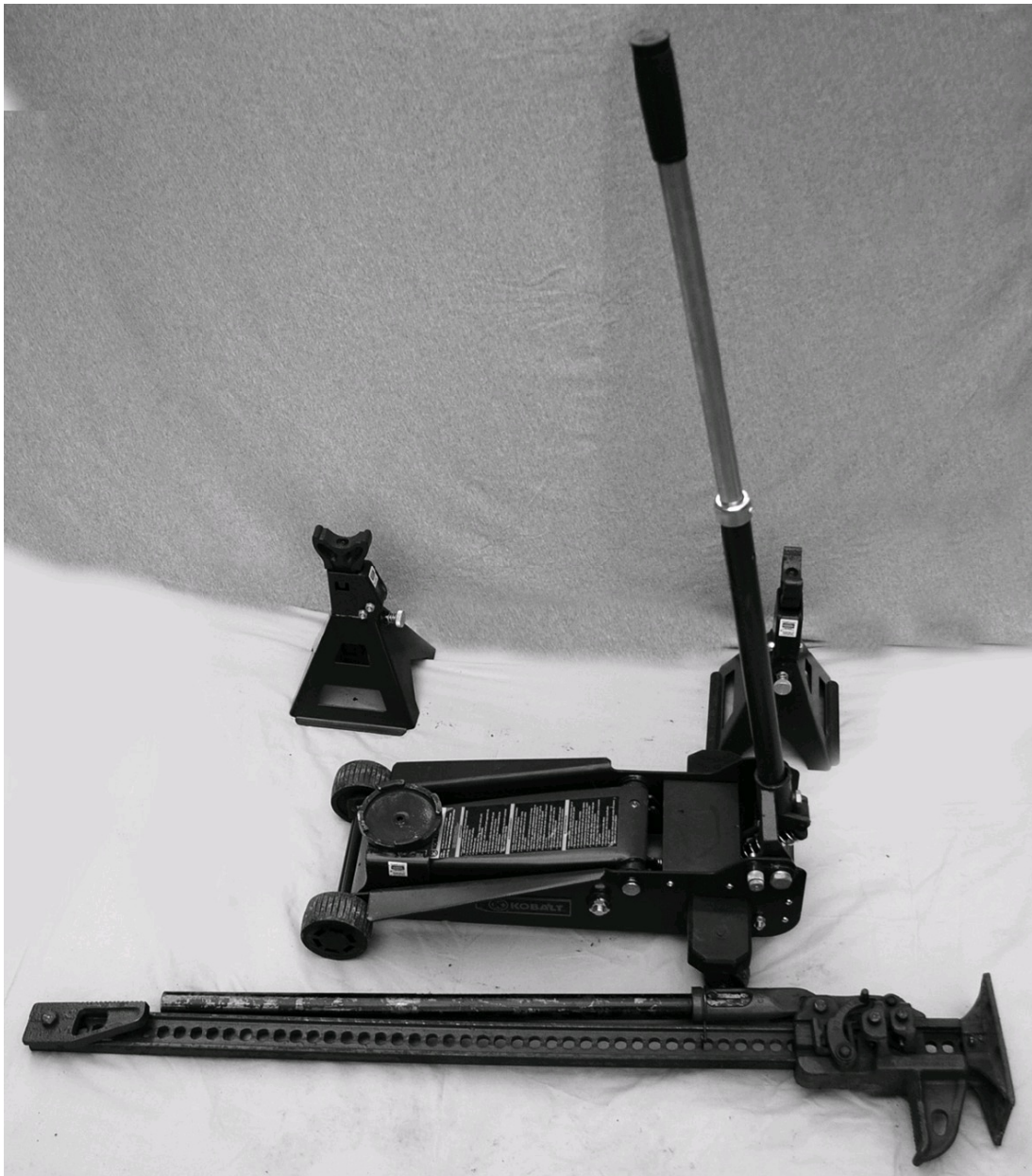
A pair of jack stands, a 3-ton floor jack, and a 48-inch Hi-Lift jack
