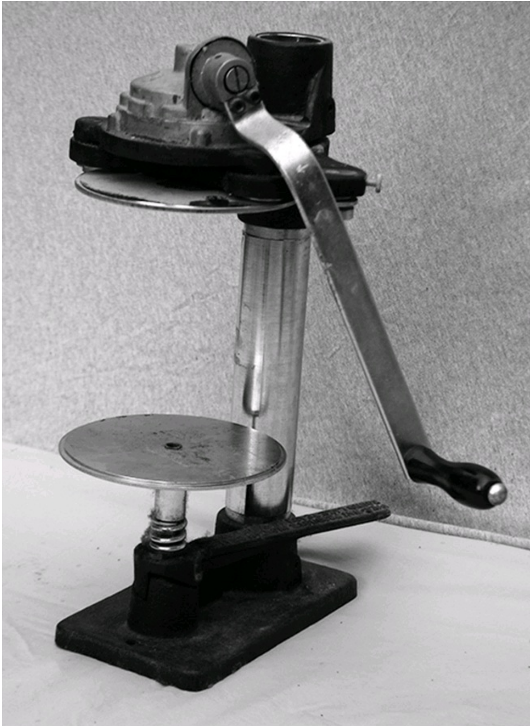
A dry-pack home-canning machine for #10 size cans
