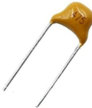
Figure 3-11. A ceramic capacitor with capacitance of 4.7 \mu\text{F}
