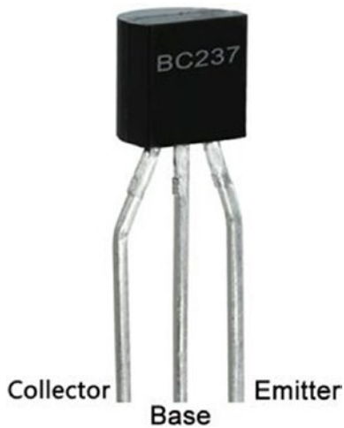
Figure 7-16. Base, collector, and emitter terminals of BC 237 transistor
