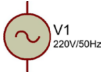
Figure 1-2. A sinusoidal source with peak value of 220\sqrt{2} = 311.12V and frequency of 50 Hz
