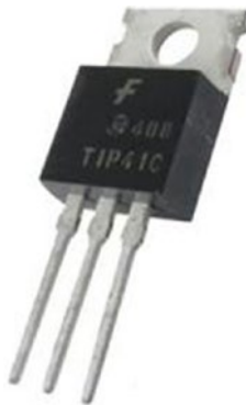
Figure 7-5. A BJT transistor with TO-220 package
