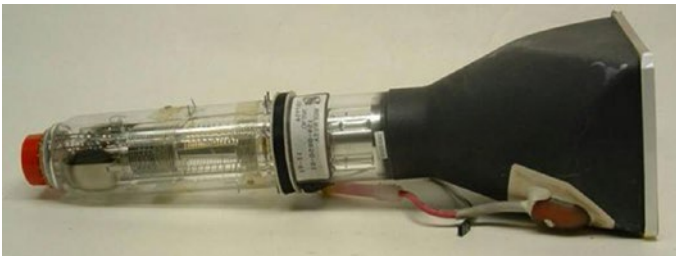
Figure 13-8. CRT of an analog oscilloscope
