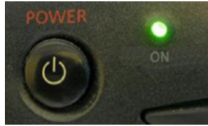
Figure 5-30. On LED shows the presence of input voltage
