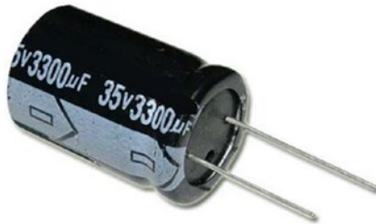
Figure 3-9. An electrolytic capacitor with working voltage of 35 V
