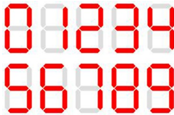
Figure 5-21. Displaying numbers on seven segment displays
