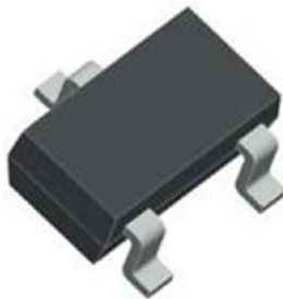
Figure 7-7. A BJT transistor with SMD package
