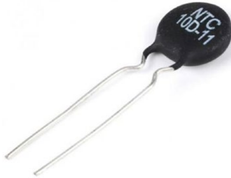
Figure 4-24. NTC type thermistor
