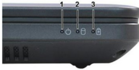
Figure 5-15. LEDs are used as indicator
