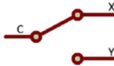
Figure 2-7. Common terminal is connected to X
