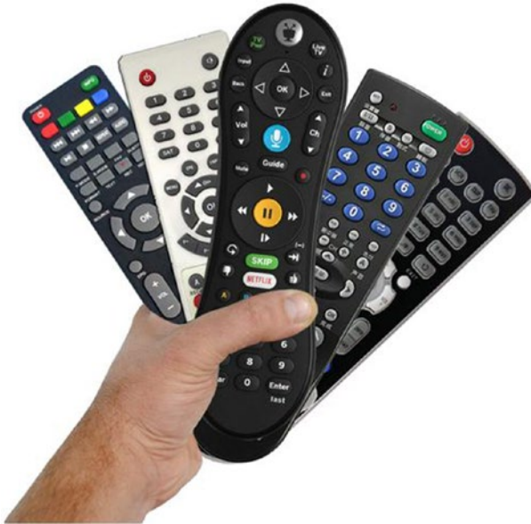
Figure 5-23. Most of remote controls use an infrared LED to send the commands
