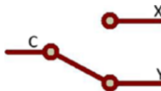
Figure 2-8. Common terminal is connected to Y
