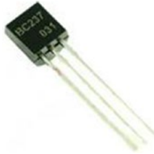
Figure 7-4. A BJT transistor with TO-92 package
