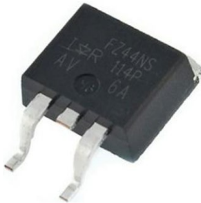
Figure 8-2. A MOSFET transistor with SMD package
