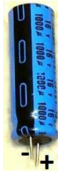
Figure 7-29. Negative terminal has a “-” marking and/or a colored strip along the can
