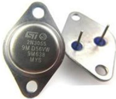
Figure 7-6. A BJT transistor with TO-3 package
