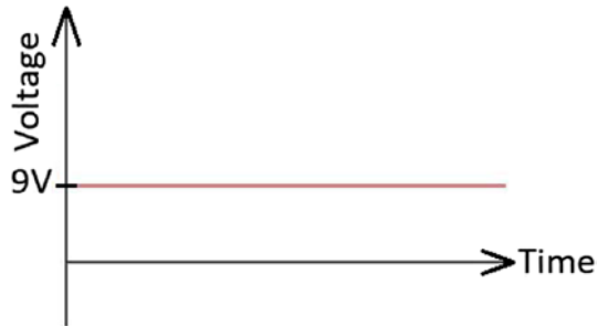
Figure 1-18. Voltage vs. time for a battery
