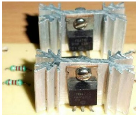
Figure 7-36. Transistors are mounted to the heat sink in order to decrease the device temperature
