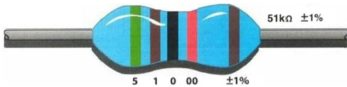
Figure 4-11. Resistor with five color bands
