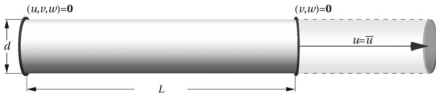
Fig. 8.1 Necking of cylindrical bar. Geometry and boundary conditions
