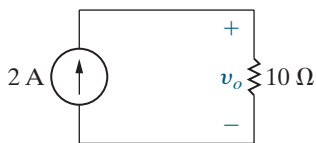
Figure 4.45 ▲ The circuit shown in Fig. 4.44 after combining sources and resistors.
