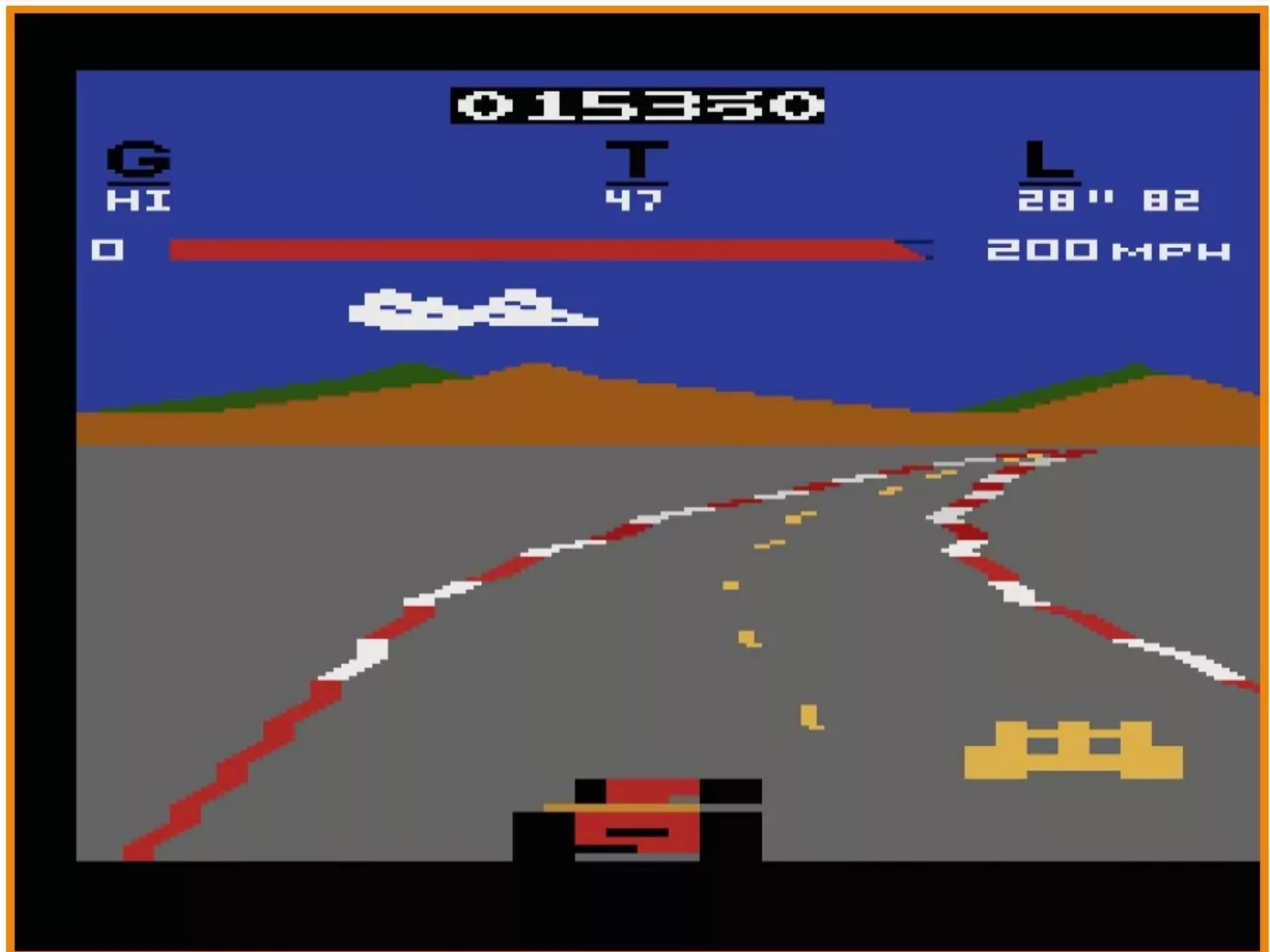
► [Atari 2600] Pole Position makes clever use of the missile and ball sprites to draw its roads.
