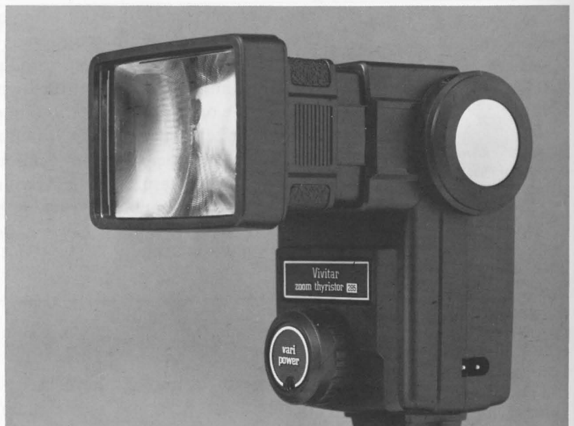
Figure 11-4. Electronic flash. Small portable electronic flash units often incorporate automatic exposure sensing. With this model, the sensor can be mounted separately on the camera if the flash is used from a different position (to side-light the subject, for example), thus ensuring that only the light actually reaching the camera is used for exposure control.
