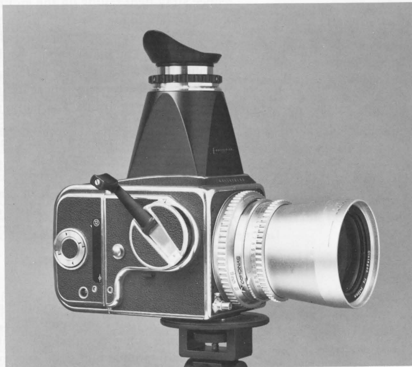
Figure 11-5. "Chimney" viewfinder for the Hasselblad. The finder shown includes a built-in magnifying lens to help with accurate focusing on the ground glass. The magnifier has a focus adjustment for the eye. Magnifiers without focus adjustment can be fitted with a corrective lens for users who wear glasses.
