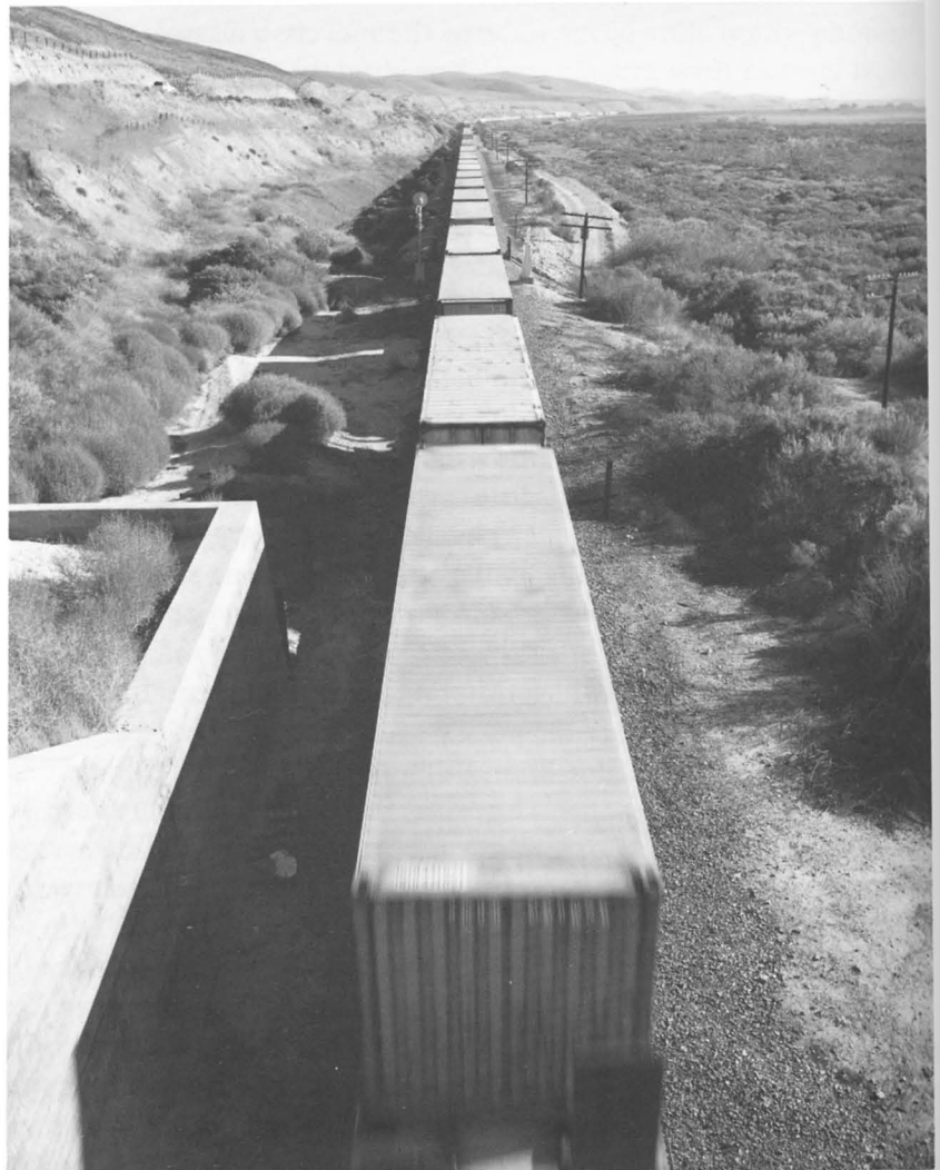
Figure 8-3. Train, near Salinas, California. This photograph of a rapidly moving freight train demonstrates that blur due to motion is related to distance. At an exposure time of 1/250 second, the near freight car shows movement, while the more distant cars are sharp.
