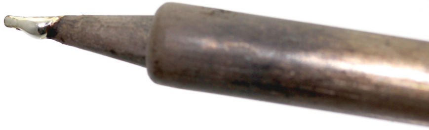
FIGURE 9-16: Tinning the tip helps to preserve your iron and makes soldering easier.
