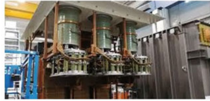
Actual three-phase rectifier transformer
