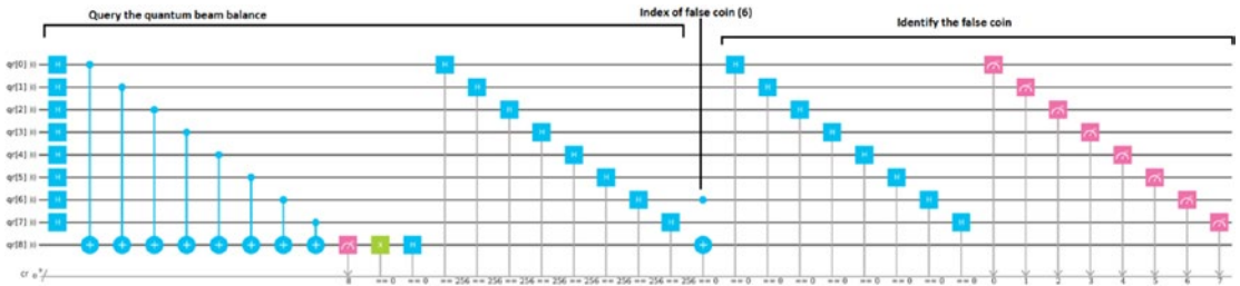
Figure 8-3. Quantum circuit for the counterfeit coin puzzle with N = 8 , k = 1 , and fake at index 6
