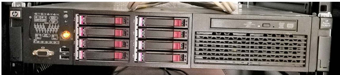
Figure 2.5: A rack-mountable server
