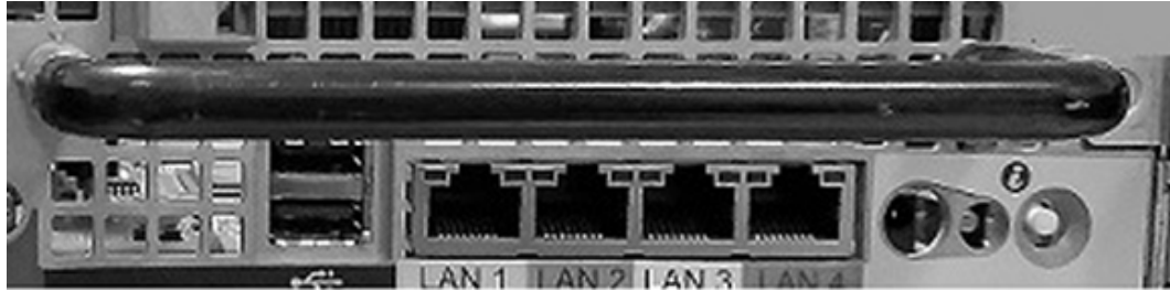
Figure 2.4: Network interfaces on a server
