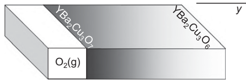
Figure 3.10 Set-up sketch of oxygen diffusion into half-space of \text{YBa}_2\text{Cu}_3\text{O}_6 .
