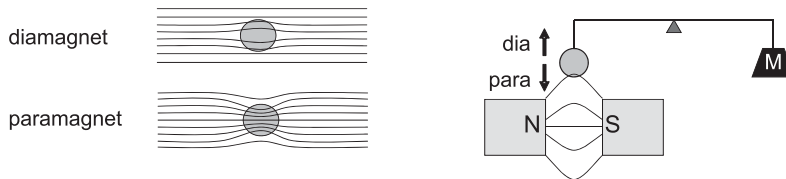
Figure 9.4 A paramagnet is attracted into the magnetic field, diamagnet is repelled; the paramagnet will appear to weigh more in the experiment sketched.
