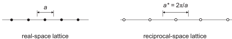
Figure 6.2 The 1D real- and reciprocal-space lattice. In the latter, the interval that is marked corresponds to the first Brillouin zone.
