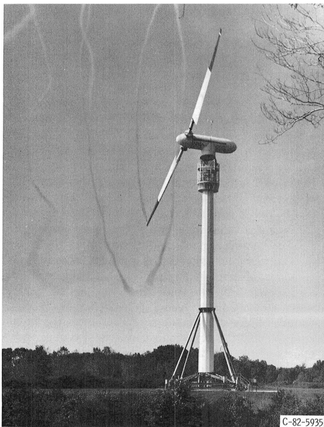
Figure 62. — Rotor blade tip vortex experiment with blade tip smoke generator—Mod-0 wind turbine.
