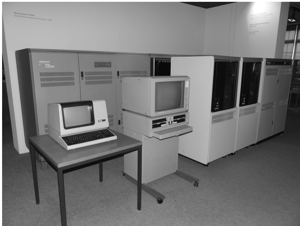
Figure 7-17 Digital Equipment Corporation VAX 11/780 minicomputer and terminals (Source: Bernd Gross, CC-BY-SA-4.0, https://commons.wikimedia.org/wiki/File:VAX_11-780_und_Nachentwicklung_K_1840_TSD.JPG )
