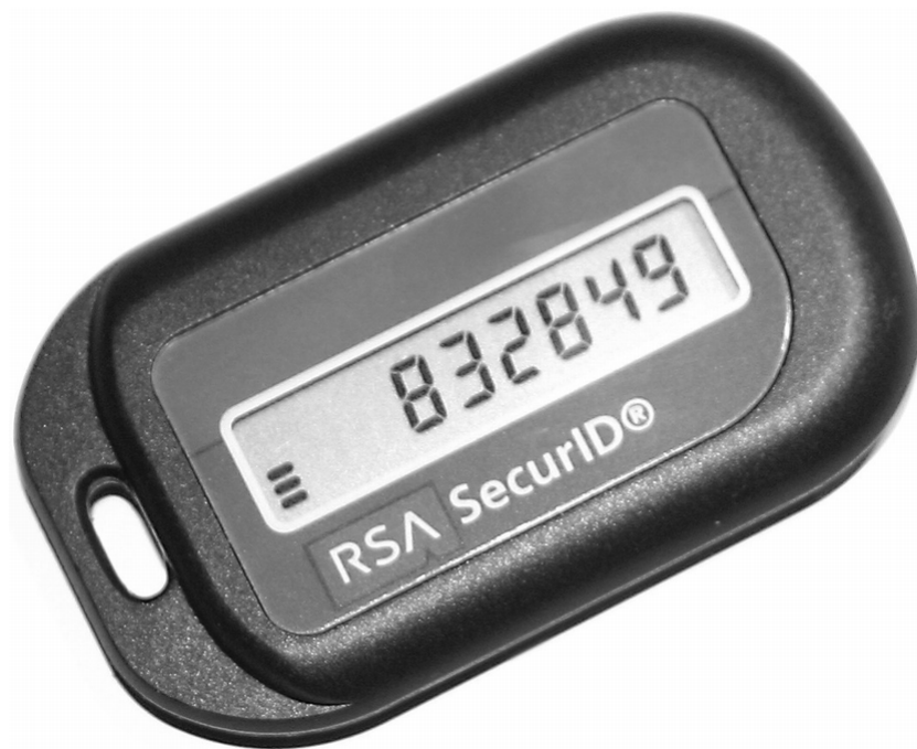
Figure 2-11 An RSA SecurID Token. It displays a code on the screen that is unique to the device and changes on a regular interval. Image downloaded from Wikimedia Commons ( commons.wikimedia.com ) and licensed under Creative Commons Attribution-Share Alike 1.0 Generic license ( https://creativecommons.org/licenses/by-sa/1.0/deed.en )
