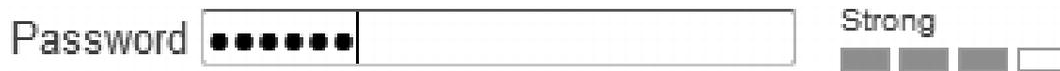
Figure 2-9 An example password meter from the 2013 time frame. More recent password meters typically provide some feedback on what is wrong with the password
