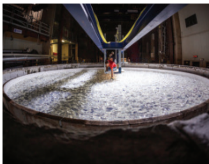
Under a university football stadium in Tucson, a technician checks fired glass that will become a mirror in the Giant Magellan Telescope.
