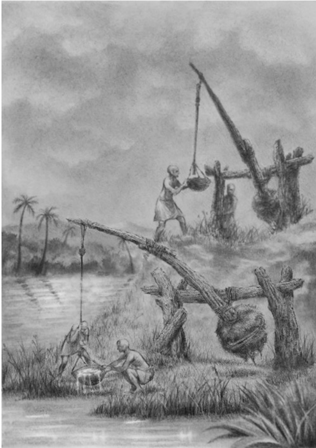
Figure 5-1. Use of Shaduf by ancient humans to help draw water from river
