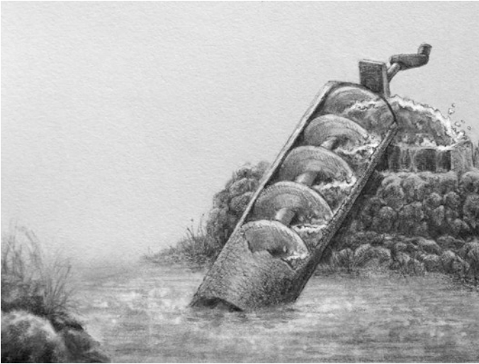
Figure 5-4. Showing the innards of Archimedes' screw helping irrigate by drawing water from river
