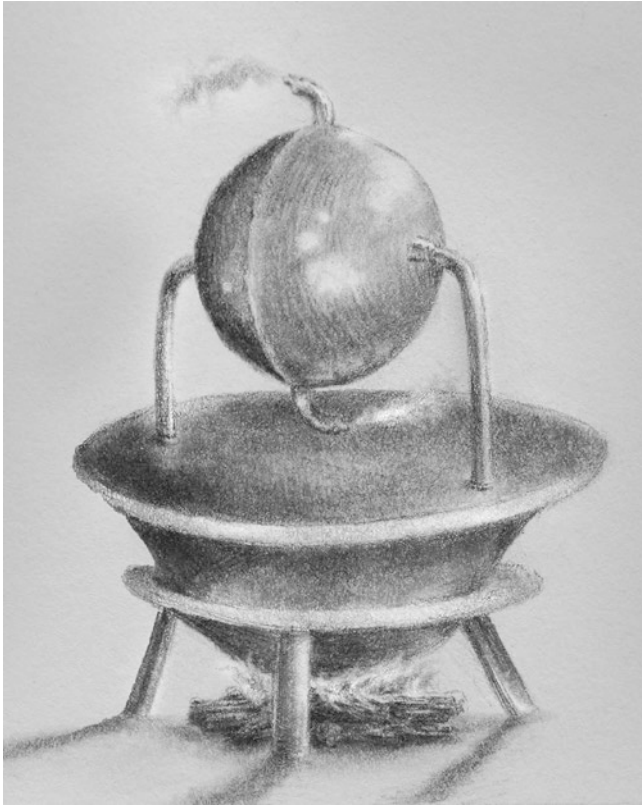
Figure 5-7. Aeolipile was the probably one of the earliest inventions that converted heat energy into motion
