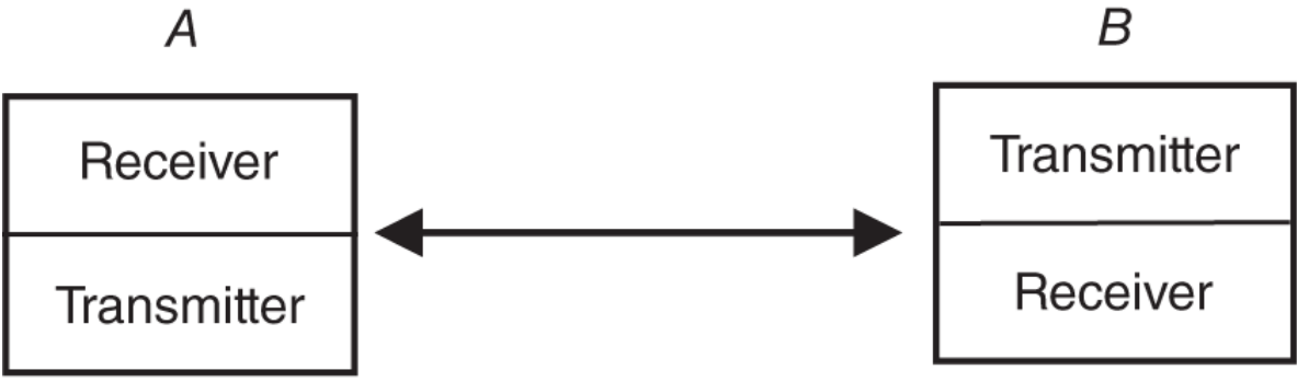
Half-duplex ( A-to-B or B-to-A take turns)
