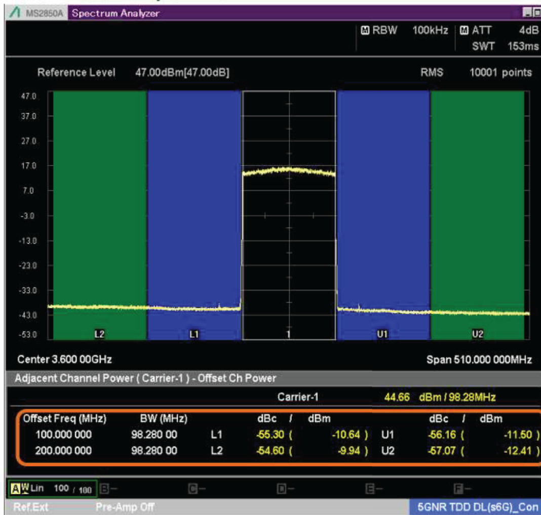
Figure 9.13 Illustration of adjacent leakage power ratio (ACLR).
