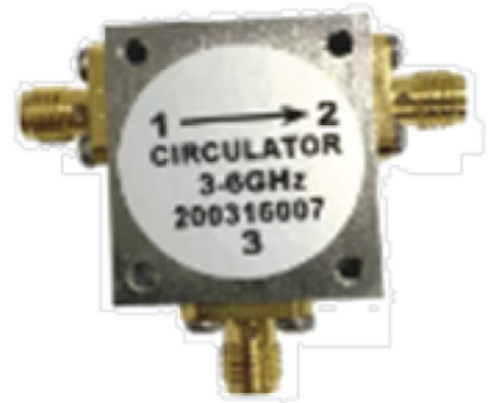
Figure 5.26 Photo of a commercial circulator and a diagram of a transceiver frontend using a circulator.
