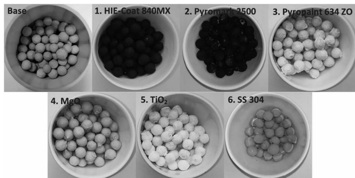
FIGURE 13.3 Photographs of the cured coated samples (MP 3). The uncoated Denstone 2000® is seen in the base sample. The average hydraulic diameter of a particle is 6 mm.
