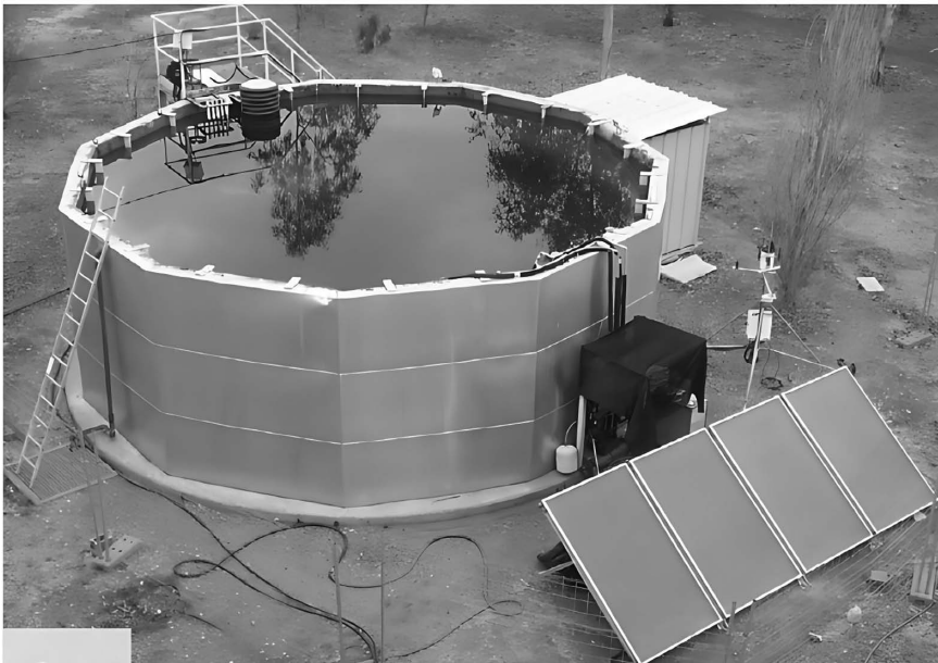
FIGURE 6.15 Experiment setup for solar pond with collectors.
