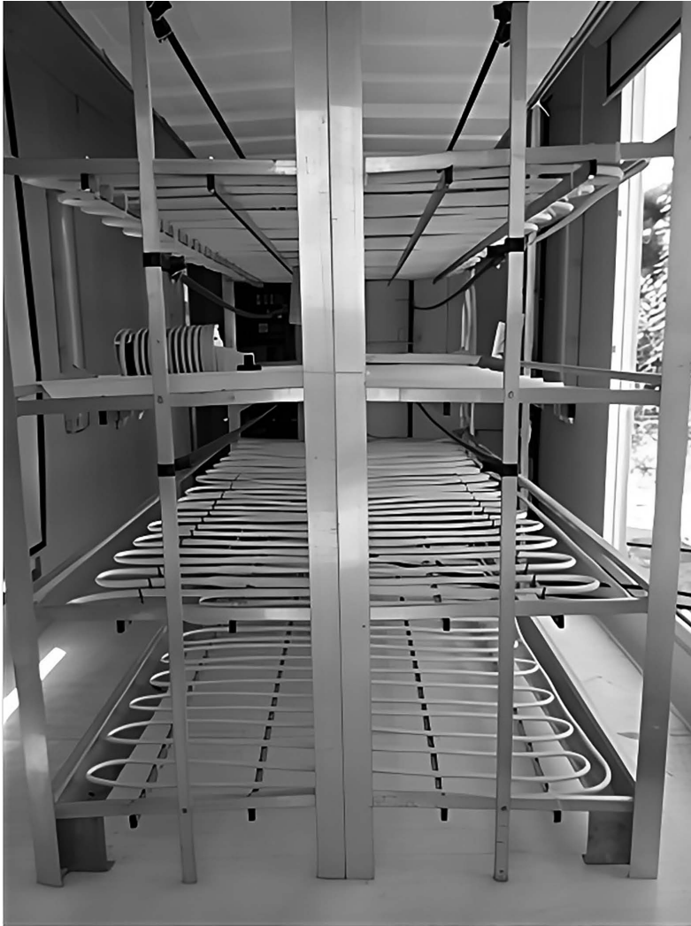
FIGURE 9.3 The multi-stage exchanger system.
