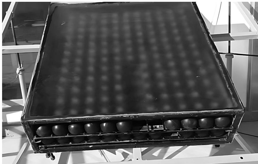
FIGURE 9.7 Solar heating system with latent heat storage.
