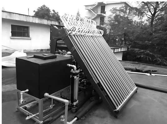
FIGURE 6.12 Water heating system with oscillating heat pipe.
