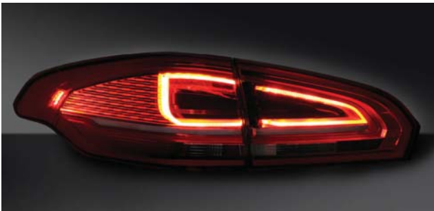
Figure 4.21 Light guide for automotive tail lighting using a light guide optics concept. Source: Image from FORVIA Hella.
