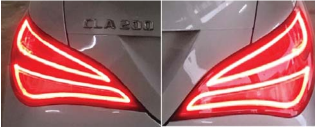
Figure 4.18 The Mercedes CLC200 tail lamp, while a very flat design, gets a “tunnel look” and a sense of depth from its LEDs and their multiple reflections.
