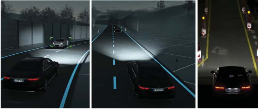
Figure 4.13 Digital matrix headline is automatically switching on or off at a very fine resolution depending on the traffic situation. Source: REC Anything [15].
