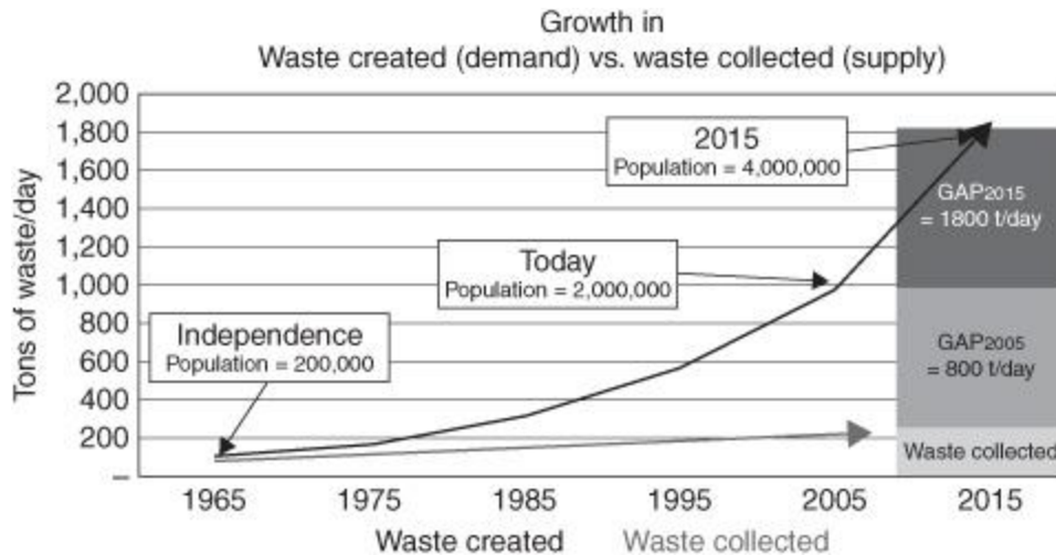
FIGURE 16-6 Current and future gaps of waste created versus collected in City A.
