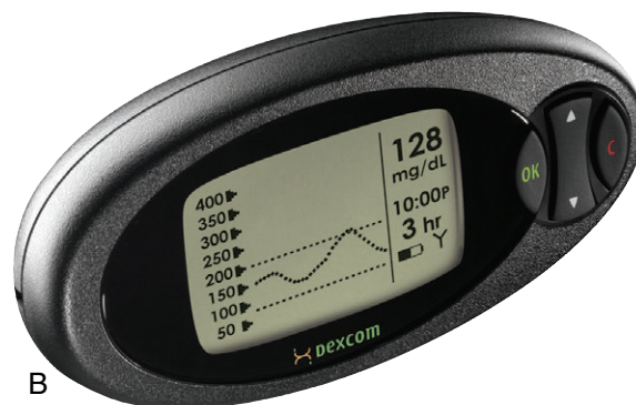
FIG 43-6 A, Tiny sensor implanted under skin transmits continuous reading to receiver. B, Monitor displays and stores readings. (Courtesy DexCom.)
