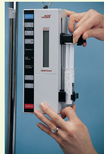
STEP 7c(3) Ensure that syringe is secure after placing it into mini-infusion pump.
