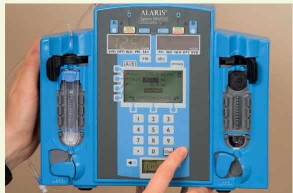
STEP 7b Select rate and volume to be infused and press start button.
