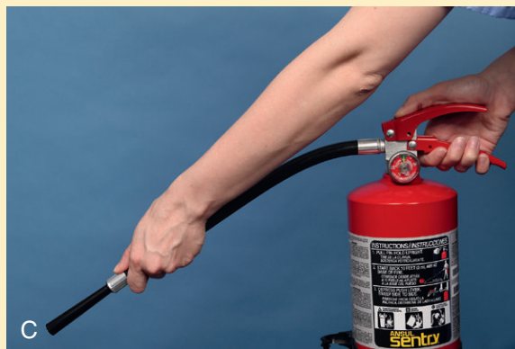
STEP 7b(1)(a-c) A, Pull safety pin from fire extinguisher. B, Aim nozzle of hose at base of fire. C, Squeeze handle while sweeping side to side with nozzle.
