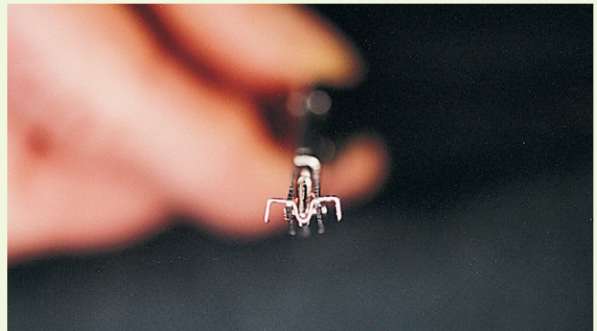
STEP 11c Metal staple removed by extractor.
