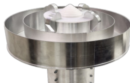
◀▼ DSA-2000 Artist’s concept of one of the 5-meter dishes of the DSA-2000, along with its antenna feed ( below ), built with parts from a baking company.
