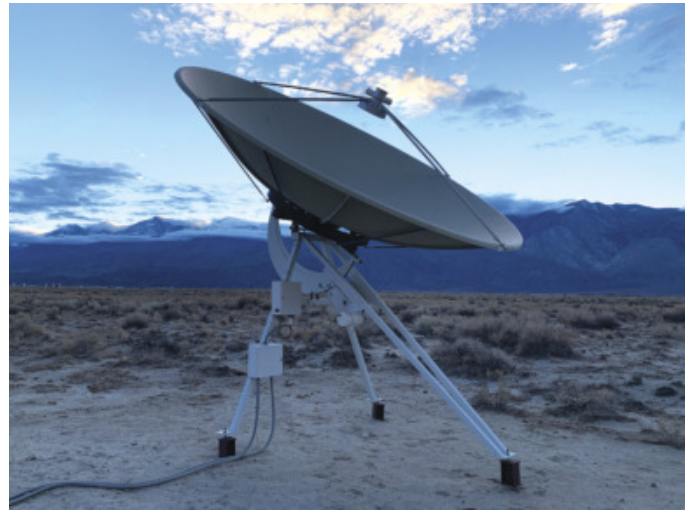
▲▼ DSA-110 DSA-2000’s precursor is already up and running, with a dense, T-shaped core of antennas ( below ) and 15 more individual dishes spread out over 2.5 km ( above ).
