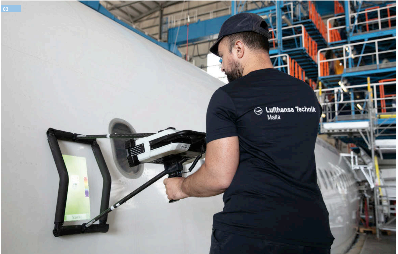
03 Augmented reality rig to help scan for superficial damage
