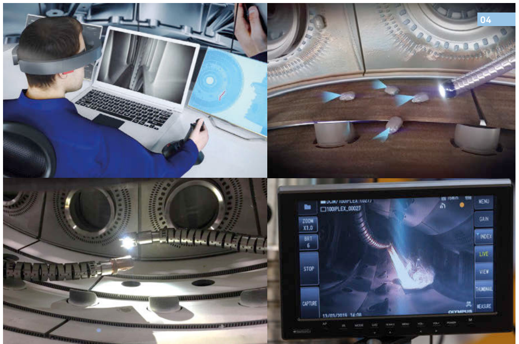
04 Rolls-Royce’s maintenance innovations, clockwise from top left: Cobra, being controlled by AR; Swarm; FLARE, flame-spraying; and FLARE, exploring
