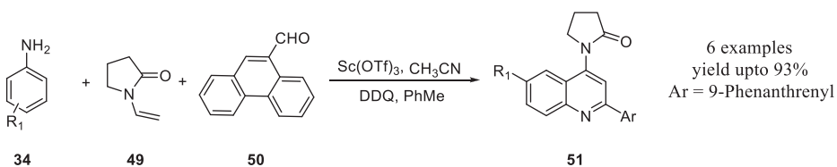
Figure 3.19: Pavarov multicomponent assembly of quinolone catalyzed by \text{Sc}(\text{OTf})_3 .
