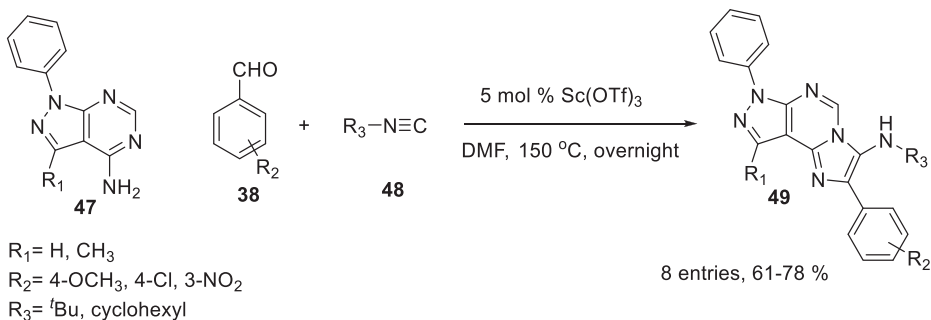
Figure 10.18: Sc(OTf) 3 -catalyzed synthesis of fluorescent imidazo[1,2-c]pyrazolo[3,4-e]pyridines.
