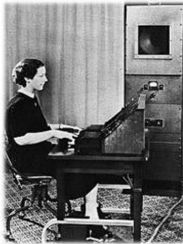
Figure 16.20 The Voder developed by Homer Dudley of Bell Labs at the 1939 World's Fair in New York. The operator worked at a keyboard, with a wrist bar to control the voicing parameter and a pedal for pitch control.
