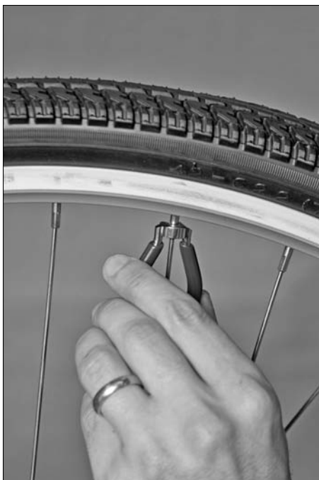
Figure 7-14: Using a spoke wrench.
