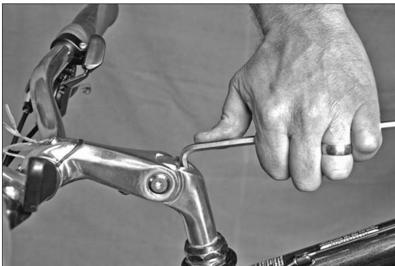
Figure 15-18: Loosening the socket head bolt.
