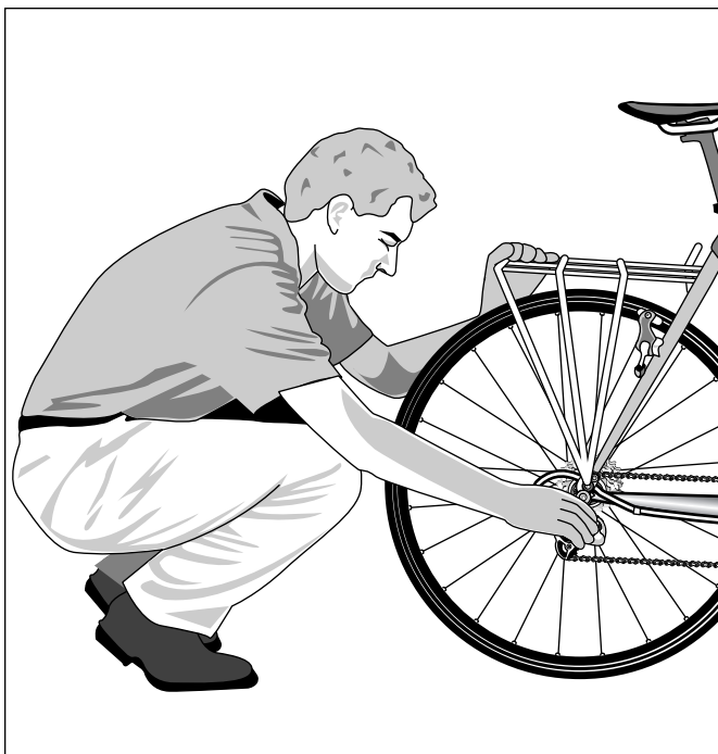
Figure 12-5: Checking the frame from the back.
