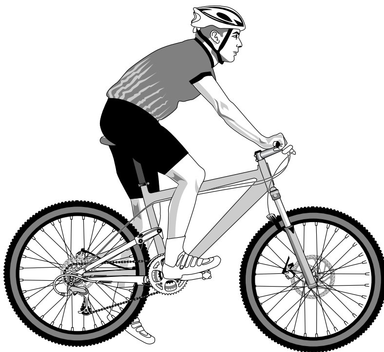
Figure 18-2: The proper saddle height.
