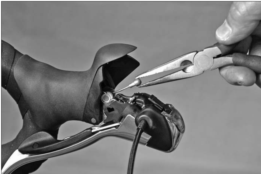
Figure 8-20: Removing the cable.
