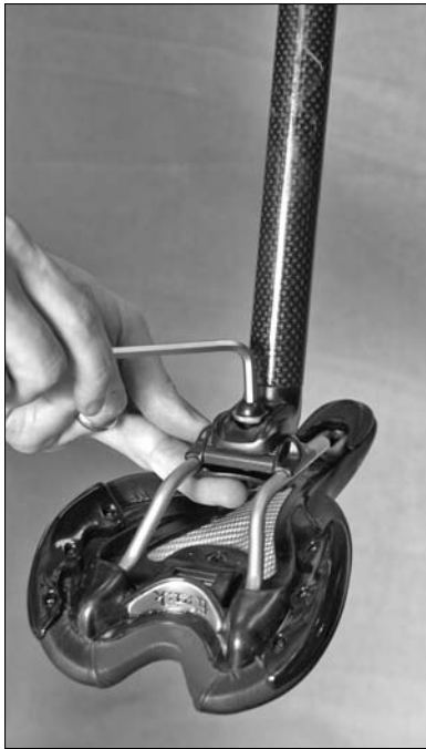
Figure 9-7: Attaching a two-piece clamp.
