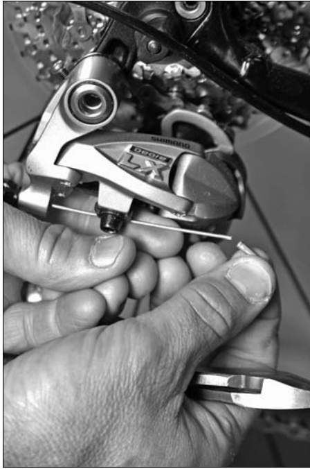
Figure 14-9: The cable cap.
