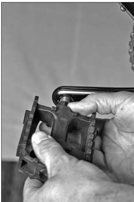
Figure 13-4: Reattaching the pedal.
