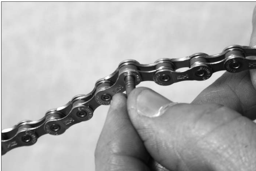
Figure 10-14: Inserting the pin.
