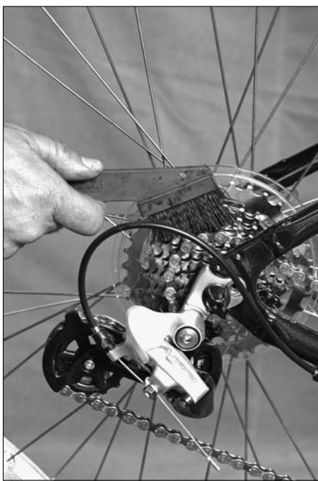
Figure 16-1: Using a brush to clean the sprockets.
