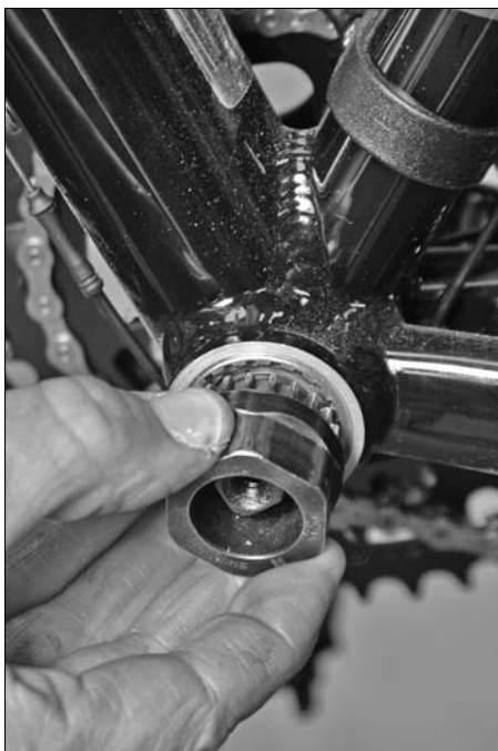
Figure 13-11: Attaching a bottom bracket tool.
