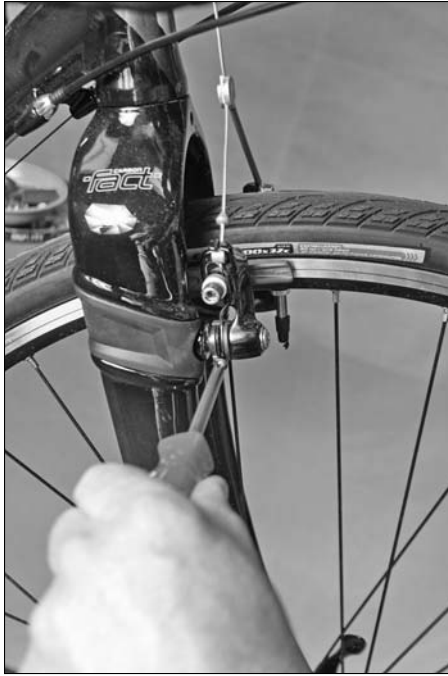
Figure 8-13: Adjusting brake tension.
