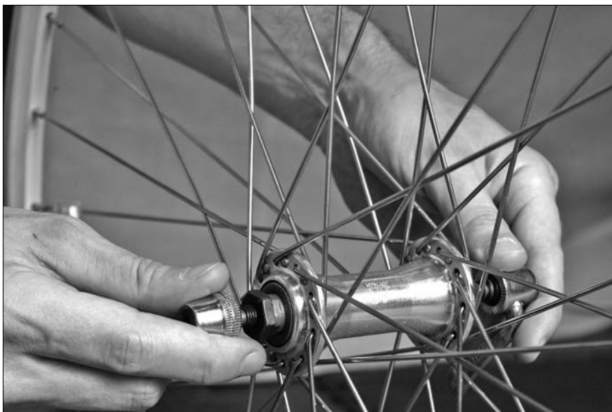
Figure 7-2: Removing a quick- release wheel.
