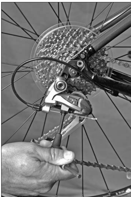
Figure 14-8: Attaching the cable.
