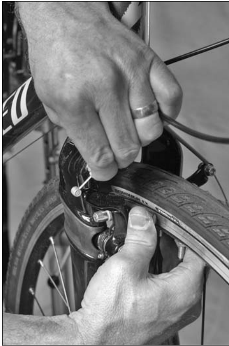
Figure 8-6: Undoing the quick- release.
