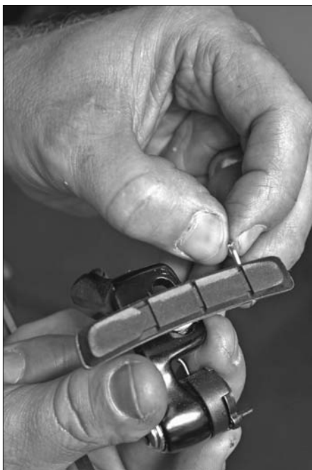
Figure 8-9: Removing the brake- pad pin.
