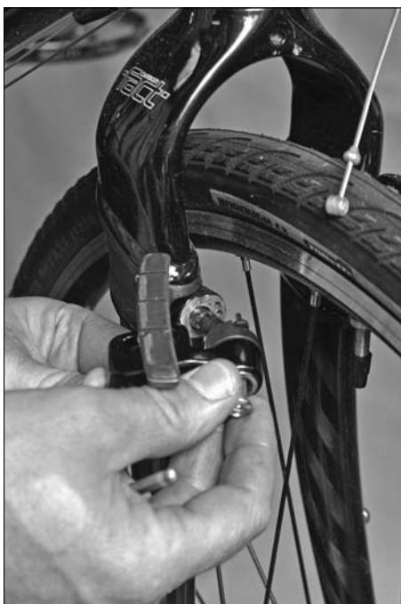
Figure 8-8: Removing the brake.
