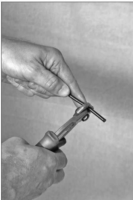
Figure 8-21: Cutting the cable housing.
