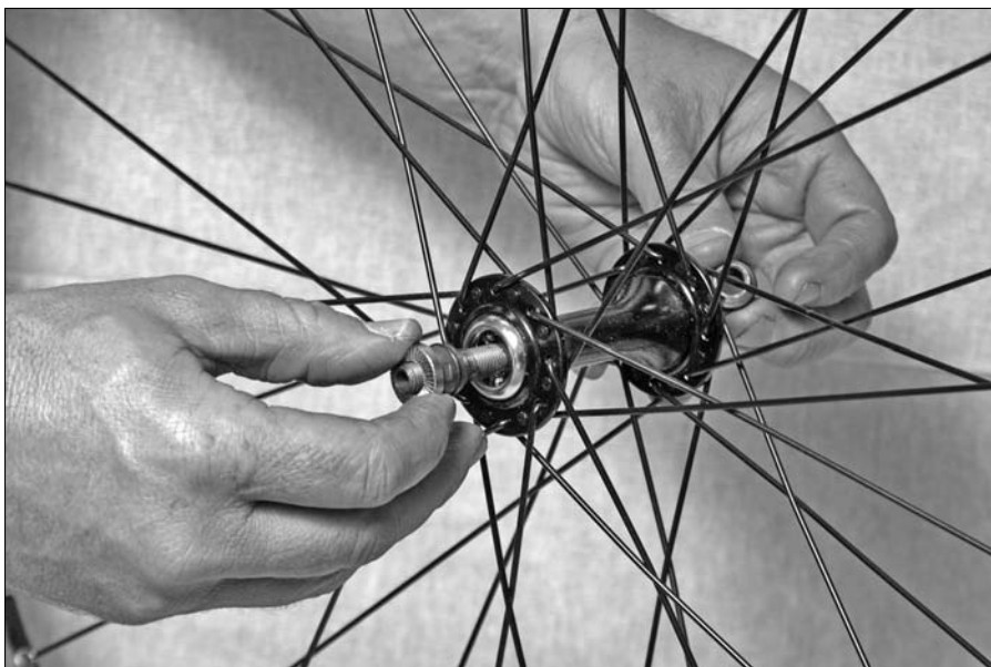
Figure 7-6: Removing the axle.
