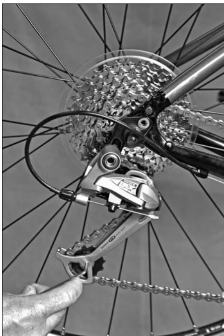
Figure 14-2: Loosening the bottom jockey wheel.
