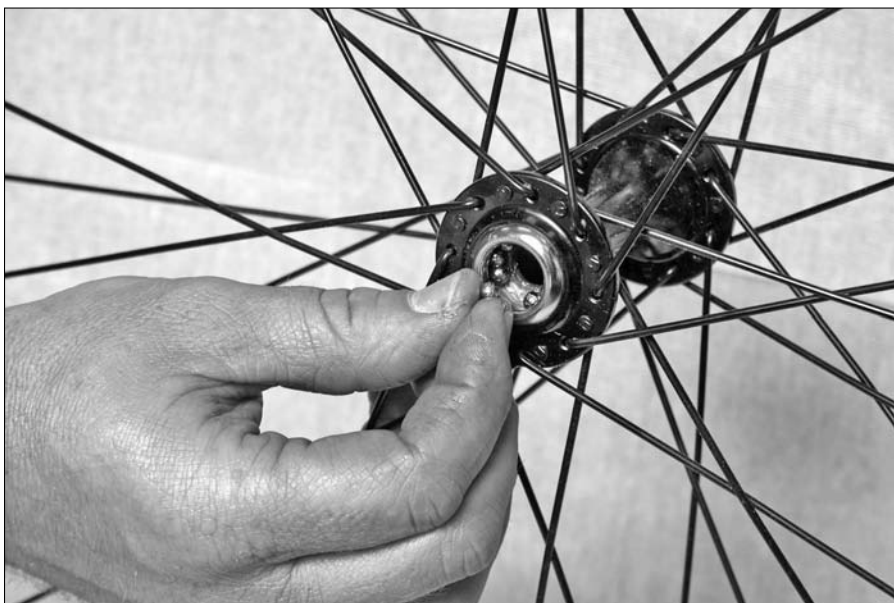
Figure 7-7: Removing the bear- ings.
