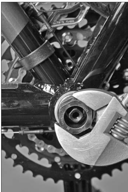
Figure 13-12: Using the bottom bracket tool.
