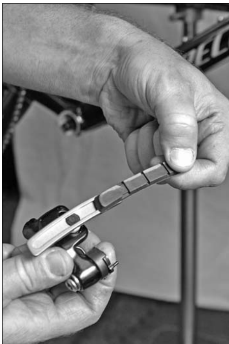
Figure 8-10: Removing the brake pad.
