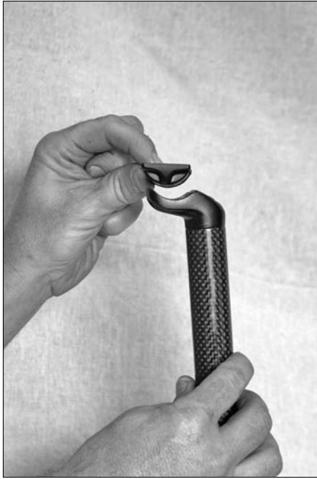
Figure 9-6: One piece saddle dis- assembled.
