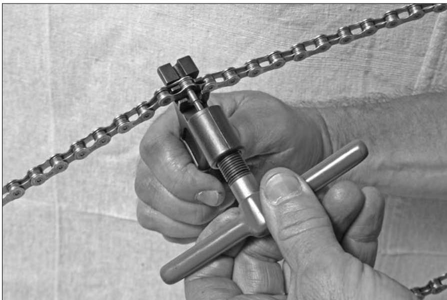
Figure 10-11: Preparing to separate a chain
