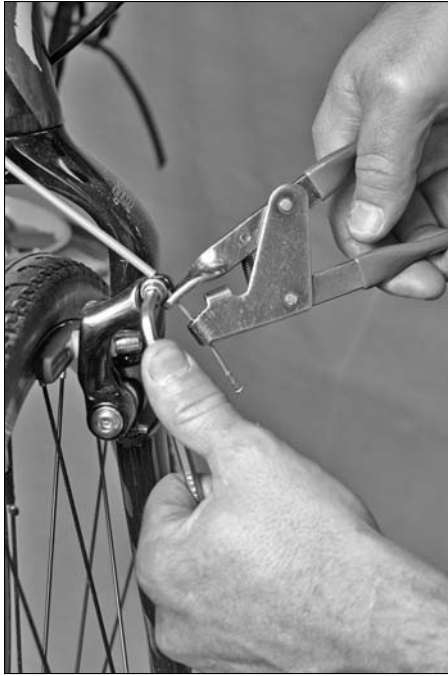
Figure 8-11: Using a fourth-hand tool.
