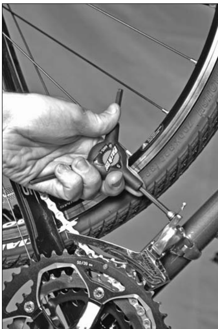
Figure 14-11: Removing the cable.
