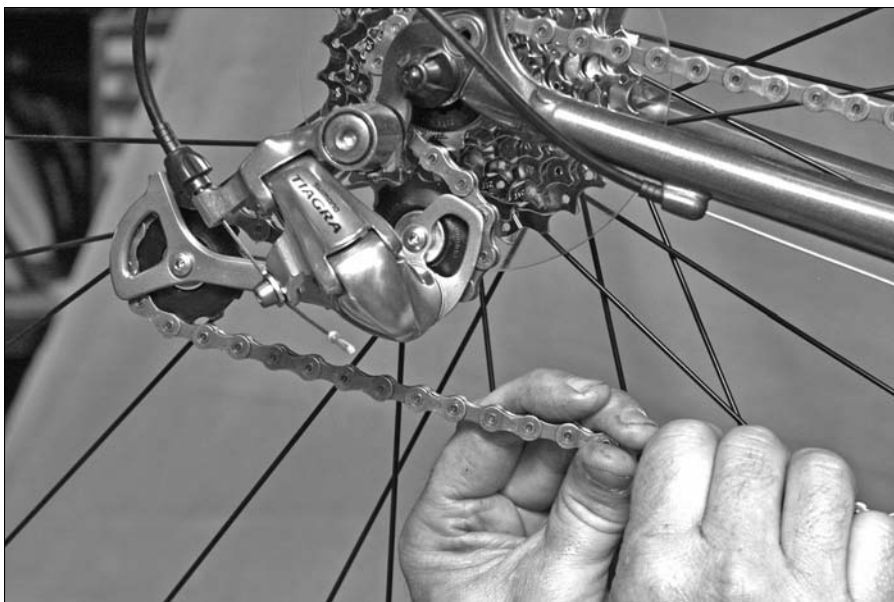
Figure 10-12: Measuring the chain
