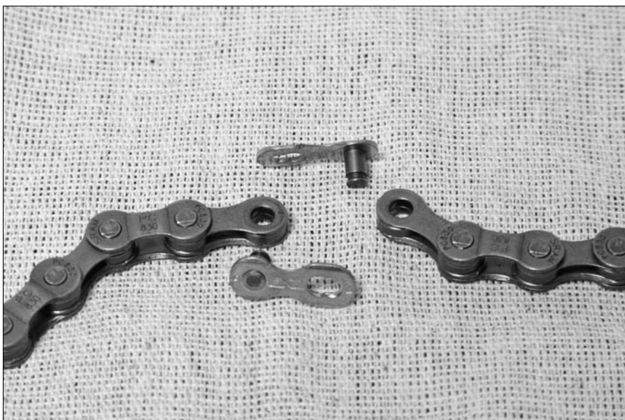
Figure 10-1: An SRAM PowerLink chain.
