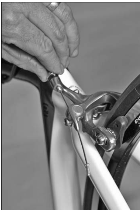
Figure 8-16: Adjusting the cable on center- mount brakes.
