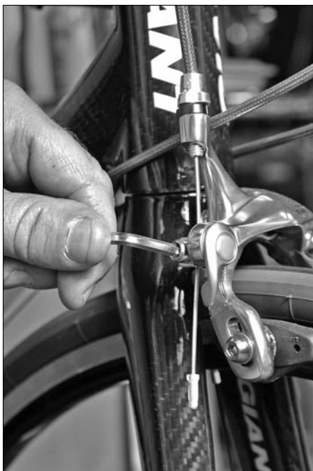
Figure 8-15: Adjusting center- mount brakes.
