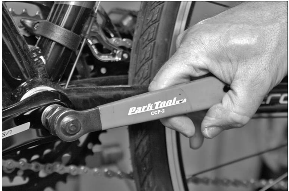
Figure 13-8: Using the crank-arm extractor.
