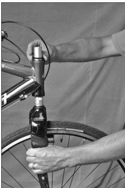
Figure 15-15: Removing the fork.
