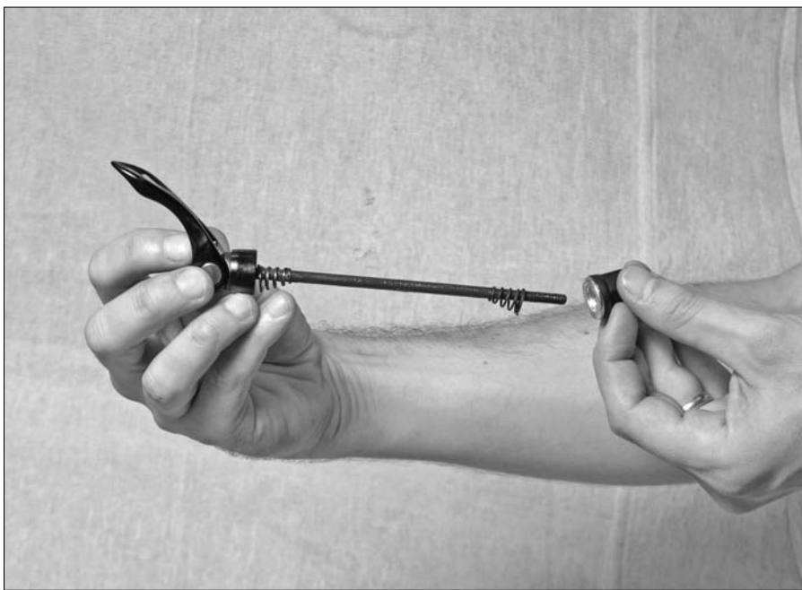
Figure 7-3: The quick- release skewer.
