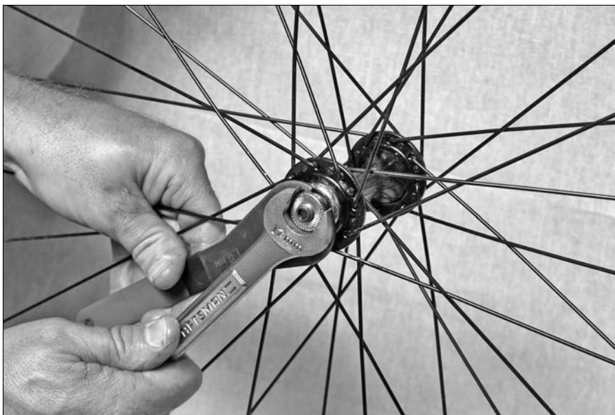
Figure 7-11: Tightening the cones.
