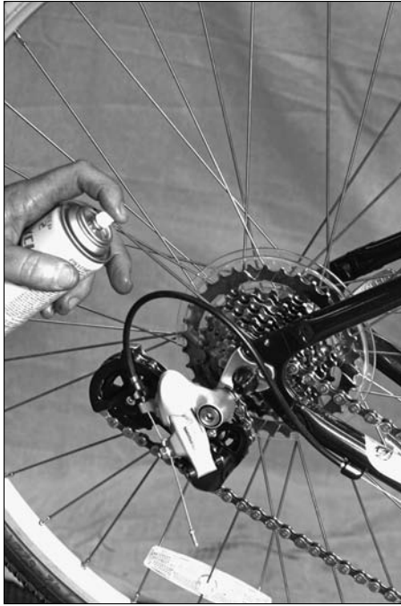
Figure 16-2: Degreasing various parts of a bike.
