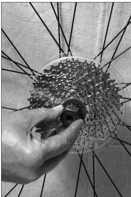
Figure 11-3: Inserting the freewheel remover tool into the center of the cassette.
