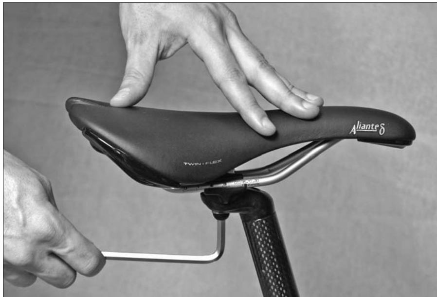
Figure 9-8: Adjusting the saddle
