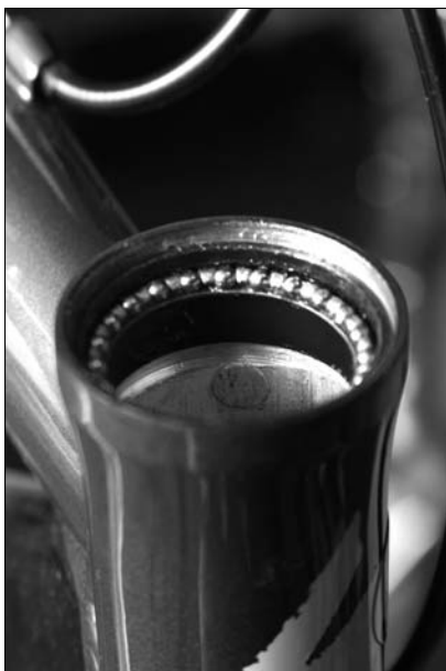
Figure 15-16: Bearings in the headset.
