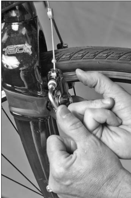
Figure 8-12: Adjusting the brake.
