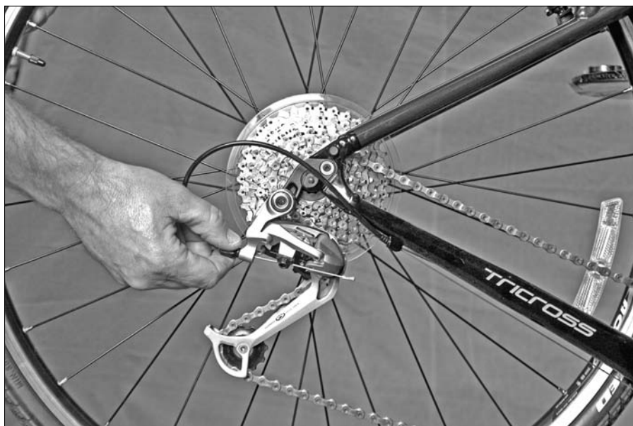
Figure 14-10: The barrel adjuster.
