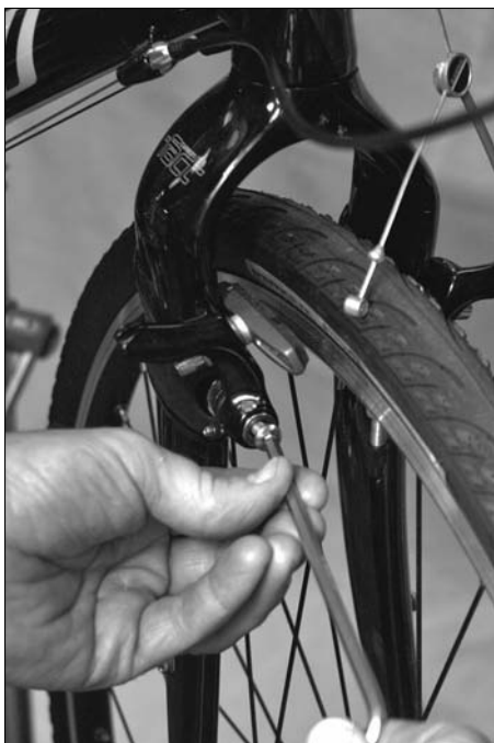
Figure 8-7: Loosening the brake.
