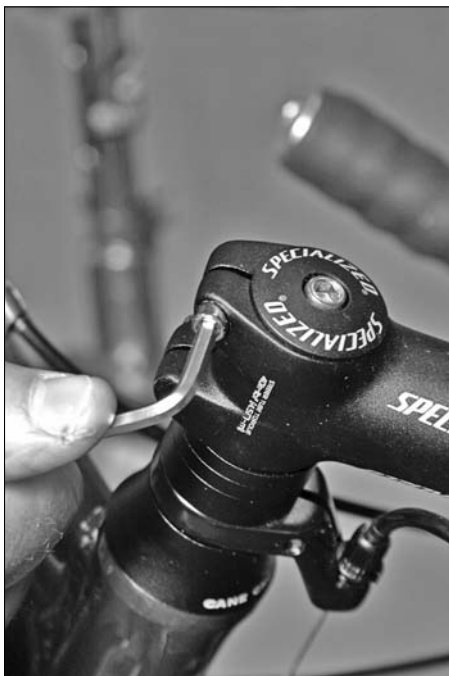
Figure 15-12: Undoing the clamp bolt.
