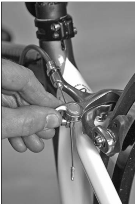
Figure 8-14: Moving the lever on center- mount brakes
