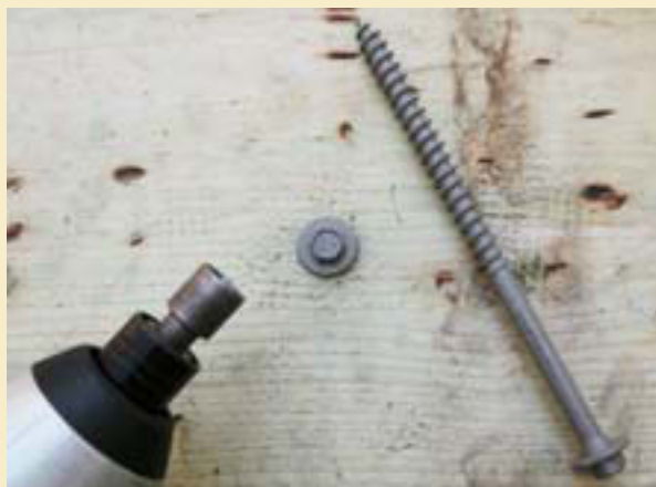
Self-tapping ledger screws do not require pilot holes or washers and have low-profile heads so they do not interfere with joist hanger installation.
