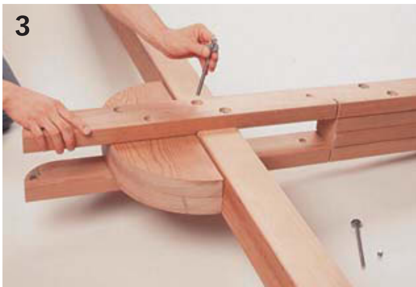
Fasten the post, rails, and braces with lag bolts. Drill counterbores for the bolt heads and the nuts.
