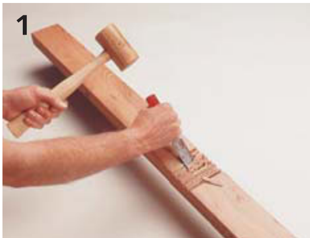
Cut a mortise into each side rail by making a series of ¼"-deep kerf cuts and then removing the waste wood with a mallet and chisel.
