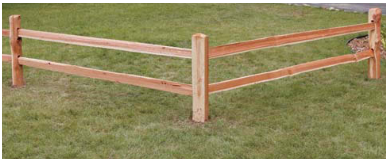
A split rail fence looks great as a garden backdrop or a friendly boundary line. The rough-hewn texture and traditional wood joints are reminiscent of homesteaders' fences built from lumber cut and dressed right on the property.
