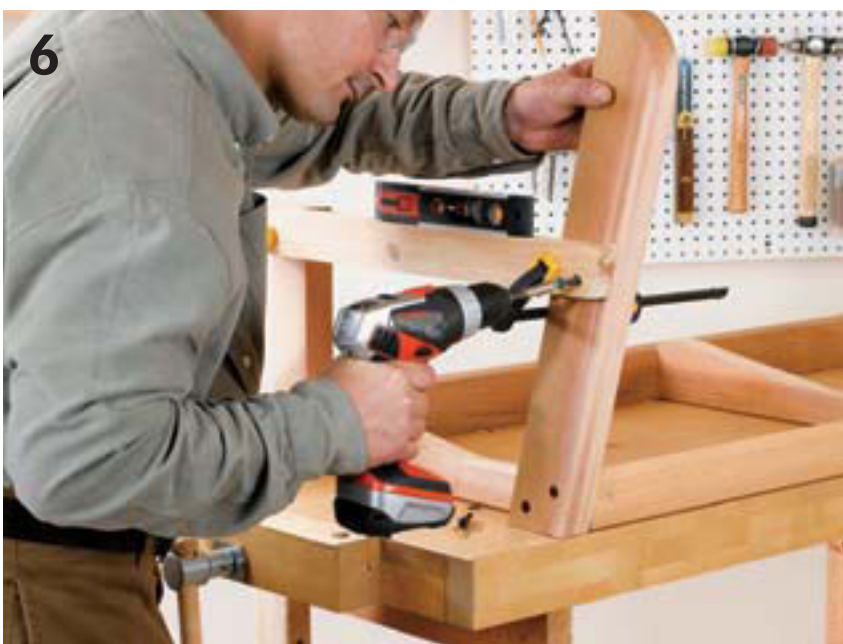
Attach the arm supports. Drive two 2½" deck screws through each end of the arm supports and into the front and back posts. Then attach the arm front with two 2½" deck screws.
