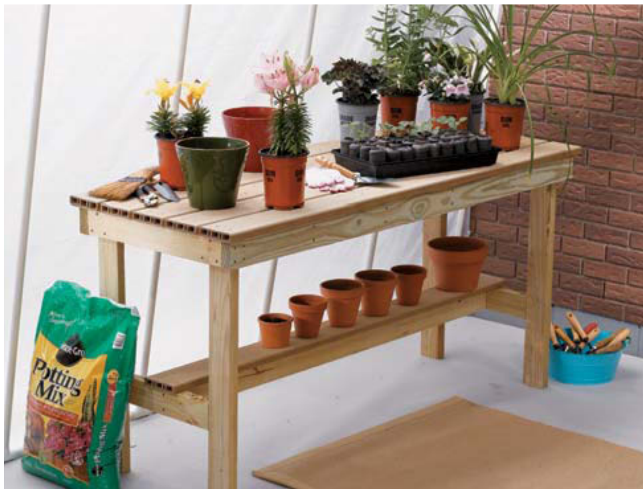
This potting bench has a 28 × 71" top and is built with four 2 × 4s and three standard-size decking boards. The handy pot shelf below the bench top is made with a cutoff from one of the deck boards.
