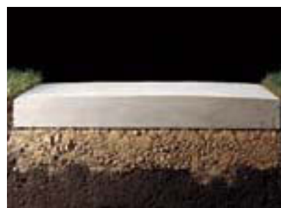
Walkways should crown in the center to provide water runoff.
