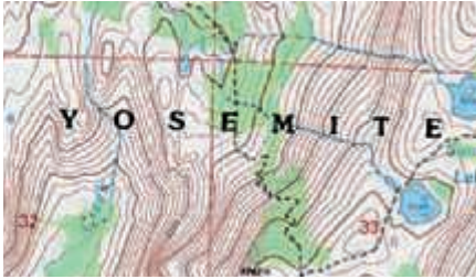
FIGURE 14.26 Contours within Yosemite National Park in California show streams, which follow paths of steepest descent, running perpendicular to the contours. (Source: Yosemite National Park Map from U.S. Geological Survey, http://www.usgs.gov )
