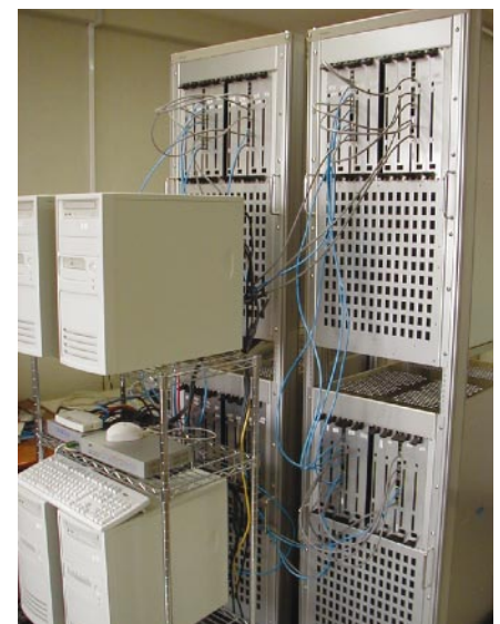
Starring role: a GRAPE-6 machine (above), custom-built to model globular clusters (left).
