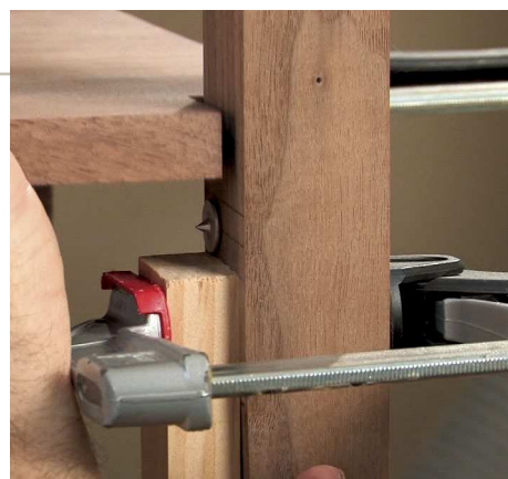
Locate the shelf. A support block clamped to the leg holds the shelf in place.
