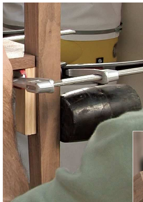
Tap once. A light mallet tap drives the dowel center into the shelf edge (left). The dimple (below) locates the drill bit for a perfectly aligned hole.
