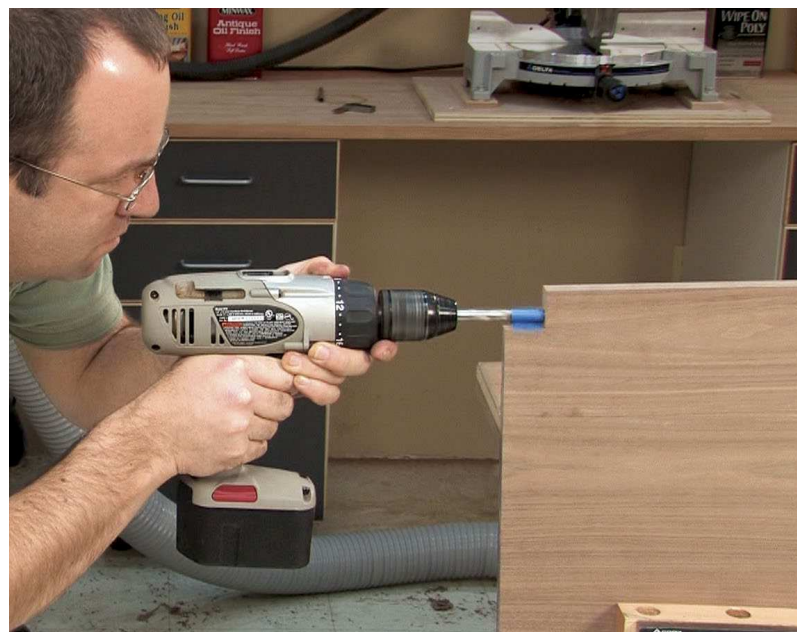
Drill the shelf edge. Eyeball the drill and the edge of the shelf to make sure the hole is straight and square.
