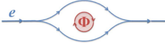
Fig. 5 An electron is circulating around a confined magnetic flow \Phi . Although the magnetic field is zero along the path, the vector potential is non-zero. Therefore, the wave packet acquires a relative phase
