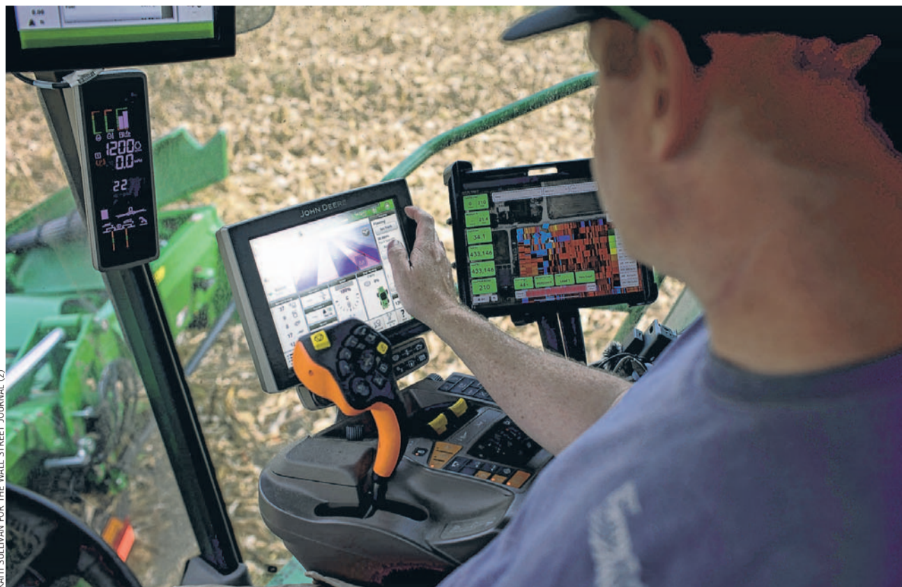
Indiana farmer Brian Scott has been using a Precision Planting upgrade on his Deere planter since 2019 to meter out seeds on his 2,500-acre farm. This spring, he updated the planter's capabilities to close the trench it digs in the soil to plant seeds.
