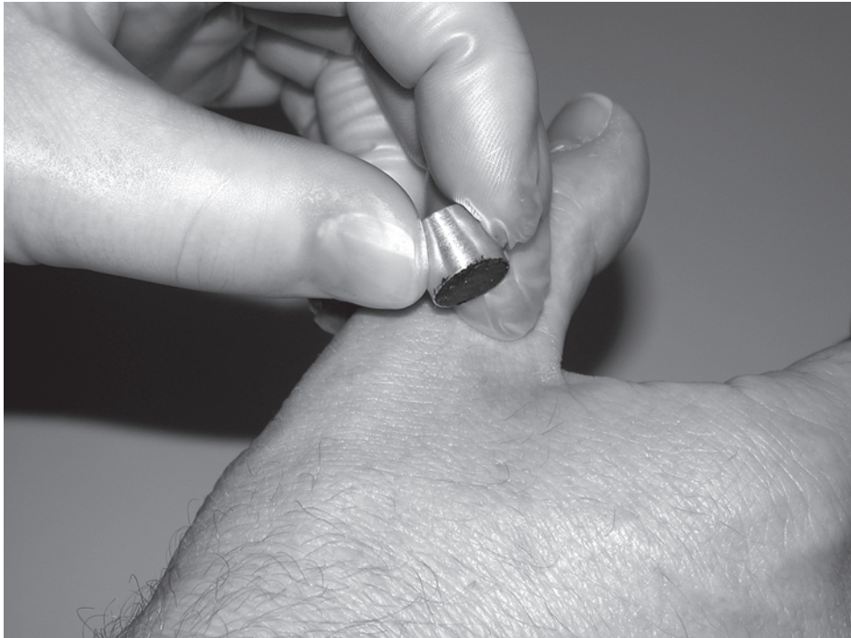
Figure 9.11 The use of an aluminium stub that is topped with a sticky, electrically conducting tab to collect gunshot residues
