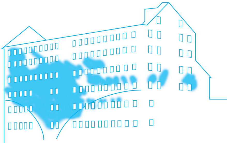
Figure 10.5 V-shaped smoke damage evident when a burnt building is viewed as a whole from the outside
