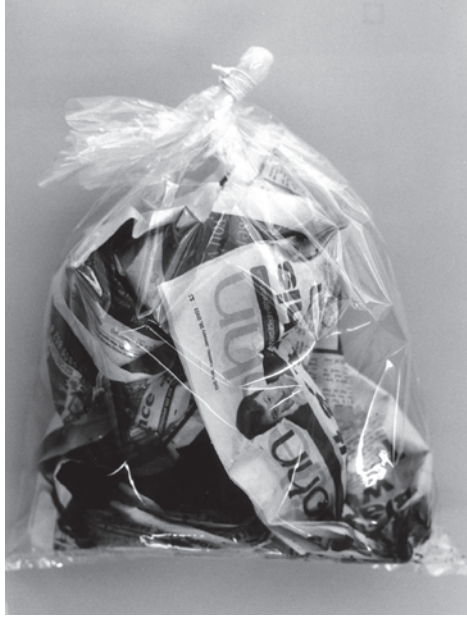
Figure 2.12 A nylon bag closed with an airtight swan-neck seal
