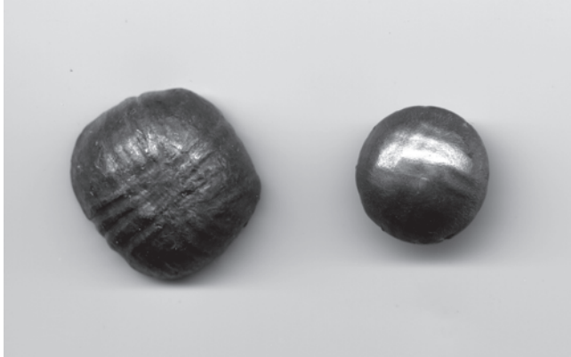
Figure 9.8 Weave pattern on the noses of two bullets
