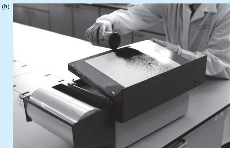
(a) Charging the film using the corona and (b) applying the photocopy toner powder
