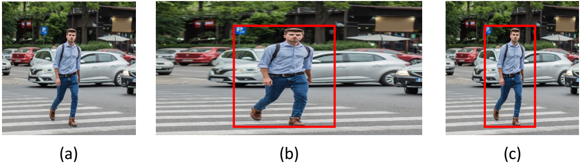
Figure 10.24 Illustration of the detection and localization of objects at multiple scales and aspect ratios using a fixed input window. The original image (a) is replicated multiple times and each copy is scaled in the horizontal and/or vertical directions, as illustrated for a horizontal scaling in (b). A fixed-sized window is then scanned over the scaled images. When an object is detected with high probability, as illustrated by the red box in (b), the corresponding window coordinates can be projected back into the original image space to determine the corresponding bounding box as shown in (c).
