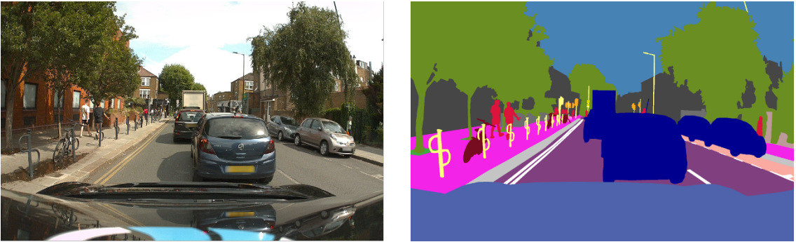
Figure 10.26 Example of an image and its corresponding semantic segmentation in which each pixel is coloured according to its class. For example, blue pixels correspond to the class ‘car’, red pixels to the class ‘pedestrian’, and orange pixels to the class ‘traffic light’. [Courtesy of Wayve Technologies Ltd.]
