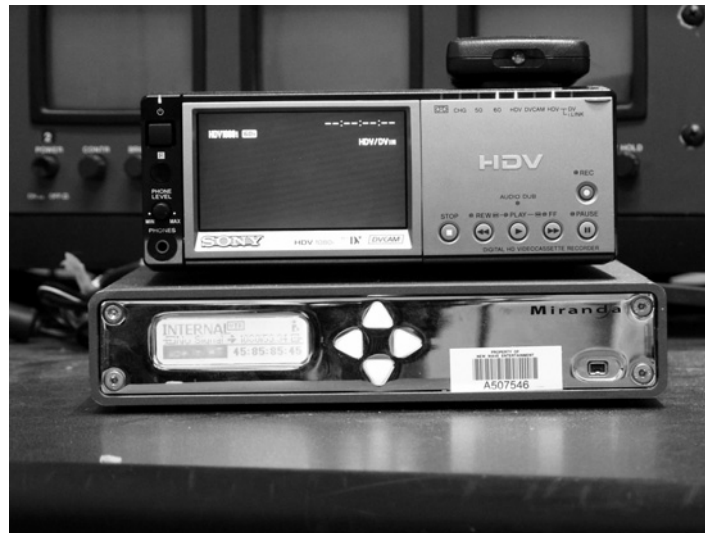
Figure 5.3 The Sony HDV with a Miranda HDV to HSD-SDI converter. Although this combination converts the MPEG-2 HDV images to HD, it requires much more storage than importing and editing HDV natively in MPEG-2.
