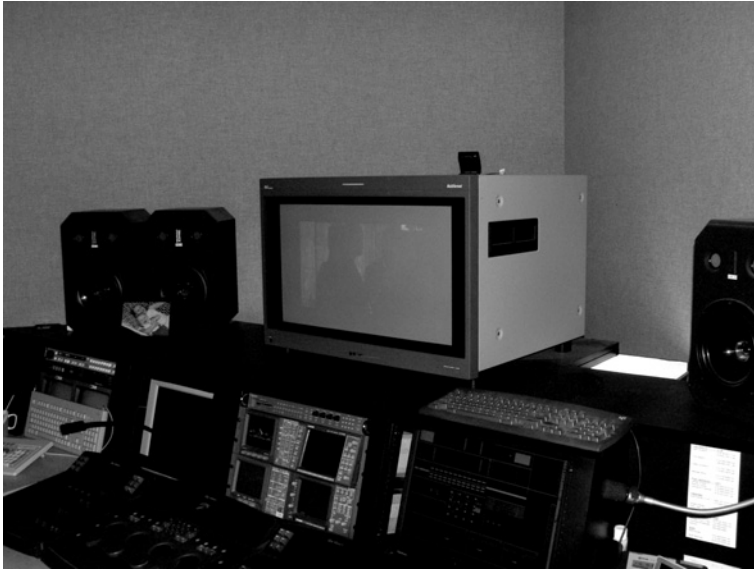
Figure 7.2 CRT monitor. The heavy, interlaced, and often calibrated CRT monitor is slowly being replaced by flat screen monitors.
