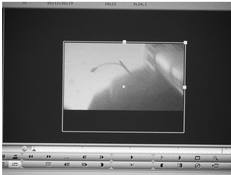
Figure 2.4 Adjusting 4 × 3 in 16 × 9 space. When placing a 4 × 3 standard definition image in a 16 × 9 HD frame, the bottom of the frame is the part usually eliminated.
