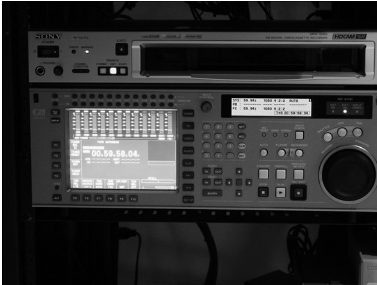
Figure 2.8 HDCAM SR. The HDCAM SR has become one of the standard studio HD recorders.
