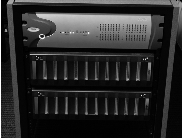
Figure 2.6 The storage requirement for HD is much larger than that of SD. This is a photo of two rows of local RAID array on top of the hardware for a Symphony Nitris HD editing system.
