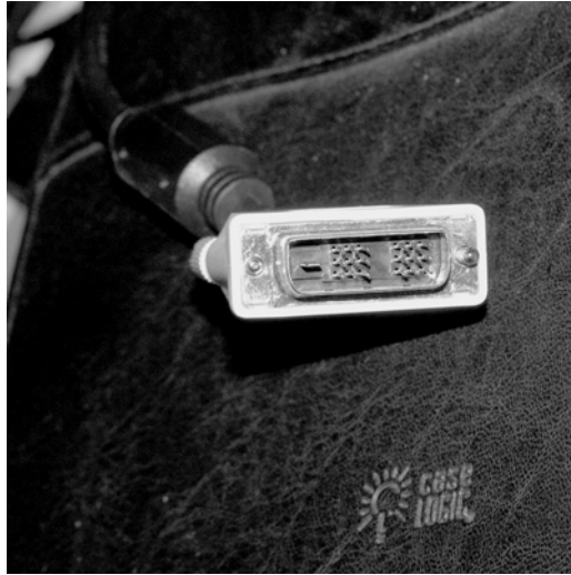
Figure A-4 This digital-only connector is a common connector for desktop monitors.
