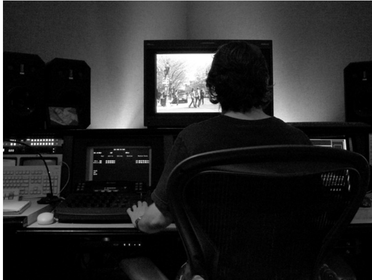
Figure 6.10 Color correction bay. The art of color correction is often given to professionals with sophisticated equipment, specifically designed for this purpose. The textless program is recorded to tape, and then in a tape to tape process a new color corrected master is created. This media is loaded back into the nonlinear editor and texted.
