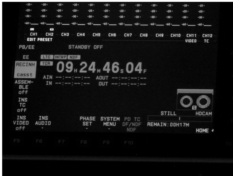
Figure 7.3 HDCAM SR time code. Just to the right of the “System Menu” is the time code display on an HDCAM SR. Converting 23.98 to 29.97, the deck can play out either drop or non-drop time code. This can cause problems if the wrong setting is selected.
