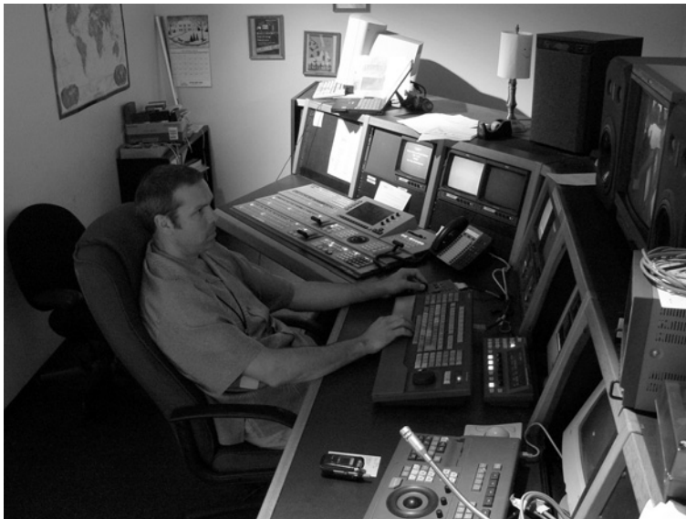
Figure 4.6 The linear bay of old still gets use as a dubbing and shot pull edit system. In a few cases, even for high definition, linear edit systems can be efficient.
