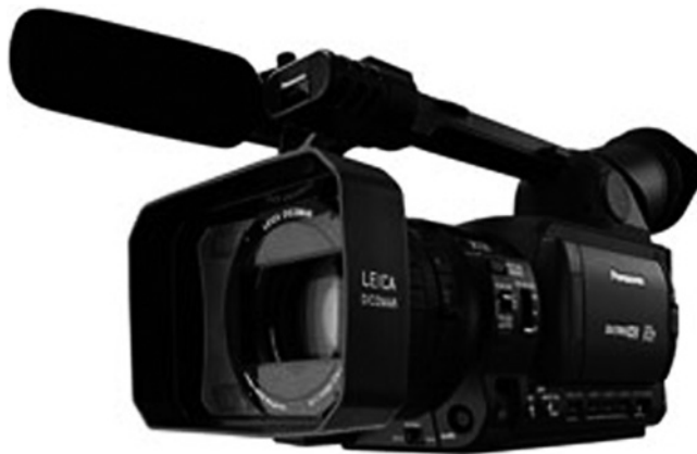
Figure 3.7 Panasonic's AG-HVX200 has garnered a great deal of interest. It stores images and sound to solid state media.
