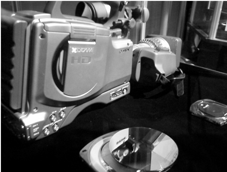
Figure 1.4 Sony's XDCAM HD. This camera, introduced in 2006, records its data to an optical disk. Not only does it record the HD image, it also records a smaller copy of the footage, called a proxy, that can be used for creative editing. When the program is finished, the full size information is recaptured for the finished product, avoiding having to capture the entire amount of footage at full resolution.
