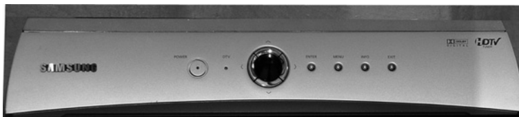
Figure 3.3 HD decoder. This is a Samsung HD over-the-air decoder. It has a standard definition output, and two frame size outputs, 720 and 1080. This is only used for DTV reception. For cable or satellite HD conversions, there are different conversion boxes.
