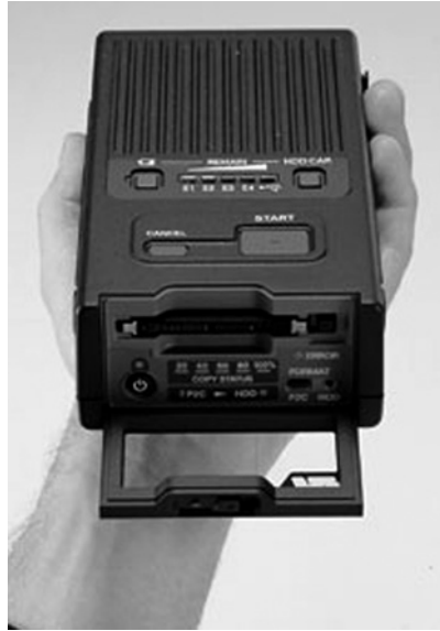
Figure 5.5 DVCPRO P2 Store Drive. This device is designed to offload media from the Panasonic P2 PIMCA card. (Photo courtesy of Panasonic Electronics.)
