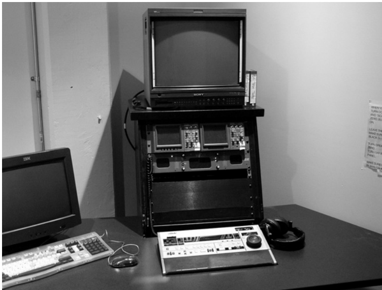
Figure 4.7 The quality control room is where the final edited video is examined frame by frame. Before a program is sent out, it is usually examined from start to finish to make sure everything is perfect from a technical perspective.
