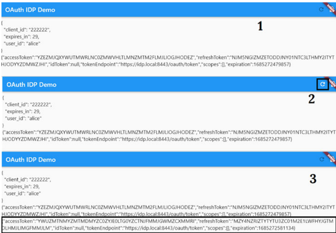
Figure 5.16: Refreshing the access token from the PKCE client
