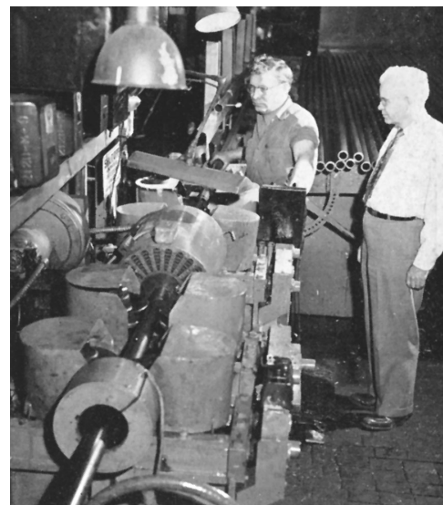
FIGURE 8. Cecil Farrow (right) watches operation of system for electromagnetic testing of longitudinally welded steel tubes.
