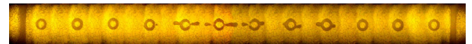
FIGURE 57. Mosaic image of upper row of rivets spaced 25 mm (1.0 in.) apart and associated with aluminum aircraft lap joint in Fig. 56. Numerous radial surface breaking fatigue cracks are visible. Eddy current frequency was 200 kHz.
