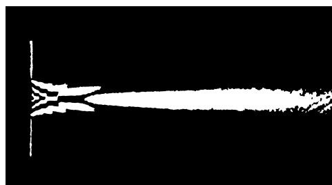
FIGURE 10. Acoustic model of radiation pattern, showing near field and far field. Source is at left, with energy propagating from left to right. Photograph shows acoustic waves propagating in illuminated liquid (schlieren technique). 53
