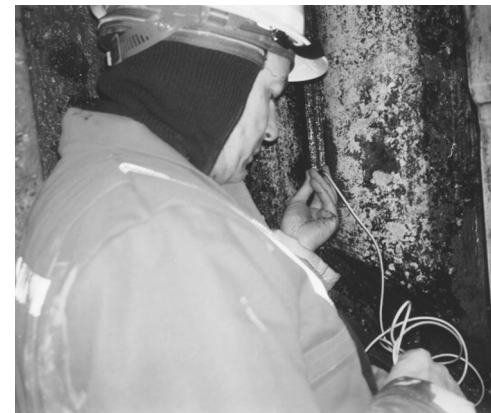
FIGURE 18. Eddy current testing of welds in marine environment: (a) eddy current scanning through coatings and on damp surfaces; (b) magnetic particle testing verifies eddy current results (arrows point to magnetic particle indication).
