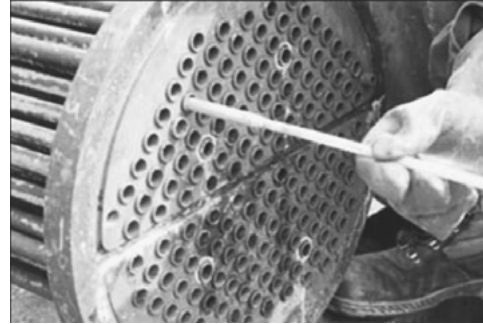
FIGURE 3. Magnetic flux leakage probe inserted in carbon steel tube bundle of crude petroleum processing unit.
