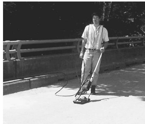
FIGURE 8. Hand held ground penetrating radar instrument in use on bridge deck.
