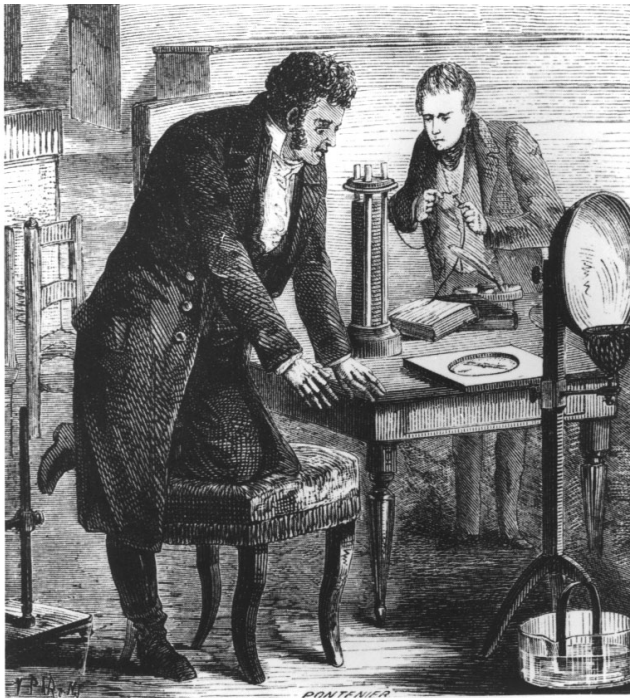
FIGURE 2. Hans Christian Ørsted: (a) with students Ørsted discovers electric current’s magnetic effect on compass when circuit is completed; (b) Ørsted’s observation that compass needle near electric current moves to position perpendicular to direction of current.
