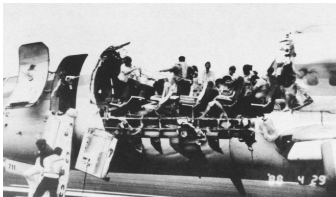
FIGURE 1. Fatigue cracks contributed to damage to aircraft fuselage in flight (April 1988).
