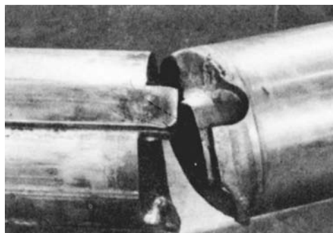
FIGURE 15. Shaft fractured at keyway.
