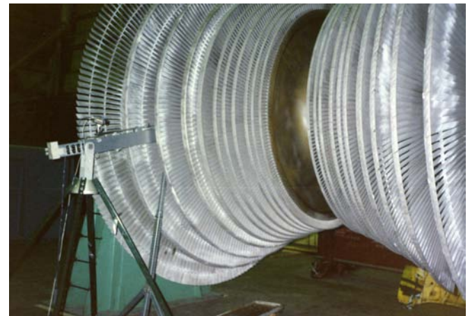
FIGURE 13. Inspection turbine disk blade attachment areas. Turbine placed on rollers rotates while test data are acquired.
