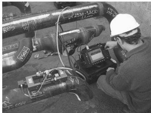
FIGURE 49. Typical semiautomated handscanner for piping test.
