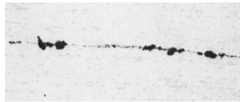
FIGURE 9. Oxide layer with entrapped refractory inclusions in rolled aluminum.
