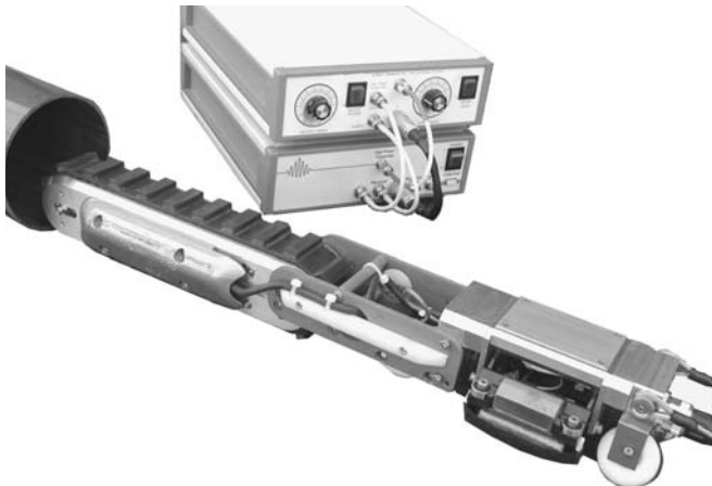
FIGURE 78. Small tractor motor pulls electromagnetic acoustic transducer test probe into small diameter pipe. Guided waves propagate around circumference to inspect pipe wall.
