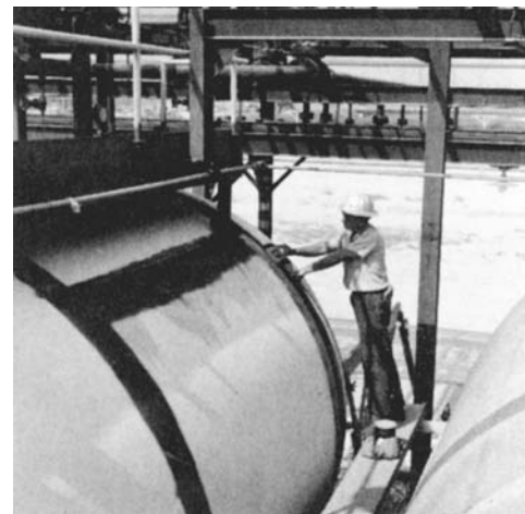
FIGURE 16. Ultrasonic tests in progress on heavy wall vessels: (a) in-service pressure vessel weld test; (b) preservice pressure vessel weld test.
