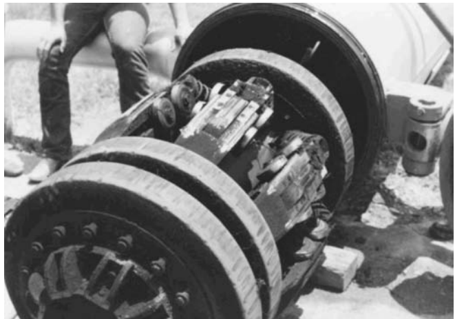
FIGURE 77. Pipe and tube testing with electromagnetic acoustic transduction.
