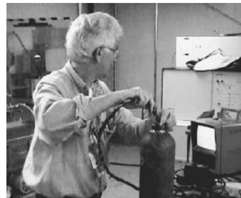
FIGURE 4. Visual test using a borescope to view the interior of a cylinder.
