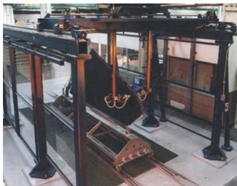
FIGURE 5. Example of overhead gantry water squirter through-transmission and pulse echo system for large composite objects.
