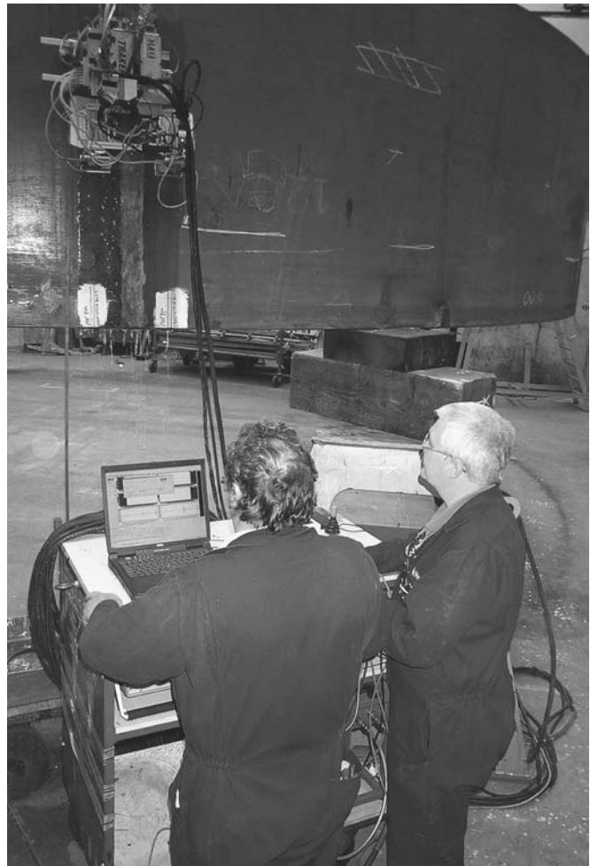
FIGURE 57. Magnetic wheel tracker performing contact phased array weld test.
