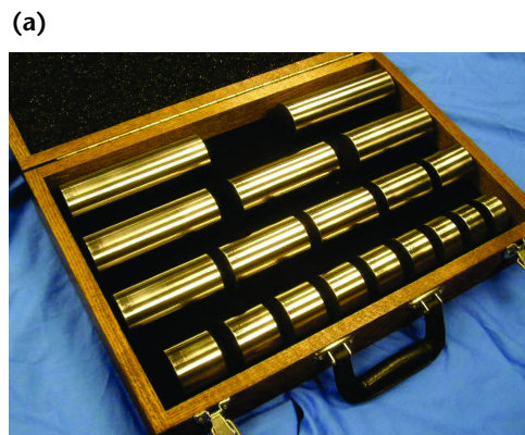
FIGURE 12. Flat bottom hole blocks for ultrasonic calibration: (a) set of 19 steel blocks; (b) diagram.
