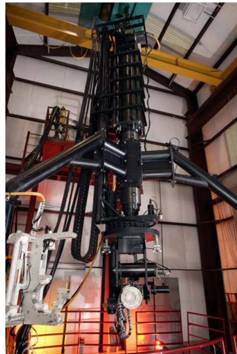
FIGURE 1. Ultrasonic system for testing of pressurized water reactor welds — welds of vessel seams, of flange to shell, of nozzle to shell, of nozzle to piping, of shell to lower head welds, of meridian (on lower head) and of nozzle inner radius. Unit on left is used to dock the module containing pulser preamps and transducers to change these units quickly without removing device from vessel.
