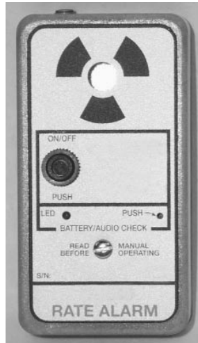
FIGURE 4. Gamma and X-radiation sensing devices incorporating geiger-müller tubes: (a) survey meter for range selectable from 0 to 20 mSv·h -1 (0 to 2 R·h -1 ) and automatic aural alarm over 2.5 mSv·h -1 (250 mR·h -1 ); (b) survey meter with on/off switch for aural monitoring; (c) for high noise areas, personal rate alarm with flashing light and optional earplug for aural alarm; (d) area monitor with standard 20 μSv·h -1 (2 mR·h -1 ) trip point, audio piezo alert and large red strobe warning light; (e) visual alarm for gamma and X-rays from 80 keV to 1.5 MeV and adjustable alarm threshold.
