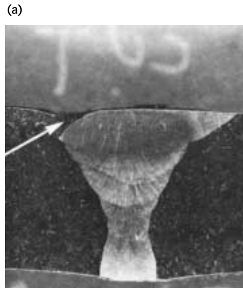
FIGURE 30. Undercut on outside diameter: (a) photomacrograph at 4.6 \times ; (b) radiographic image at 1 \times .
