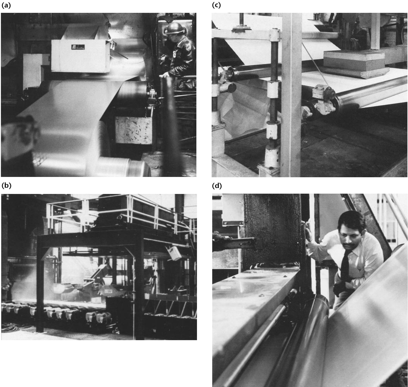
FIGURE 2. Automated applications of X-ray density gaging: (a) measurement of thickness of coiled stainless steel; (b) measurement of thickness of hot strip steel; (c) measurement of moisture content of paper at paper mill; (d) measurement of packaging tape after application of adhesive coating. 14
