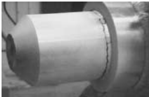
FIGURE 5. Liquid penetrant indication of cracking.
