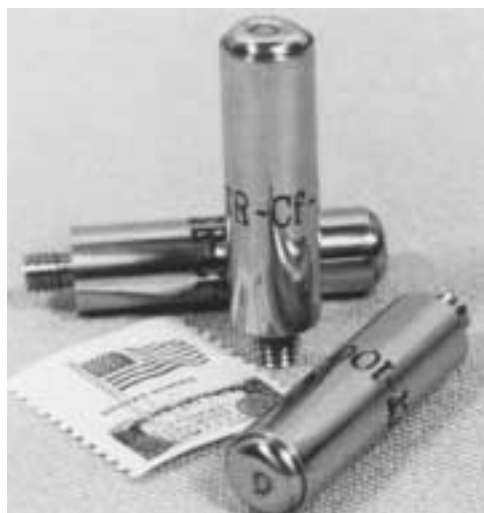
FIGURE 10. Californium-252 sources compared in size to postage stamp.
