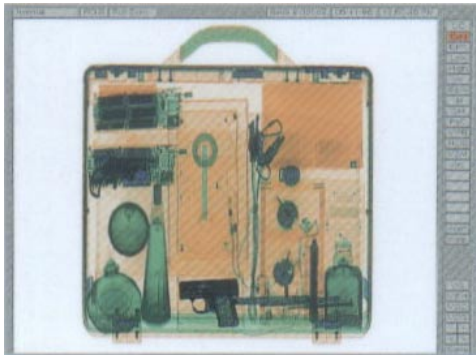
FIGURE 17. Radioscopic image of suitcase contents: (a) detailed image; (b) image thresholded to view items of greatest density.
