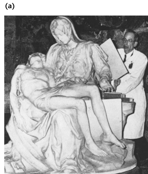
FIGURE 29. Michelangelo Buonarroti's Pietà , Saint Peter's Basilica, Vatican: (a) film cassette placement; (b) image of hand, showing pins used to repair broken fingers. 96
