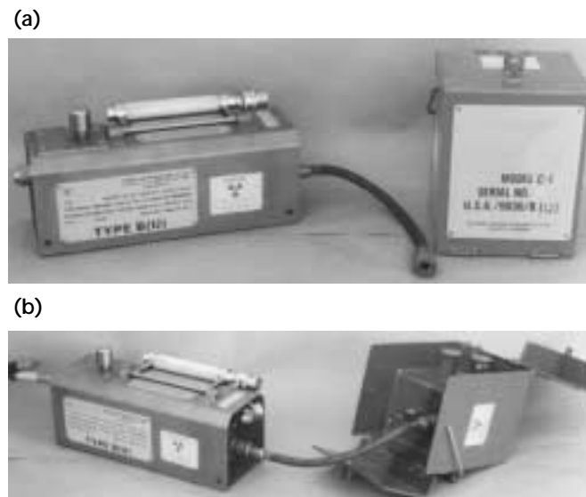
FIGURE 14. Exposure device with source exchanger: (a) exchanger (left) closed, exposure device fitted with short exchange tube; (b) exchanger open and attached, ready for source transfer to exchanger (note source pigtail in storage position, on the left).
