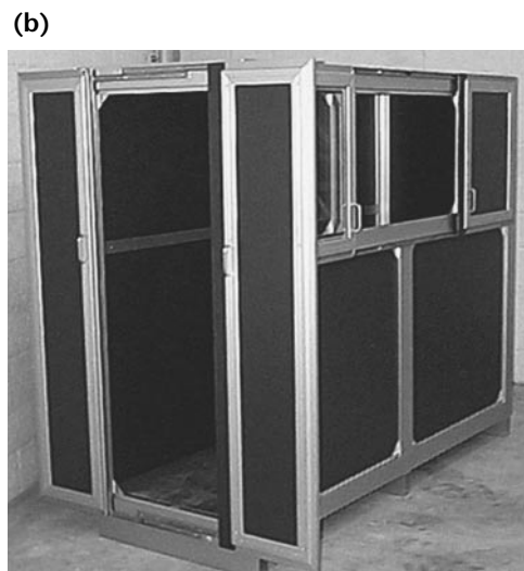
FIGURE 7. Shielding above radiation source reduces radiation reflected from atmosphere. Such radiation is called skyshine. 28
