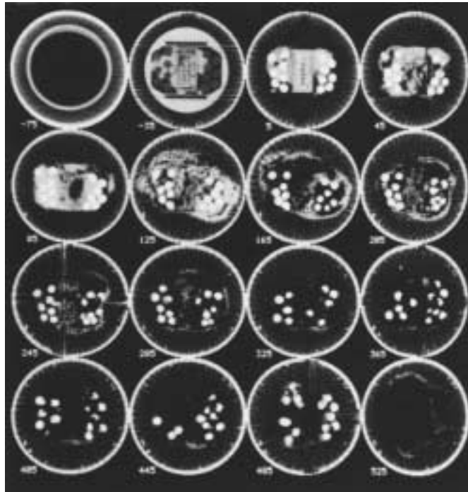
FIGURE 29. Typical slice images from last fuel assembly tested: (a) array of 16 images of rod cross sections at resolution of 128 \times 128 pixels; (b) magnification by interpolation of one cross section image to 128 \times 128 pixels. 32 Interpolation does not improve genuine resolution but avoids pixelization of image.
