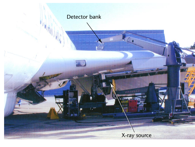
FIGURE 14. Setup for inspection of wing structure.
