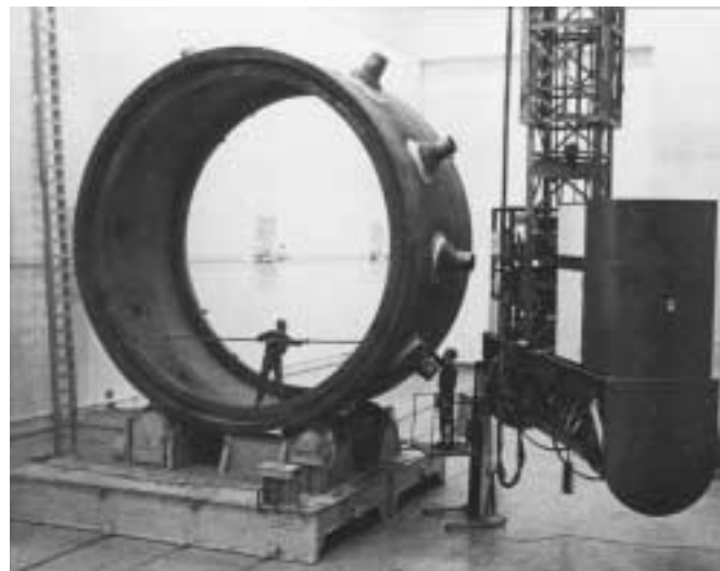
FIGURE 18. Placing film and aligning 13 MeV linear accelerator beam for examination of boiling water reactor nozzle weld. 20
