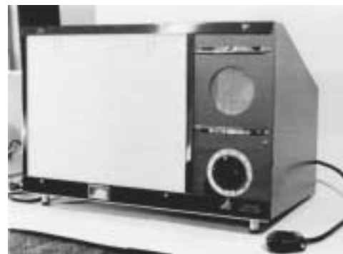
FIGURE 5. High intensity combination illuminator with iris diaphragm spot viewer and large viewer.
