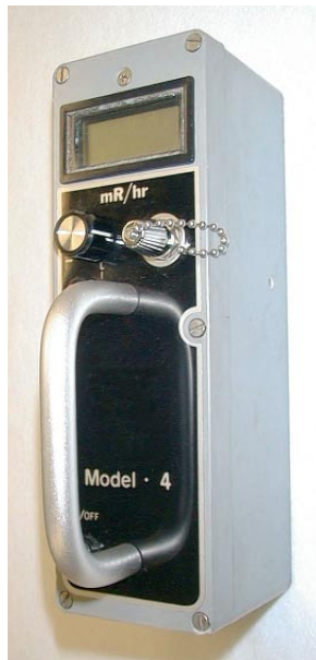
FIGURE 4. Gamma and X-radiation sensing devices incorporating geiger-müller tubes: (a) survey meter for range selectable from 0 to 20 mSv·h -1 (0 to 2 R·h -1 ) and automatic aural alarm over 2.5 mSv·h -1 (250 mR·h -1 ); (b) survey meter with on/off switch for aural monitoring; (c) for high noise areas, personal rate alarm with flashing light and optional earplug for aural alarm; (d) area monitor with standard 20 μSv·h -1 (2 mR·h -1 ) trip point, audio piezo alert and large red strobe warning light; (e) visual alarm for gamma and X-rays from 80 keV to 1.5 MeV and adjustable alarm threshold.
