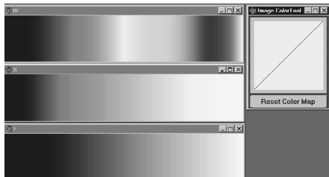
FIGURE 4. Linear lookup table with gamma = 1.0 applied to image (valued 0 to 255) for three different color maps.
