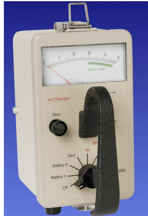
FIGURE 1. Radiation survey meter incorporates air filled ionization chamber vented to atmosphere, with five selectable linear ranges: 0 to 50 \mu\text{Sv}\cdot\text{h}^{-1} (0 to 5 \text{mR}\cdot\text{h}^{-1} ), 0 to 500 \mu\text{Sv}\cdot\text{h}^{-1} (0 to 50 \text{mR}\cdot\text{h}^{-1} ), 0 to 5 \text{mSv}\cdot\text{h}^{-1} (0 to 500 \text{mR}\cdot\text{h}^{-1} ), 0 to 50 \text{mSv}\cdot\text{h}^{-1} (0 to 5 \text{R}\cdot\text{h}^{-1} ), 0 to 500 \text{mSv}\cdot\text{h}^{-1} (0 to 50 \text{R}\cdot\text{h}^{-1} ).
