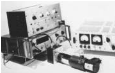
FIGURE 24. Gaging system for direct readout process monitor for carbon coating thickness on nuclear fuel microspheres. 27
