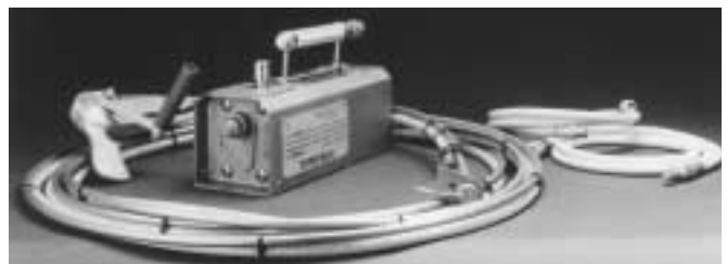
FIGURE 11. Exposure device with crankout and guide tube.
