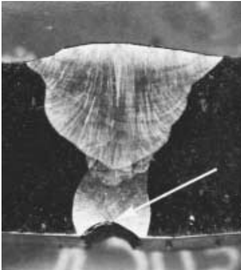
FIGURE 33. Concave root surface: (a) photomacrograph at 4.3 \times ; (b) radiographic image at 1.2 \times .
