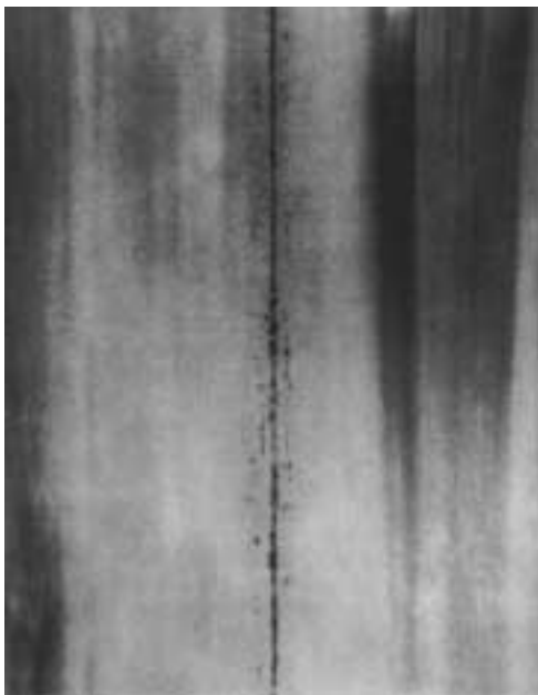
FIGURE 18. Streaking caused by inadequately cleaned film hangers.
