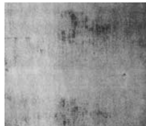
FIGURE 23. Pressure marks caused by foreign matter on rollers or improper roller clearance.
