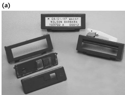
FIGURE 2. Clip-on personal radiation dosimeters: (a) film badges; (b) thermoluminescent dosimeters (TLDs). 21
