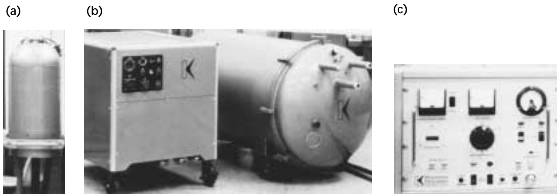
FIGURE 9. Components of mobile deuterium tritium neutron radiographic system: (a) deuterium tritium source head, typically on 6 m (20 ft) cables; (b) cooling unit (left) and power supply; (c) control unit.
