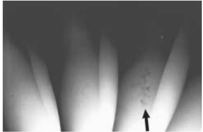
FIGURE 6. Sponge shrinkage in 13 mm (0.5 in.) aluminum casting.
