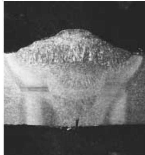
FIGURE 28. Incomplete or inadequate penetration: (a) photomacrograph; (b) radiographic image.
