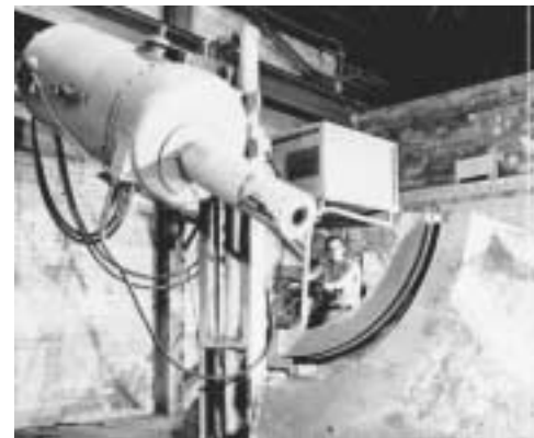
FIGURE 18. Van de graaff 2.5 MeV electrostatic generator.
