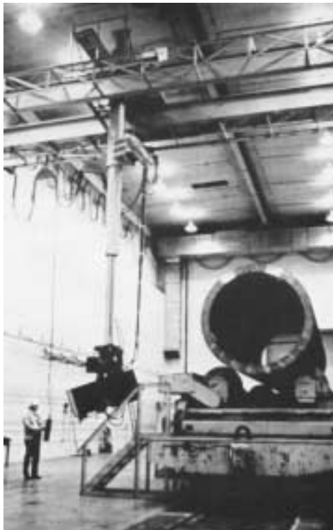
FIGURE 19. Radiographic examination of pressure vessel welds is conducted with 7.5 MeV linear accelerator. 20
