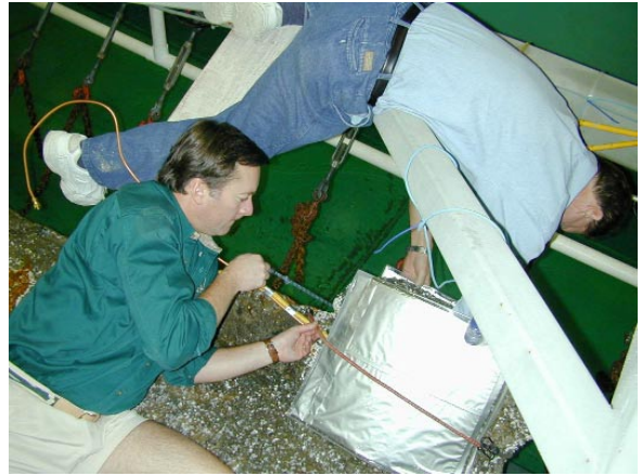
FIGURE 26. Radiography of submarine Hunley : (a) positioning a radiosopic image plate on hull exterior; (b) computed radiograph of hull's rivets (the vessel was riveted from the inside and sanded to improve its hydrodynamics); (c) setting up exposure of iridium-192. 91
