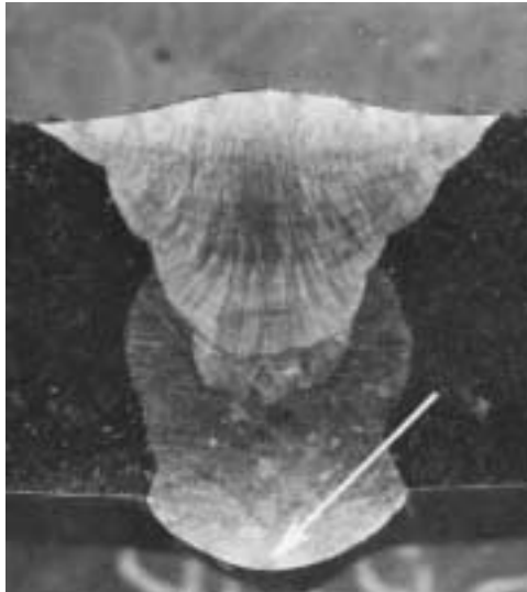
FIGURE 31. Excessive penetration: (a) photomacrograph at 4.5 \times ; (b) radiographic image at 1.2 \times .
