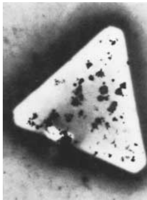
FIGURE 2. Localized silver in printout image. This is a T grain, a form used with soft intensifying screens.
