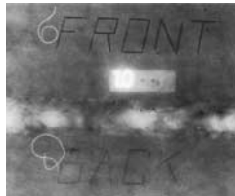
FIGURE 16. Words front and back scratched in the surface of front and back lead foil screens before radiography of a 25 mm (1.0 in.) welded steel plate. Hairs placed between respective screens and film are visible as light marks preceding inscribed words.
