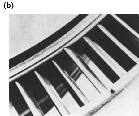
FIGURE 22. Case-to-ablative bond discontinuities are revealed by radiopaque additive in adhesive: (a) first image; (b) closer image.
