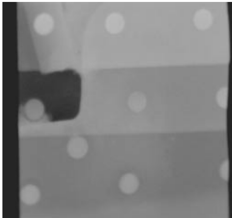
FIGURE 15. Enhancement of corrosion data: (a) scaled radiographic image; (b) three-dimensional rendering from detector of reversed geometry, scanning source system.
