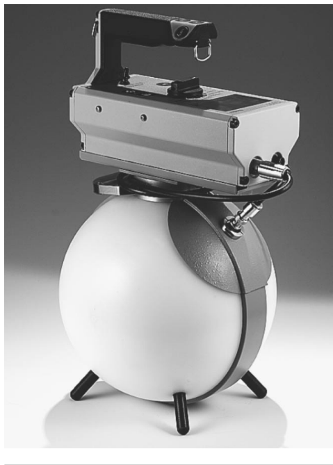
FIGURE 3. Boron trifluoride neutron radiation detector tube provides high gamma rejection up to about 5 \text{ Sv} \cdot \text{h}^{-1} ( 500 \text{ R} \cdot \text{h}^{-1} ) and detects neutrons with energies from thermal to about 10 MeV.
