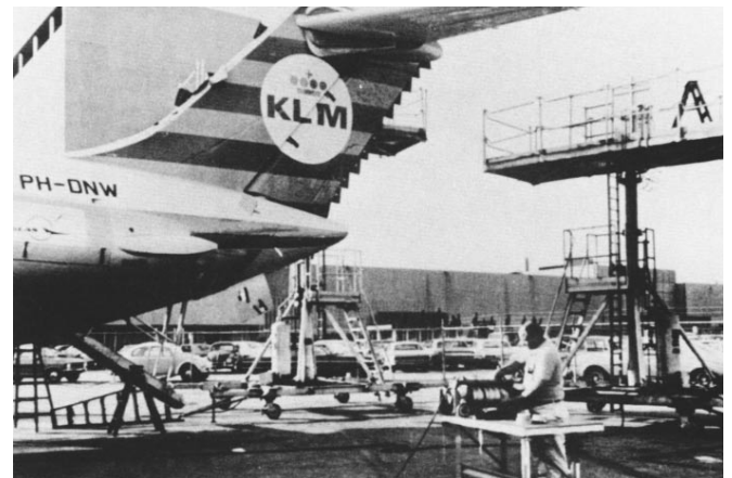
FIGURE 8. Position of X-ray source to expose maximum area of structure being radiographed.
