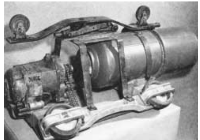
FIGURE 1. Internal pipeline X-ray generator and crawler device. 1
