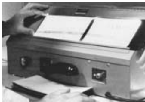
FIGURE 4. High intensity illuminator designed for viewing strip film.
