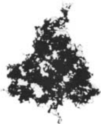
FIGURE 7. Electron micrograph of developed silver bromide grain.
