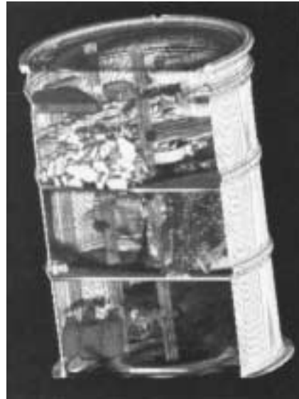
FIGURE 32. Volume rendered 100-slice display of 2 MeV transmission computed tomographic data taken from waste drum phantom. 34
