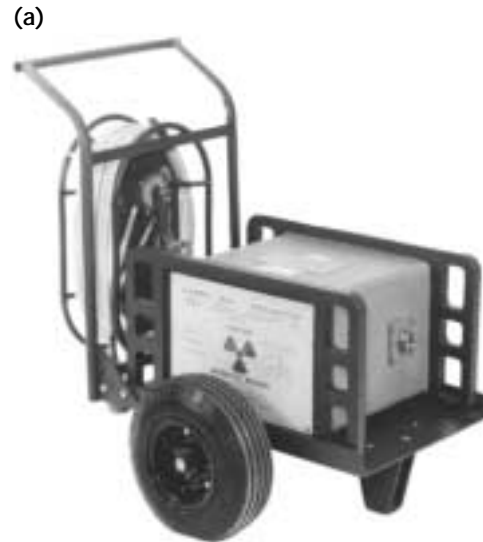
FIGURE 13. Photographs of two American National Standards Institute Type I cobalt-60 exposure devices: (a) on two-wheeled dolly, for up to 9.25 TBq (250 Ci) of cobalt-60; (b) on four-wheeled dolly.
