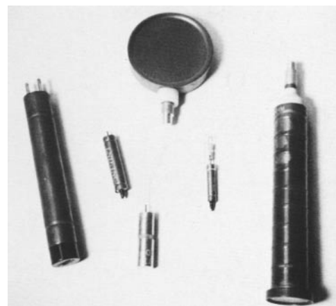
FIGURE 13. Assortment of geiger-müller counters demonstrating availability of sizes and shapes. Smallest counter shown is about 30 mm (1 in.) long.
