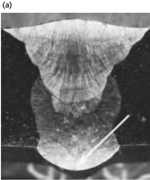
FIGURE 30. Drop-through: (a) photomicrograph at 4x; (b) radiograph at 1x. 29
