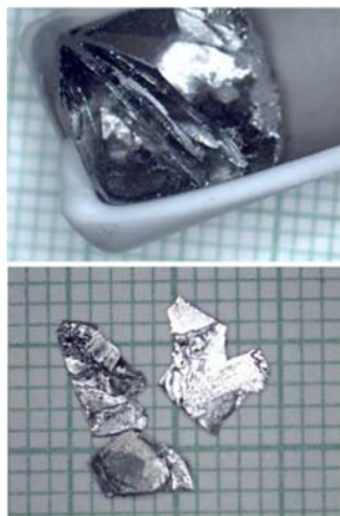
Fig. 12 (Top) Crucible limited growth of the \text{AlFe}_2\text{B}_2 . (Bottom) Plate-like crystals of \text{AlFe}_2\text{B}_2 . Reproduced from Lamichhane, T. N.; Xiang, L.; Lin, Q.; Pandey, T.; Parker, D. S.; Kim, T.-H.; Zhou, L.; Kramer, M. J.; Bud'ko, S. L.; Canfield, P. C., Magnetic Properties of Single Crystalline Itinerant Ferromagnet \text{AlFe}_2\text{B}_2 . Phys. Rev. Mater. 2018 , 2 (8), 084408, with permission of the APS Physics.
