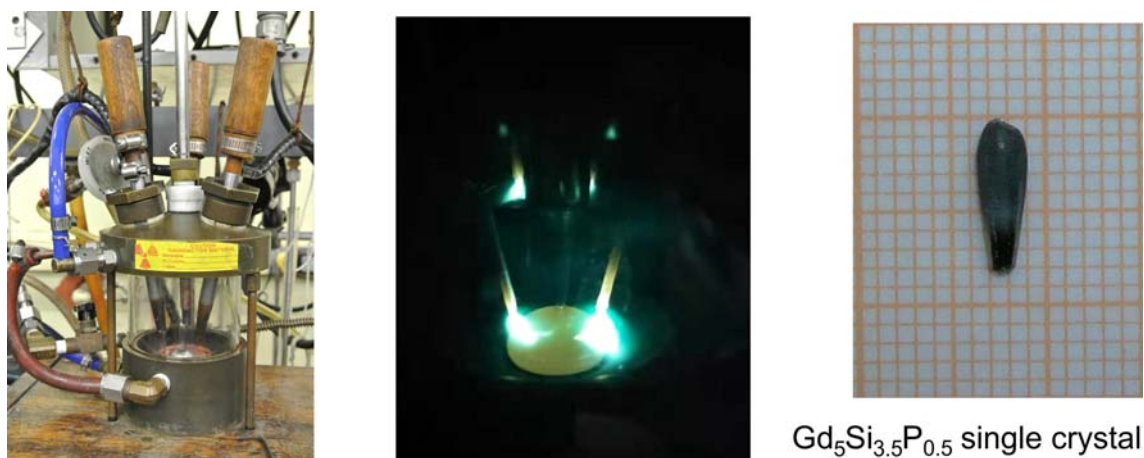
Fig. 10 (Left) Tri-arc furnace from the Centorr Vacuum Industries at the Brockhouse Institute for Materials Science, McMaster University, Hamilton, ON, Canada. (Middle) Crystal growth in progress; the sample is melted by three electrodes, and the pull rod is touching the molten sample. (Right) Crystal of the \text{Gd}_5\text{Si}_{3.5}\text{P}_{0.5} magnetocaloric material grown by the tri-arc method. The crystal facets are visible at the bottom of the crystal.
