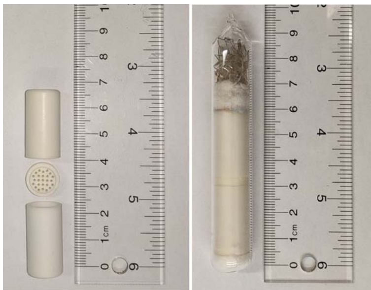
Fig. 11 (Left) Alumina crucibles with a frit disk in-between. (Right) Alumina crucibles are sealed inside a silica tube, with silica wool and broken silica pieces at the top. The sample and flux are in the lower crucible.
