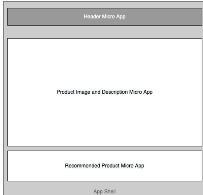
Figure 1.4 – Micro app architecture with product images and recommended products co-existing as different micro apps
