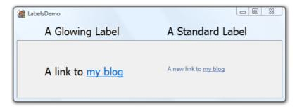
In the bottom area of the form above you can see two instances of the new LinkLabel component, a wrapper of the SysLink Windows class. This is a new control you can use only on Windows XP or later versions (not on Win-
