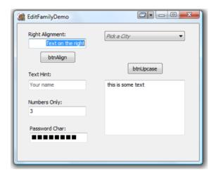
On the left side of the form you can see four edit boxes using some of the new features. The first has its text right aligned, the second displays a text hint, the third allows only numeric input, and the fourth uses Unicode CodePoint 25AO (Black Square) as its password character. (It is nice that you can use any Unicode symbol for the password character.)
