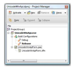
You can see there is a new Build Configurations node, with sub nodes, used to activate a build configuration in a much simpler way than in Delphi 2007. This topic is covered in the later section "Build Configurations and Configuration Settings".
