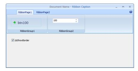
This form is different from the usual one, because its caption and standard borders have been replaced by a special custom frame, painted by the Ribbon control itself. This is the default style for the Ribbon UI, with further graphical elements (like the Application menu) added, as we'll see later.
