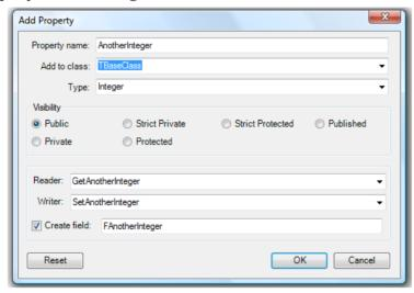
Adding a property works in a proper Delphi way (much more than using UML-based modeling). The tool tends to map to setter and getter methods though you can go for a direct field mapping if you prefer, by adding a prop-
