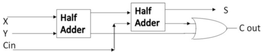
Fig. 4.30 Block Diagram of FA using HA
