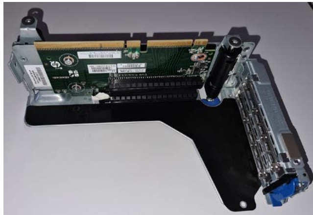
Figure 15.1 – A PCI Express riser for DL380p G8 – you have to insert your PCI Express cards into its slots
