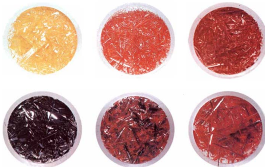
Fig. 9 Band-gap colors in \text{CdS}_{1-x}\text{Se}_x solid solutions. Pure cadmium sulfide (top left) has a band-gap energy of 2.6 eV, with the result that only violet light can be absorbed; the material has the color complementary to violet, namely yellow. In pure cadmium selenide (bottom left) the band-gap energy is 1.6 eV, so that all visible wavelengths are absorbed and the crystals are black. The other four materials are member of the solid solution samples showing a gradient in absorption, with colors from orange through red (2 eV). 3
