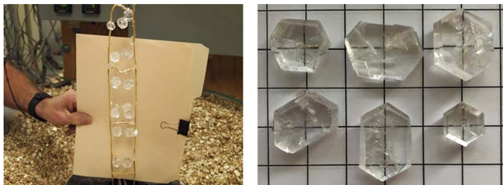
Fig. 11 Hydrothermally grown \text{RbBe}_2(\text{BO}_3)\text{F}_2 (RBBF) crystals. Left: multiple crystals grown on a gold ladder from a single hydrothermal autoclave. Right: As-grown RBBF crystals (1 cm divisions).
