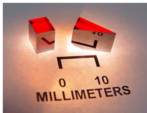
Fig. 8 Photograph of oriented, polished CSP single crystal samples grown by horizontal gradient freeze technique.
