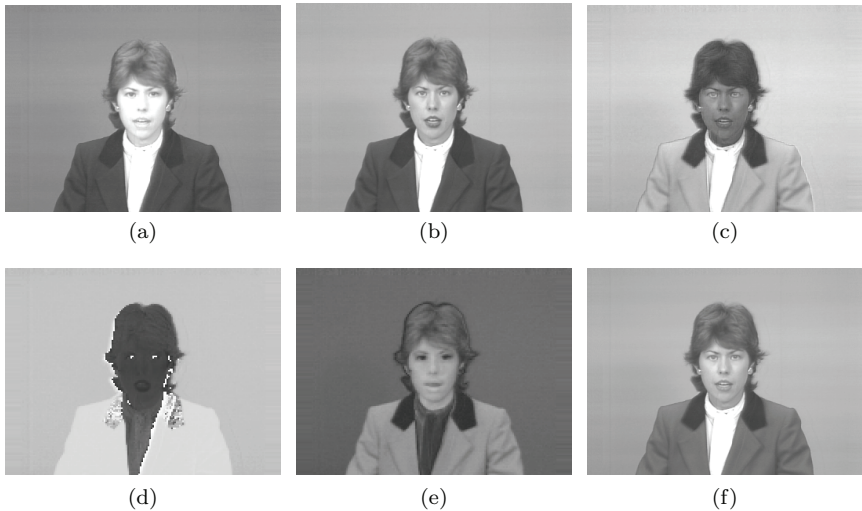
Figure 6.5. R , G , B and H , S , I components of a color image.
