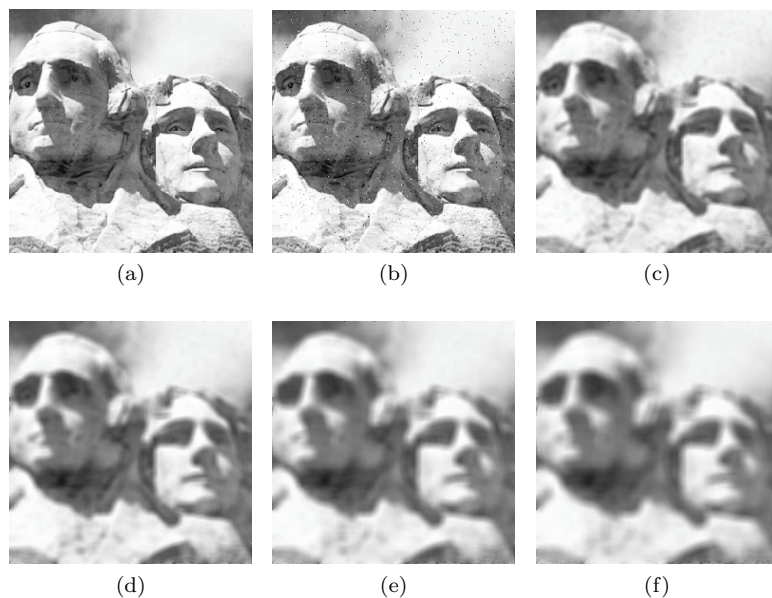
Figure 3.16. Blurring effect of spatial smoothing filter.
